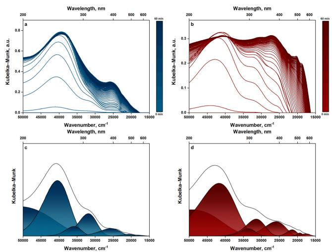
Fig. 6 Operando UV-vis spectra measured during the first hour of TOS for propene oligomerization on (left) ZSM-5 and (right) zeolite beta. Subfigures a and b denote the raw spectra (taken every minute) while subfigures c and d denote the deconvolution of the spectrum measured at the third minute of TOS [523 K; 50 kPa propene pressure; 2 g<sub>C<sub>2</sub>H<sub>6</sub></sub> g<sub>cat</sub><sup>-1</sup> h<sup>-1</sup> WHSV].
