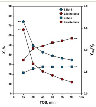
Fig. 1 Propene conversion (X) and relative yield of oligomerization and  $\beta\text{-scission}$  products (Yolig/Y $_\beta$ ) over ZSM-5 and zeolite beta [523 K; 50 kPa propene pressure; 2  $g_{C_3H_6}$   $g_{cat}^{-1}$   $h^{-1}$  WHSV]. Solid lines are guides for the eye.
