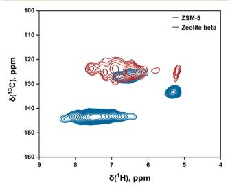
Fig. 5 2D CP-based solid-state <sup>1</sup>H-<sup>13</sup>C NMR spectra of post-reacted ZSM-5 and zeolite beta [523 K; 100 kPa propene pressure; 10-15 min TOS].
