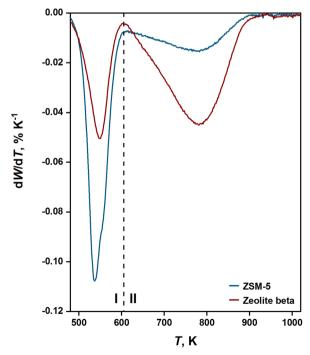
Fig. 2 Derivative of weight loss (W) with respect to temperature measured during TGA for post-reacted ZSM-5 and zeolite beta [523 K; 50 kPa propene pressure; 2  $g_{C_3H_6}$   $g_{cat}^{-1}$   $h^{-1}$  WHSV; 90 min TOS].
