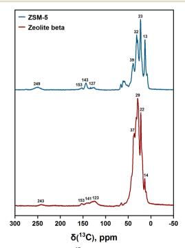
Fig. 4 CP-based solid-state <sup>13</sup>C NMR spectra of post-reacted ZSM-5 and zeolite beta [523 K; 100 kPa propene pressure; 10-15 min TOS].
