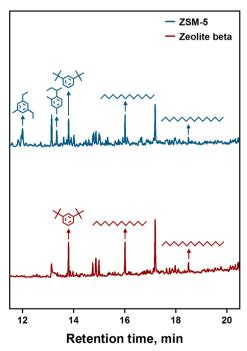
Fig. 3 GC/MS chromatograms of soluble coke extracted from postreacted ZSM-5 and zeolite beta [523 K; 50 kPa propene pressure; 2  $g_{C_xH_6}$   $g_{cat}^{-1}$   $h^{-1}$  WHSV; 90 min TOS].
