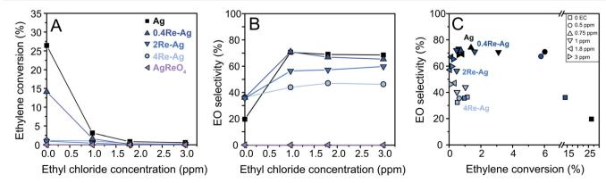
Fig. 5 Ethylene conversion (A) and EO selectivity (B) as a function of the ethyl chloride concentration, at 215 °C and in a total gas flow of 66 mL min<sup>-1</sup>. (C) EO selectivity as a function of ethylene conversion at different EC concentrations, assigned with different symbols.
