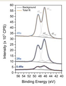
Fig. 1 X-ray photoelectron spectra of the Re 4f region of re on  $\alpha$ -alumina after calcination at 500 °C. Sample names refer to the final Re loading after Ag deposition in at% (Re/(Re + Ag)). Light grey fits correspond to Re<sup>7+</sup> and dark grey fits correspond to Re<sup>6+</sup>
