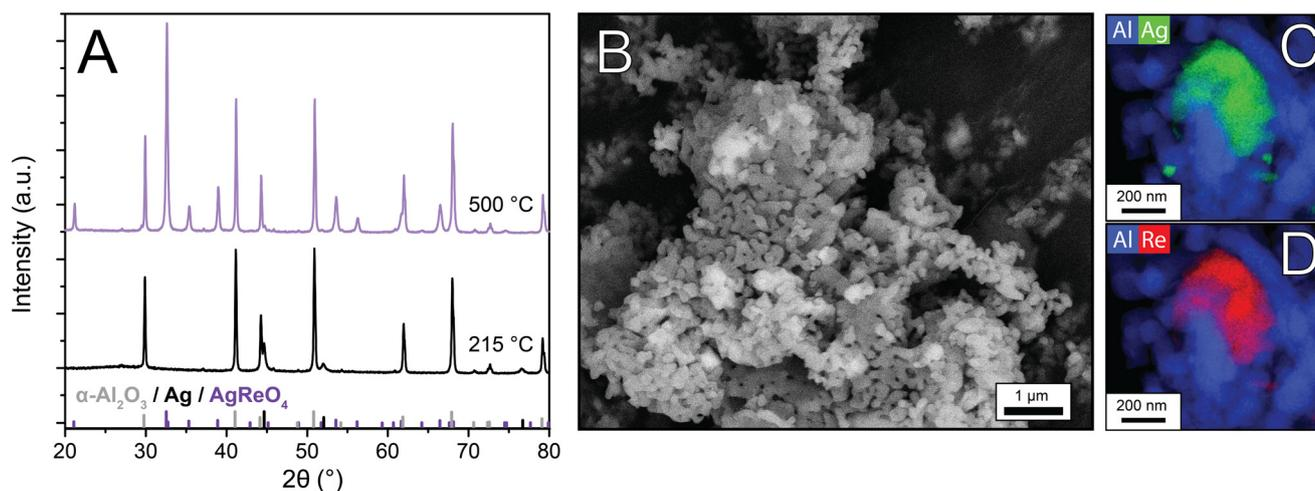
**Fig. 4** X-ray diffractograms of the  $\text{AgReO}_4$  samples calcined at 215 and 500 °C, with theoretical stick diffraction patterns of  $\alpha$ - $\text{Al}_2\text{O}_3$ , Ag and  $\text{AgReO}_4$  below (A), SEM image of  $\text{AgReO}_4/\alpha$ - $\text{Al}_2\text{O}_3$  calcined at 500 °C (B) and STEM-EDX maps of a zoomed in  $\text{AgReO}_4/\alpha$ - $\text{Al}_2\text{O}_3$  particle (C and D).
