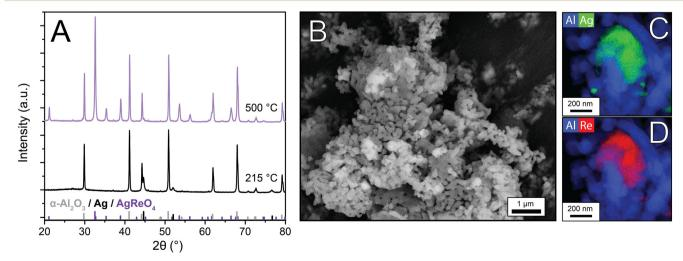
Fig. 4 X-ray diffractograms of the AqReO<sub>4</sub> samples calcined at 215 and 500 °C, with theoretical stick diffraction patterns of  $\alpha$ -Al<sub>2</sub>O<sub>3</sub>, Aq and AgReO<sub>4</sub> below (A), SEM image of AgReO<sub>4</sub>/ $\alpha$ -Al<sub>2</sub>O<sub>3</sub> calcined at 500 °C (B) and STEM-EDX maps of a zoomed in AgReO<sub>4</sub>/ $\alpha$ -Al<sub>2</sub>O<sub>3</sub> particle (C and D).
