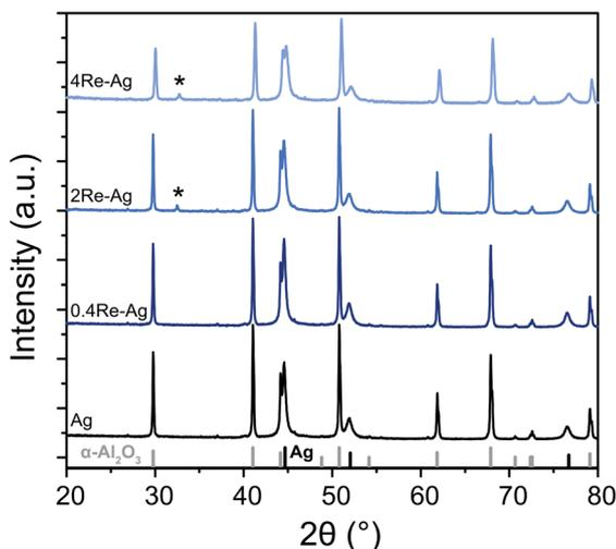
**Fig. 3** X-ray diffractograms of the Ag and Re-promoted Ag catalysts. Theoretical stick diffraction patterns of  $\alpha$ - $\text{Al}_2\text{O}_3$  (grey) and Ag (black) are depicted below the diffractograms as reference. The asterisk (\*) indicates  $\text{AgReO}_4$ .
