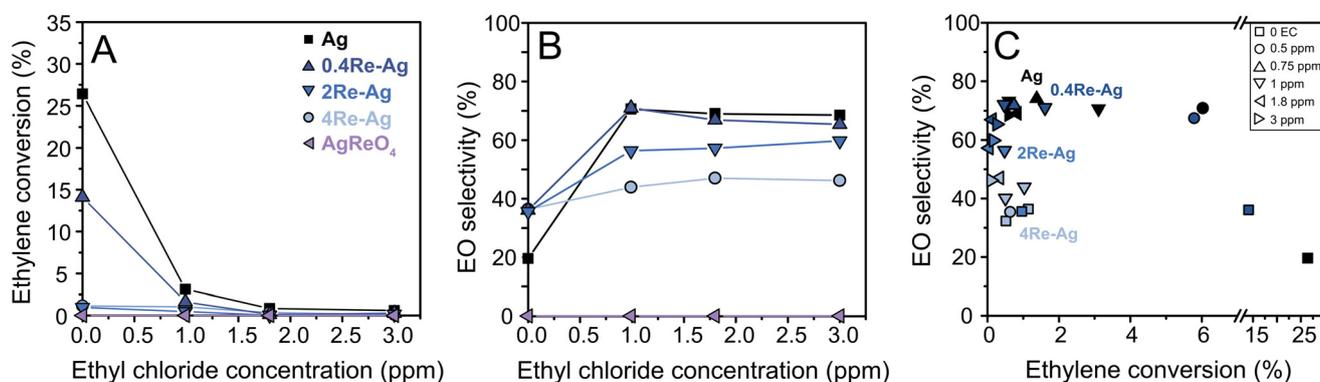
**Fig. 5** Ethylene conversion (A) and EO selectivity (B) as a function of the ethyl chloride concentration, at 215 °C and in a total gas flow of 66 mL min<sup>-1</sup>. (C) EO selectivity as a function of ethylene conversion at different EC concentrations, assigned with different symbols.
