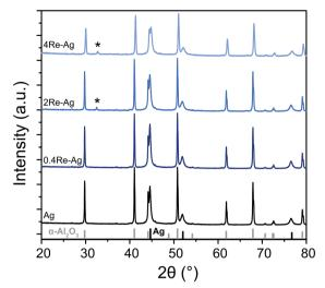
Fig. 3 X-ray diffractograms of the Ag and Re-promoted Ag catalysts. Theoretical stick diffraction patterns of  $\alpha$ -Al<sub>2</sub>O<sub>3</sub> (grey) and Ag (black) are depicted below the diffractograms as reference. The asterisk (\*) indicates AgReO<sub>4</sub>.
