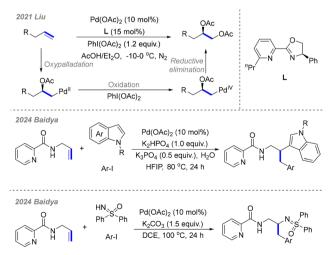
Scheme 90 Palladium-catalyzed difunctionalization of olefins via metal coordination
