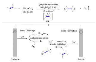
Scheme 87 Electrocatalytic dihalogenation of olefins.
