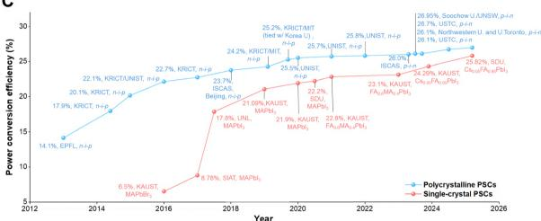
Fig. 7 (A) and (B) Typical architectures of n-i-p and p-i-n PSCs. (C) Timeline of single-junction PSC efficiency for polycrystalline (certified) and SC (non-certified) perovskites. Certified data were extracted from the NREL best research-cell efficiency chart (ref. 221), while the efficiency data of SC perovskite solar cells is obtained from ref. 52, 67, 185, 187, 188, 192, 193, 196, 206 and 208.
