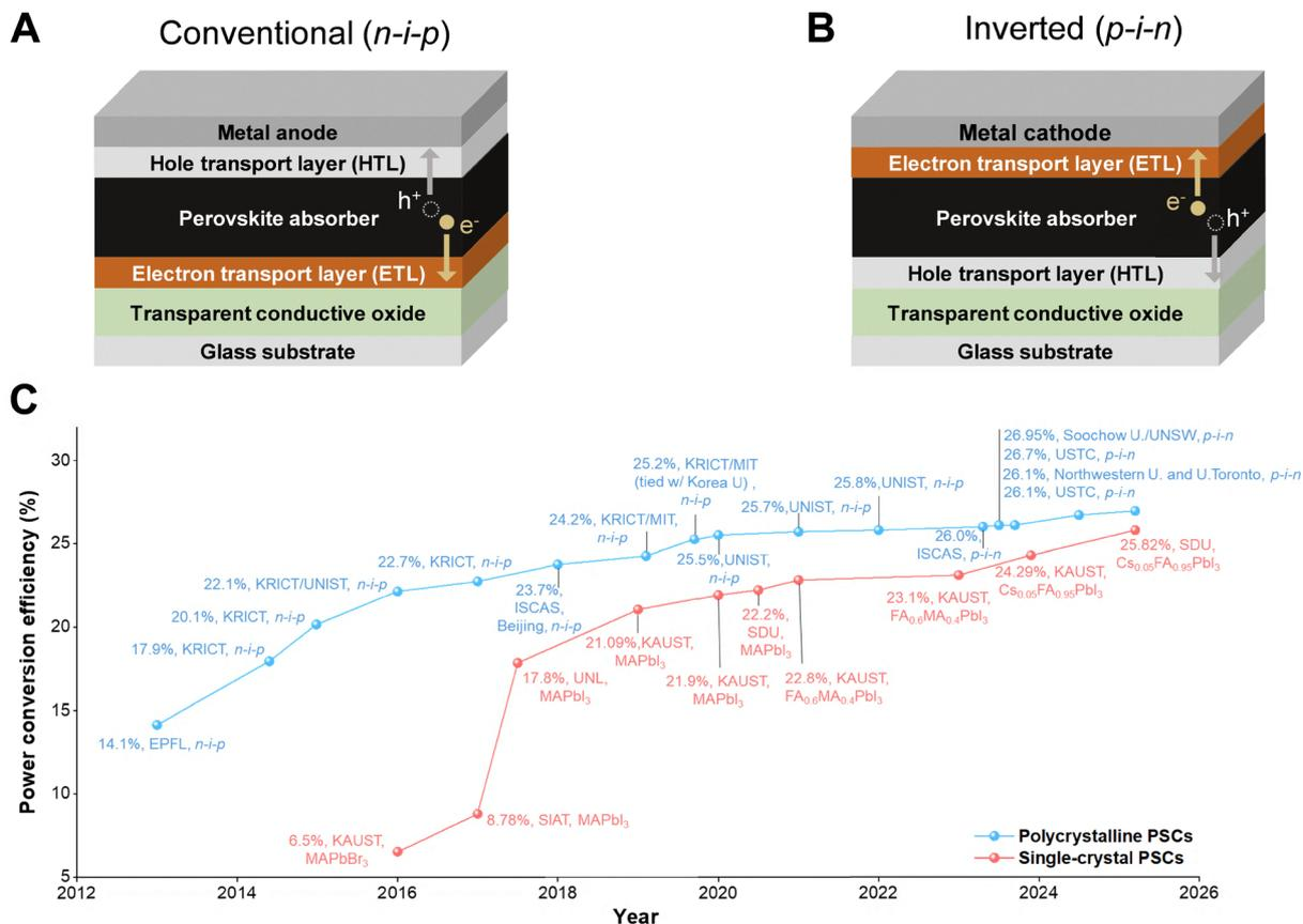
Fig. 7 (A) and (B) Typical architectures of *n-i-p* and *p-i-n* PSCs. (C) Timeline of single-junction PSC efficiency for polycrystalline (certified) and SC (non-certified) perovskites. Certified data were extracted from the NREL best research-cell efficiency chart (ref. 221), while the efficiency data of SC perovskite solar cells is obtained from ref. 52, 67, 185, 187, 188, 192, 193, 196, 206 and 208.
