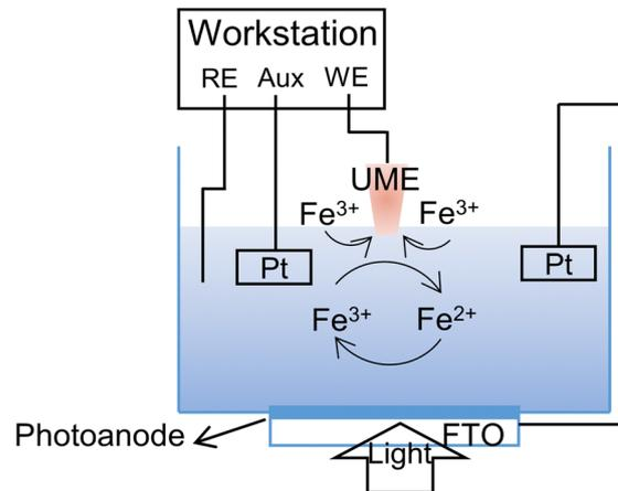
Fig. 11 Basic principles for investigating the interfacial reaction kinetics in photoelectrochemical water splitting under the feedback mode of SPECM.
