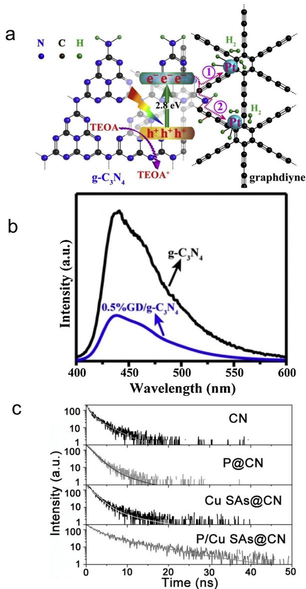
Fig. 3 (a) Schematic diagram for photocatalytic  $\text{H}_2$  evolution on graphdiyne/ $\text{g-C}_3\text{N}_4$  hybrid nanocomposite. (b) Steady-state PL spectra of the samples. Reproduced with permission.<sup>99</sup> Copyright 2019, Elsevier B.V. (c) TRPL analysis and fitting results ( $\lambda_{\text{ex}} = 320 \text{ nm}$ ). Reproduced with permission.<sup>101</sup> Copyright 2022, Wiley-VCH.
