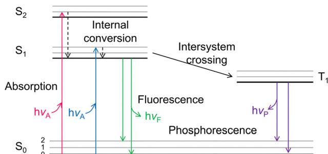
**Fig. 2** Jablonski energy band diagram. S<sub>0</sub>: ground state orbital, S<sub>1</sub>: the first excited singlet state, S<sub>2</sub>: the second excited singlet state,  $h\nu_A$ : absorbed photon energy,  $h\nu_F$ : energy released in the form of fluorescence.
