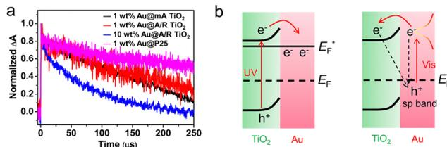
Fig. 9 (a) Normalized decay curves of TRIR absorption at  $1200\text{ cm}^{-1}$  for the photoelectrons in different  $\text{Au}/\text{TiO}_2$  photocatalysts upon the excitation wavelength of 532 nm. Reproduced with permission.<sup>45</sup> Copyright 2019, American Chemical Society. (b) Schematic energy level diagram illustrating electron transfer and the recombination process under UV and Vis irradiation.
