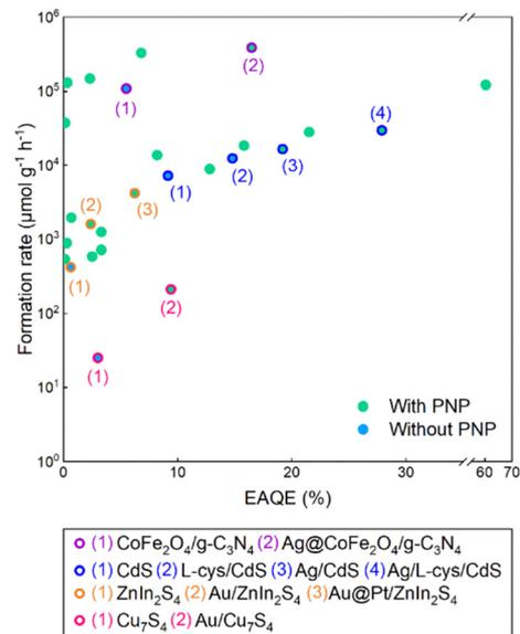
Fig. 27 Formation rate of H<sub>2</sub> versus the external apparent quantum efficiency (selected at the wavelength corresponding to the highest efficiency) for water reduction for the different structures with and without plasmonic nanoparticles (PNPs). Each outer circle color corresponds to one reference showing the photocatalytic performance evolution through additional units composing the photodevice.
