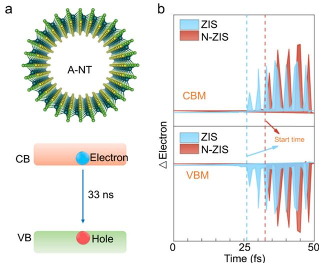
Fig. 22 (a) Predicted atomic structure and recombination time for an electron-hole pair in MoSSe nanotube photocatalyst. Reproduced with permission.<sup>257</sup> Copyright 2019, Royal Society Chemistry. (b) Electron occupation number of VBM and CBM under external field (to simulate photo-illumination) obtained by rt-TDDFT in ZIS and N-ZIS samples. Reproduced with permission.<sup>258</sup> Copyright 2024, Elsevier B.V.
