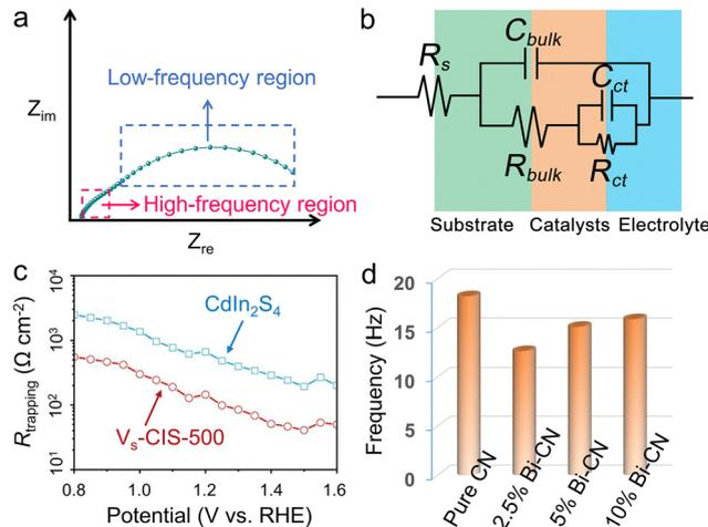
Fig. 10 Schematic diagram for the (a) typical Nyquist plot and (b) equivalent circuit. (c) Fitted  $R_{trapping}$  under different applied potentials that are extracted from the EIS results. Reproduced with permission.<sup>143</sup> Copyright 2020, Springer Nature. (d) Bode-phase plots of the EIS spectra for pristine g-C<sub>3</sub>N<sub>4</sub> and Bi-doped g-C<sub>3</sub>N<sub>4</sub> hybrids. Reproduced with permission.<sup>148</sup> Copyright 2020, Elsevier B.V.
