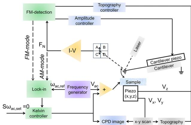
Fig. 17 Signal detection principle for KPFM technique.
