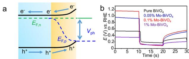
Fig. 13 (a) Schematic diagram for the generation of  $V_{ph}$  in typical n-type semiconductors.  $E_{F,n}$ , quasi-Fermi level of electrons.  $E_{F,p}$ , quasi-Fermi level of holes. (b)  $V_{ph}$  of series BiVO<sub>4</sub> samples after testing 30 seconds. Reproduced with permission.<sup>183</sup> Copyright 2019, Springer Nature.
