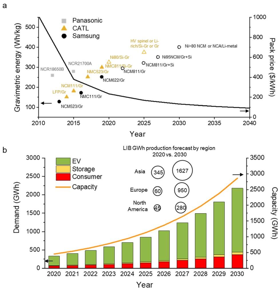
**Fig. 1** Gravimetric energy density, cost, demand and capacity of Li-ion and Li metal chemistry in 2010–2040. (a) Gravimetric performance of different batteries for automotive applications. The predicted LIB pack-cost estimates and aggregation of individual expectations throughout 2040. Reproduced with permission ref. 8. (b) Global lithium battery demand and capacity forecast by sector in 2020–2030. Reproduced with permission ref. 16 and 17.
