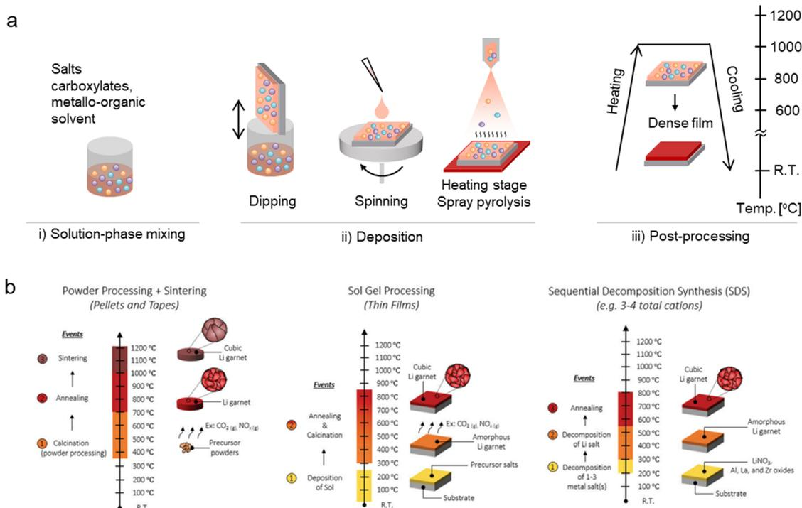
Fig. 6 (a) Typical steps in wet-chemical synthesis. (b) Processing temperature, events, and ionic conductivity of Li garnets synthesized *via* powder, sol-gel, and sequential decomposition synthesis (SDS). Reproduced with permission ref. 318.
