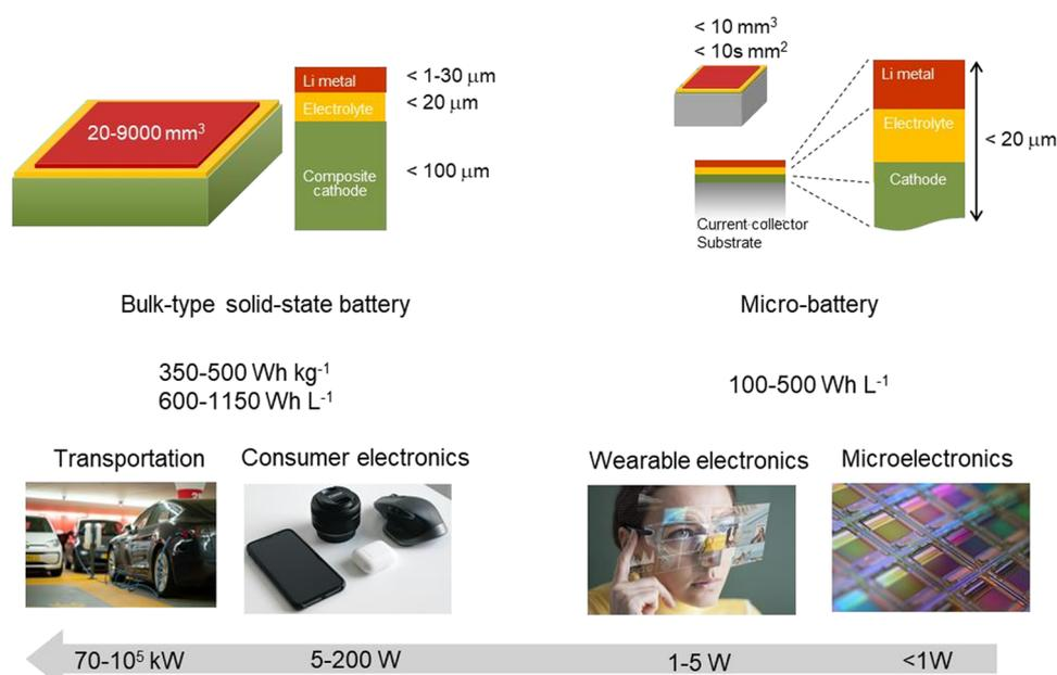
Fig. 3 Major requirement differences between bulk and micro solid-state batteries, in terms of thickness [μm], footprint area [mm<sup>3</sup>], energy density [Wh kg<sup>-1</sup> and Wh L<sup>-1</sup>] and power consumption [W] in major applications.
