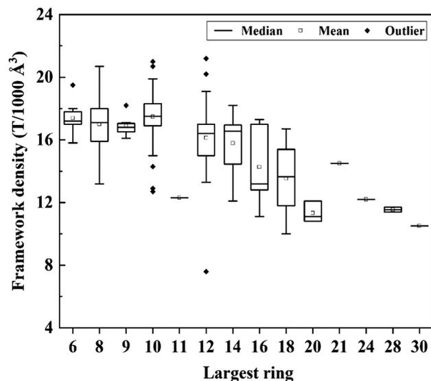
Fig. 2 Relation between zeolite framework density and largest ring, using data from IZA database with one new additional zeolite (ZMQ-1<sup>86</sup>) and including 260 structures.
