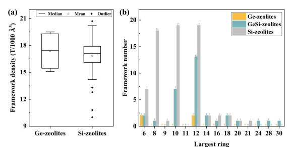
Fig. 3 (a) Framework density of SiO<sub>2</sub> and GeO<sub>2</sub> zeolites; (b) largest ring of Si-, Ge-, and SiGe-zeolites
