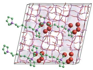
Fig. 5 Location of 1,6-bis(N-methylpyrrolidinium)hexane (H atoms omitted for clarity) in the micropore (shaded) of siliceous SSZ-74, with the short distance between siloxy or silanol oxygens (large red balls) and quaternary nitrogens (purple balls) of the OSDA highlighted (dotted lines) for the central molecule. Geometry taken from ref. 130.
