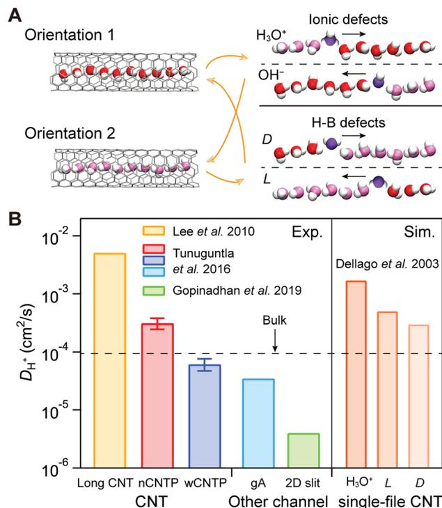
Fig. 8 Enhanced proton transport in CNTs. (A) Schematic of the charge transport mechanisms. (B) Proton diffusion coefficients across different environments, including bulk water,<sup>603,604</sup> two-dimensional (2D) graphite slits,<sup>65</sup> gramicidin A (gA) channels,<sup>180,604</sup> long CNTs<sup>121</sup> and CNT porins.<sup>180</sup> Simulations from ref. 383 provide proton transport data for a CNT (6,6) in an ideal case and in presence of a *D* or *L* defect.
