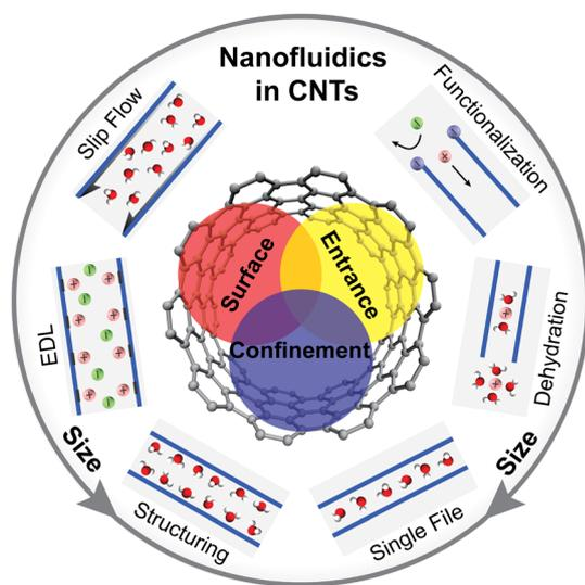
**Fig. 1** Key physical phenomena and mechanisms that govern nanofluidic transport in CNT pores. Key mechanisms include surface interactions that determine fluid slip and electrostatic coupling, entrance effects that include dehydration and interaction with charged functional groups, and confinement effects that encompass fluid ordering and single-file transport.
