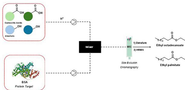
Fig. 8 Microfluidic system SEC-HRMS to identify BSA inhibitors.
