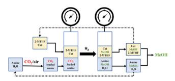
Fig. 12 Schematic representation of a biphasic system for CO<sub>2</sub> capture from air using an amine aqueous solution and hydrogenation of the captured CO<sub>2</sub> to MeOH through combination of the absorbing agueous solution with an organic phase containing the homogeneous hydrogenation catalyst. Reproduced with permission from ref. 94a.
