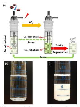
Fig. 9 (a) Illustration of the CO<sub>2</sub> capture and regeneration process with a biphasic system, (b) the homogenous amino acid salt solution before, and (c) after CO<sub>2</sub> loading, showing the formation of two phases. Reproduced from ref. 54 with copyright permission.
