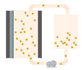
Fig. 8 Schematic illustration of liquid/solid membrane-free RFB.
