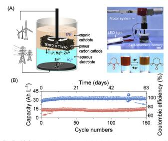
Fig. 3 (A) Schematic illustration and digital photographs of stirred selfstratified battery. (B) Cycling performance of a 20 W h L<sup>-1</sup> stirred selfstratified battery. Reproduced with permission from ref. 29. Copyright 2020, Elsevier.
