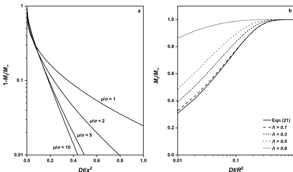
Fig. 9 (a) Effect of the size distribution on the uptake solution. Reproduced from ref. 66 with permission. Copyright 1971 Elsevier. (b) Effect of the amount of sorbate ultimately sorbed on the uptake solution. Reproduced from ref. 68 with permission. Copyright 2012 John Wiley and Sons.
