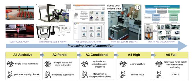
Fig. 5 The five levels of autonomy differ in the automated steps and the level of human intervention. Select examples are depicted spanning the range of automation spanned by the levels of autonomy. Figures in the top panel are reproduced under a Creative Commons license. 445,447–450
