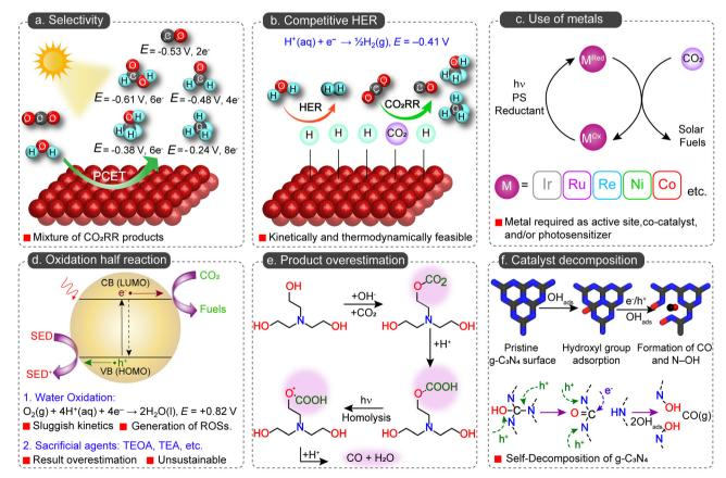
Fig. 3 Challenges of photocatalytic CO<sub>2</sub> reduction. (a) Selectivity of the product formed, (b) competitive hydrogen evolution reaction, (c) use of metals, (d) challenging oxidation half-reaction, (e) overestimation of the product yield, and (f) decomposition of the catalyst under the reaction conditions.
