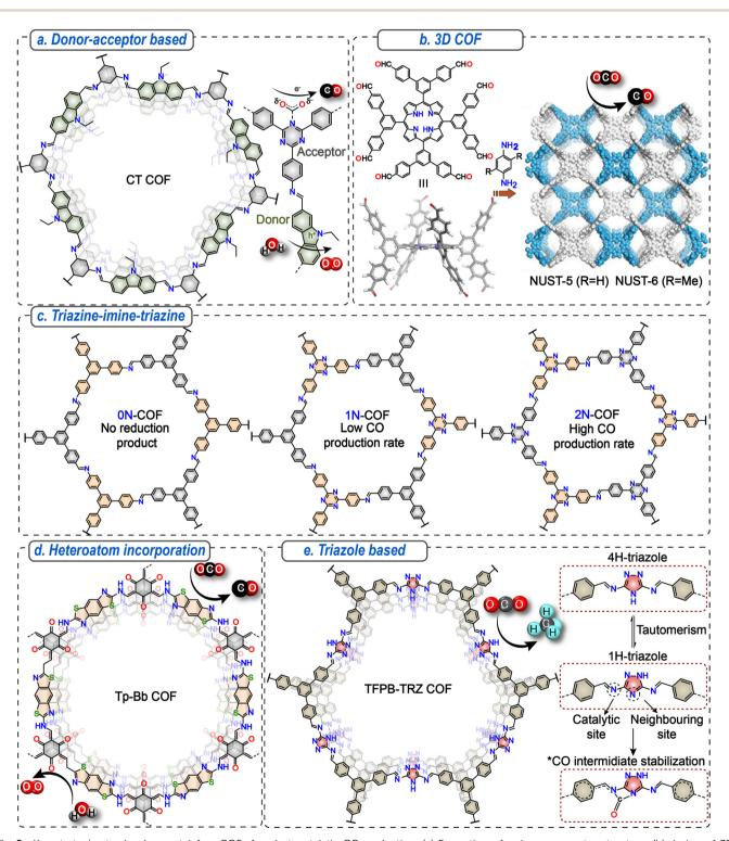
Fig. 8 Key strategies to develop metal-free COFs for photocatalytic CO<sub>2</sub> reduction. (a) Formation of a donor-acceptor structure, (b) design of 3D structure, adapted with permission from ref. 121, Copyright © 2022, American Chemical Society. (c) Fabricating COF membranes with the triazineimine-triazine linkage, (d) incorporation of heteroatoms, and (e) triazole-based system.
