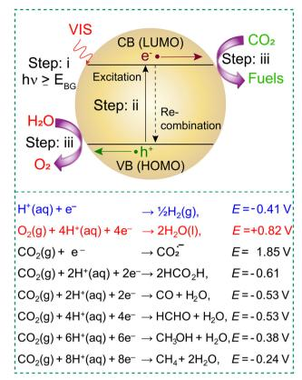
Fig. 2 Mechanism of photocatalytic CO<sub>2</sub> reduction on a semiconductor photocatalyst.
