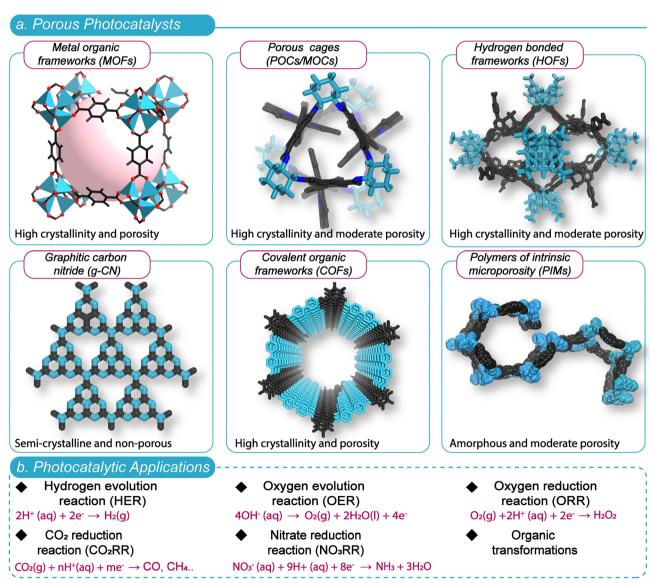
Fig. 1 (a) Schematic representation of the various categories of porous heterogeneous photocatalysts constructed using precise building units. (b) Illustration of the different photocatalytic applications of porous materials.
