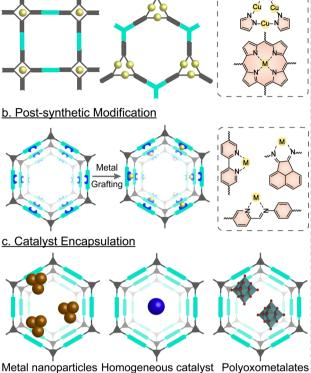
Fig. 5 Various strategies for fabricating metalated covalent organic frameworks for photocatalytic CO2 reduction.
