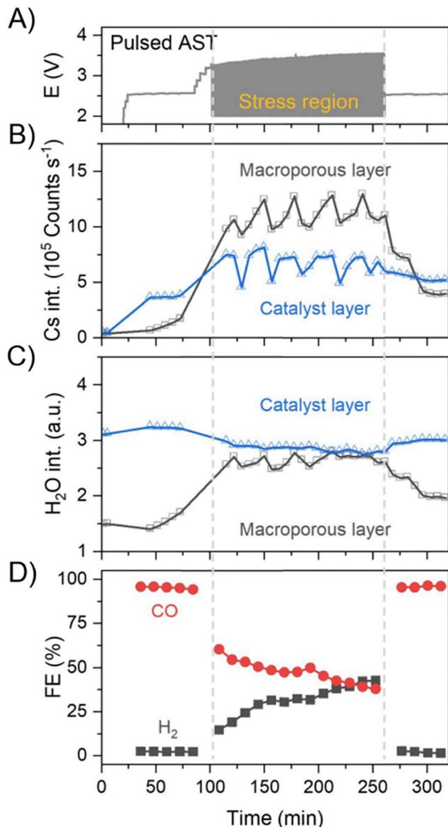
Fig. 23 (A) Cell potential during an AST in an AEM MEA with the 0.1 M  $\text{CsHCO}_3$  electrolyte. (B) Cs signal intensity (could be used towards quantification) measured by *in situ* x-ray fluorescence. (C) Water signal intensity measured by wide angle x-ray scattering. (D)  $\text{CO}_2\text{R}$  FE for CO and  $\text{H}_2$  during the AST.<sup>277</sup> Reprinted (adapted) with permission under Creative Commons License.
