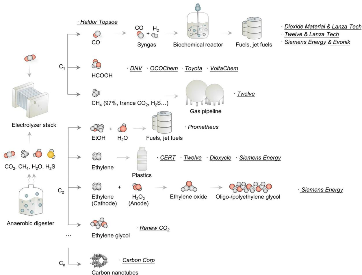
Fig. 25 Summary of pathways and target products of companies based on ECR technologies.<sup>290</sup> Reprinted (adapted) with permission. Copyright 2024 American Chemical Society.
