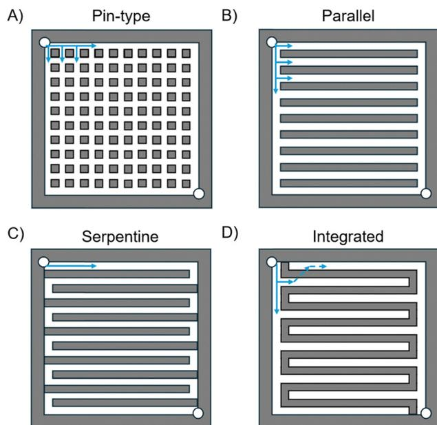
Fig. 5 Illustrations of flow field patterns: (A) pin-type, (B) parallel, (C) serpentine, and (D) integrated.
