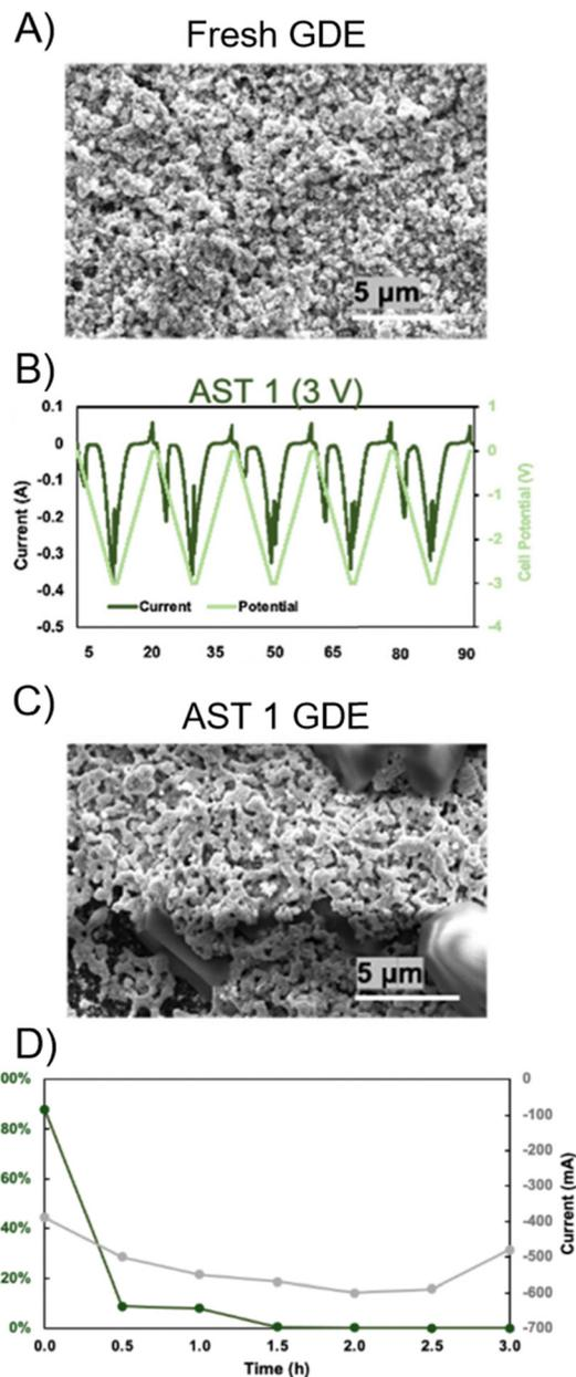
Fig. 24 (A) SEM image of an as-prepared Ag-GDE. (B) Current and cell potential of an “AST 1” protocol in a GDE flow cell. (C) SEM of GDE after the “AST 1” protocol. (D) CO FE and current as a function of time during the “AST 1” protocol.<sup>278</sup> Reprinted (adapted) with permission. Copyright 2022 American Chemical Society.
