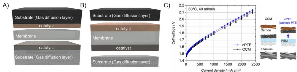
Fig. 26 Schematic illustrations of (A) CCS and (B) CCM for MEAs.<sup>303</sup> Reprinted (adapted) with permission under Creative Commons License. (C) Comparison of CCM and half CCM/half CCS water electrolysis with the same catalysts in a PEMWE device under the same operating conditions.<sup>299</sup> Reprinted (adapted) with permission under Creative Commons License.
