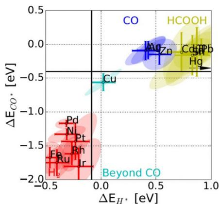
**Fig. 2** Binding energies of \*CO and \*H adsorbed intermediates as descriptors for trends in primary product formation over various ECR catalysts.<sup>31</sup> Reprinted (adapted) with permission from the Wiley materials.
