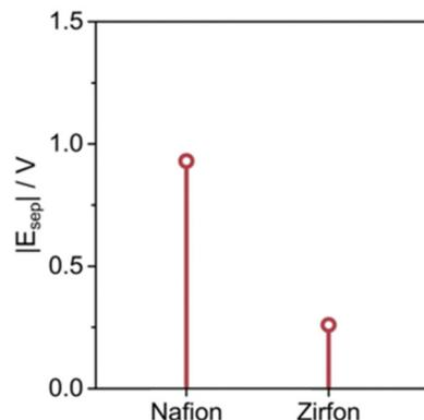
Fig. 13 Comparison of the voltage drop between two identical  $\text{CO}_2\text{R}$  setups featuring either a Nafion membrane or a porous Zirfon separator in 3 M KCl/0.05 M  $\text{H}_2\text{SO}_4$  electrolyte.<sup>117</sup> Reprinted (adapted) with permission under Creative Commons License.
