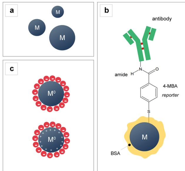
Fig. 2 Commonly encountered depictions of metallic (M) colloidal nanoparticles. (a) Representation of colloidal nanoparticles as solid bodies of a given shape, e.g., a sphere. (b) Complex representation of a SERS nanotag (*i.e.*, functionalized nanoparticle for indirect SERS) in which the conjugation chemistry is highlighted. (c) Representation of colloidal nanoparticles as solid bodies bearing a surface charge.
