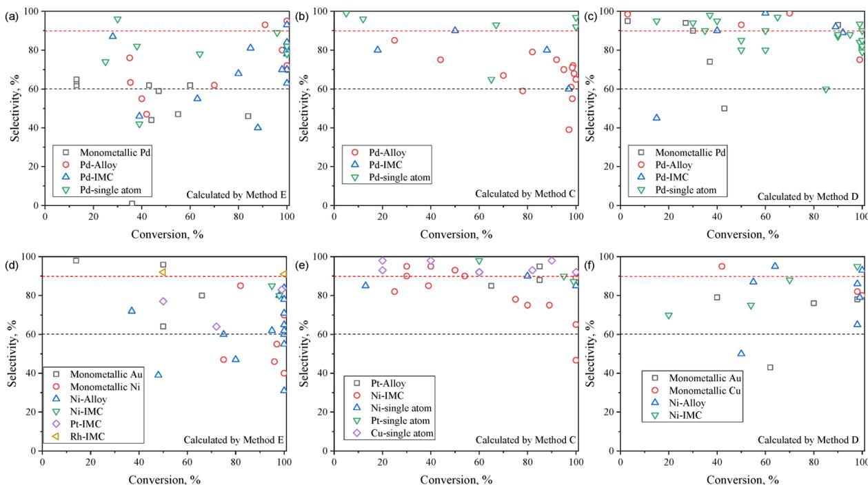
Fig. 5 Ethylene selectivity versus acetylene conversion over (a)–(c) Pd-based and (d)–(f) non-Pd-based catalysts. Methods C, D, and E in the figures correspond to the ethylene calculation methods specified in Table 2. The data are summarized from Tables 3–10.
