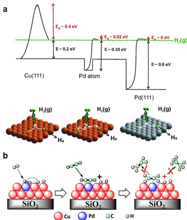
Fig. 13 (a) Potential energy diagram of  $H_2$  dissociation over the Pd<sub>1</sub>/Cu(111) surface, where the orange and gray atoms are Cu and Pd, respectively. Reprinted with permission from ref. 222. Copyright 2012 The American Association for the Advancement of Science. (b) Proposed reaction pathway for semihydrogenation of acetylene over silica-supported Cu-alloyed Pd SA. Reprinted with permission from ref. 116. Copyright 2017 American Chemical Society.
