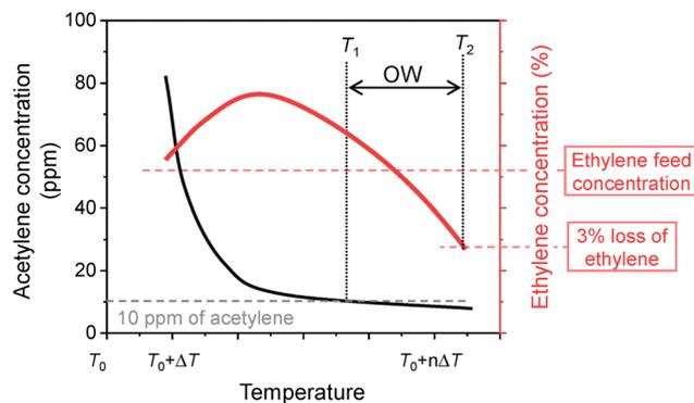
Fig. 3 Acetylene hydrogenation test for catalysts in ethylene-rich streams. Reprinted with permission from ref. 2. Copyright 2008 Taylor & Francis. The difference between  $T_1$  and  $T_2$  is called the operating window (OW). Catalyst with a large OW is more thermally stable at the temperature necessary to remove acetylene from the feed.
