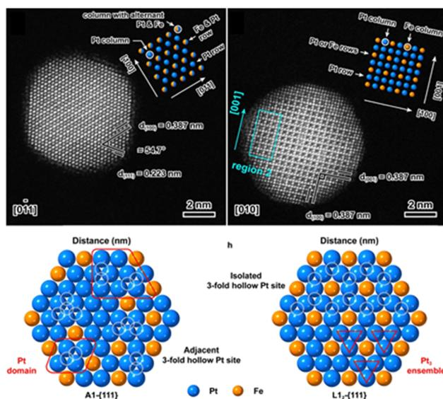
Fig. 16 Geometric arrangements of Pt and Fe atoms in the Pt<sub>3</sub>Fe A1 and L<sub>1</sub><sub>2</sub> NPs. Reprinted with permission from ref. 184. Copyright 2023 Elsevier.
