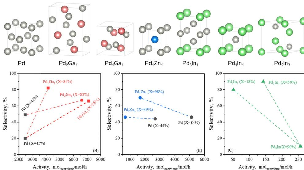
Fig. 9 Catalytic performance of Pd-based IMC catalysts for acetylene hydrogenation. Letters in parentheses indicate the selectivity calculation method as specified in Table 2.
