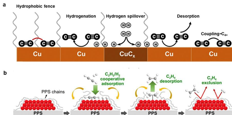
Fig. 21 (a) Schematic illustration of the semihydrogenation of alkyne on Cu<sub>2</sub>O–C<sub>16</sub>. Reprinted with permission from ref. 473. Copyright 2024 American Chemical Society. (b) Reversibility of Pd–PPS interaction and proposed acetylene hydrogenation scheme over Pd/PPS. Reprinted with permission from ref. 474. Copyright 2020 The American Association for the Advancement of Science.
