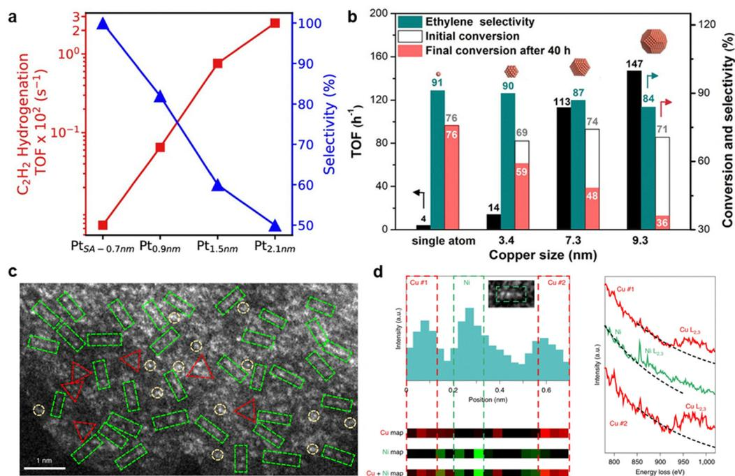
Fig. 17 Size effect of (a) Pt active site and (b) Cu active site on the activity and selectivity for acetylene hydrogenation. Reprinted with permission from refs. 255 and 196. Copyright 2019 American Chemical Society and 2020 American Chemical Society. (c) and (d) Structural characterization of Ni<sub>1</sub>Cu<sub>2</sub>/g-C<sub>3</sub>N<sub>4</sub> catalyst. Reprinted with permission from ref. 193. Copyright 2021 Springer Nature.
