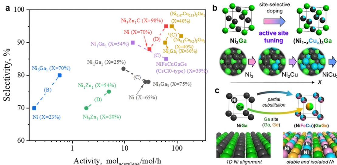
Fig. 15 (a) Catalytic performance of Ni based IMC catalysts for acetylene hydrogenation. (b) Site-selective doping of Cu to the Ni sites of Ni<sub>3</sub>Ga IMC. Reprinted with permission from ref. 179. Copyright 2024 Royal Society of Chemistry. (c) Multi-metallization of intermetallic NiGa to (NiFeCu)(GaGe) HEI. Reprinted with permission from ref. 174. Copyright 2022 Wiley-VCH GmbH. Letters in parentheses indicate the selectivity calculation method as specified in Table 2.
