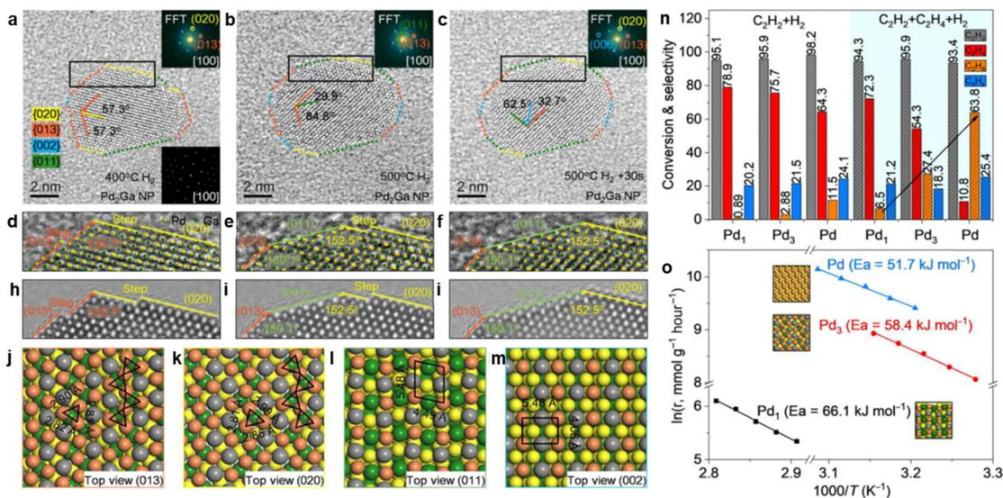
Fig. 10 (a)–(m) Surface atom arrangement and variation during Pd<sub>2</sub>Ga refacetting, and (n) and (o) Hydrogenation properties of different surface Pd geometries. Reprinted with permission from ref. 81 Copyright 2022 The American Association for the Advancement of Science.
