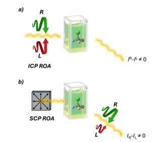
Fig. 10 Schematic representation of the two ROA techniques. (a) ICP ROA measures ( $I^R - I^L$ ), where  $I^R$  and  $I^L$  are the scattered intensities in rightand left-circularly polarized incident light, respectively. (b) SCP ROA measures  $(I_R - I_L)$ , where  $I_R$  and  $I_L$  are the intensities of the right- and left circularly polarized components, respectively, of the scattered light using incident light of fixed polarization.
