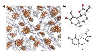
Fig. 15 (a) The crystal structure of a chiral guest, santonin, trapped in a crystalline sponge. (b) ORTEP drawing (50% probability) of the santonin trapped in the pore and the chemical structure of santonin. Reproduced from ref. 72 with permission from Springer Nature BV, copyright 1995.
