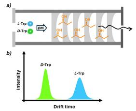
Fig. 14 Separation of D- and L-tryptophan by IM-MS. (a) The presence of (R)-2-butanol as a chiral selector in the gas of the drift tube induces diverse drift times of the opposite enantiomers. (b) The intensity of peaks relative to the two enantiomers can be correlated to the ee of the sample
