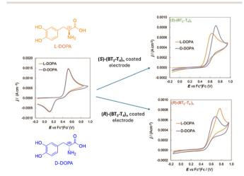
Fig. 16 Cyclic voltammetry of DOPA enantiomers (4 mM H<sub>2</sub>O + 50 mM HCl) recorded with (left) a bare GC electrode, (right, up) a GC electrode coated with (S)-(BT $_2$ -T $_4$ ) $_n$ , and (right, down) a GC electrode coated with (R)- $(BT_2-T_4)_{n_1}$  the enantiomeric pair of bithianaphthene-based oligomers. Reproduced from ref. 79 with permission from The Royal Society of Chemistry, copyright 2010.
