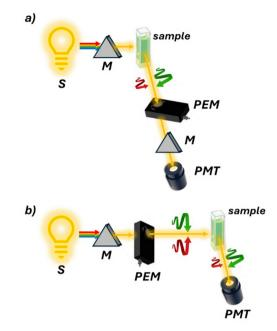
Fig. 8 Schematic representation of (a) a CPL and (b) an FDCD spectropolarimeter. FDCD has the same optical components as CD with the photomultiplier tube (PMT) placed at 90° to collect the fluorescence. CPL instead has the photoelastic modulator (PME) after the sample to detect the differently emitted right and left circular polarizations.
