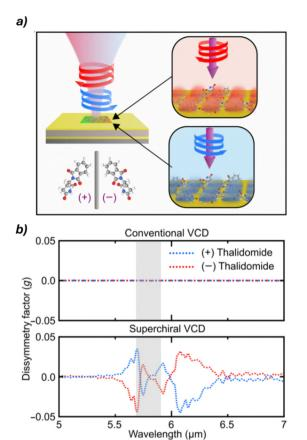
Fig. 11 (a) Schematic representation of the chiral analysis of (+)/(-)-thalidomide using the gold-based plasmonic sensor. (b) Comparison of dissymmetry factors obtained with conventional VCD and superchiral light-enhanced VCD, highlighting the substantial signal enhancement achieved with the nanophotonic approach. Reproduced from ref. 54 with permission from The American Association for the Advancement of Science, copyright 2024.
