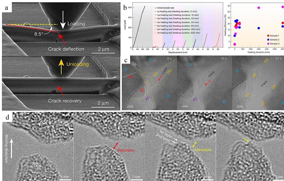
Fig. 11 Study of the self-healing behaviour of ntDC. (a) The SENB test of ntDC.<sup>149</sup> Reproduced with permission from ref. 149, Copyright 2020, Springer Nature. (b) Testing of mechanical properties with different healing times of ntDC. (c) DOs formation process. (d) Atomic-scale healing processes of ntDC.<sup>163</sup> Reproduced with permission from ref. 163, Copyright 2023, Springer Nature.
