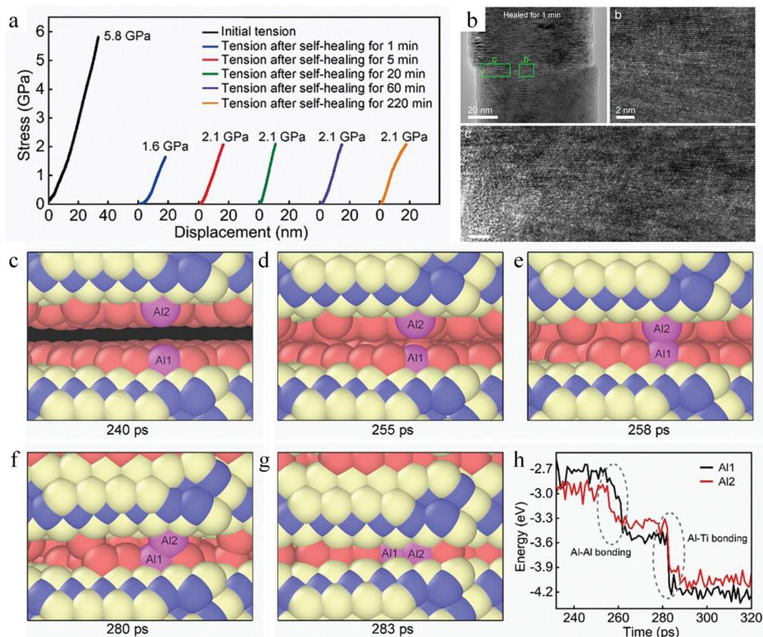
Fig. 17 Study of the self-healing behavior of  $\text{Ti}_3\text{AlC}_2$  MAX phase. (a) Stress–displacement curves obtained from healing experiments. (b) Characterization of fracture surfaces of  $\text{Ti}_3\text{AlC}_2$ . (c)–(h) The self-healing process between two fracture surfaces of the  $\text{Ti}_3\text{AlC}_2$ .<sup>168</sup> Reproduced with permission from ref. 168, Copyright 2024, Wiley-VCH.
