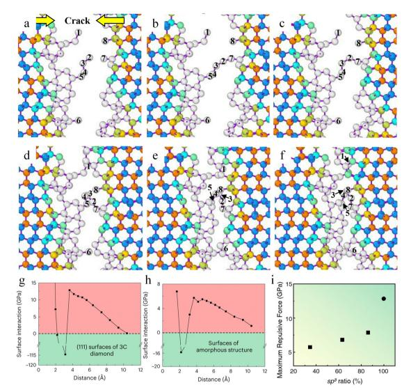
Fig. 12 Simulation of the self-healing process between two fractured ends of ntDC. (a)-(f) Molecular dynamics simulation of the ntDC crack healing process with DOs. (q) Force per area versus distance curve between two (111) surfaces of diamond. (h) Force per area versus distance curve between two amorphous DO structures with an sp3 ratio of 34.7%. (i) The maximum repulsive force per area versus sp3 content. 163 Reproduced with permission from ref. 163, Copyright 2023, Springer Nature.
