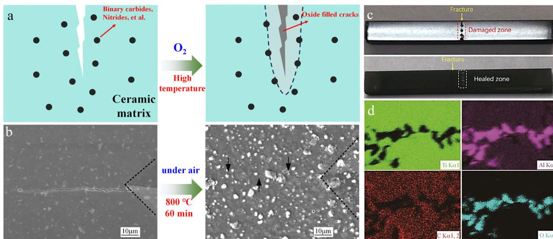
Fig. 3 Self-healing ceramics based on oxidizing mechanism. (a) Schematic of oxidative healing mechanisms. (b) Surface crack morphology of self-healing  $\text{Al}_2\text{O}_3$  ceramic before and after healing.<sup>63</sup> Reproduced with permission from ref. 63, Copyright 2023, Elsevier. (c) and (d) Fracture behavior of  $\text{Ti}_2\text{AlC}$  before and after healing and EDS spectrum of the healed region.<sup>66</sup> Reproduced with permission from ref. 66, Copyright 2022, Springer Nature.
