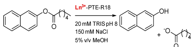
Fig. 29 Hydrolysis of 2-naphthyl hexanoate by Ln-PTE-R18.
