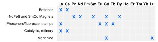
Fig. 25 Overview of the most developed Industrial uses of Ln: rechargeable batteries, permanent magnets, lightings, catalysis and refinery, and medicine. Pm is a radioactive element and does not occur in Nature.
