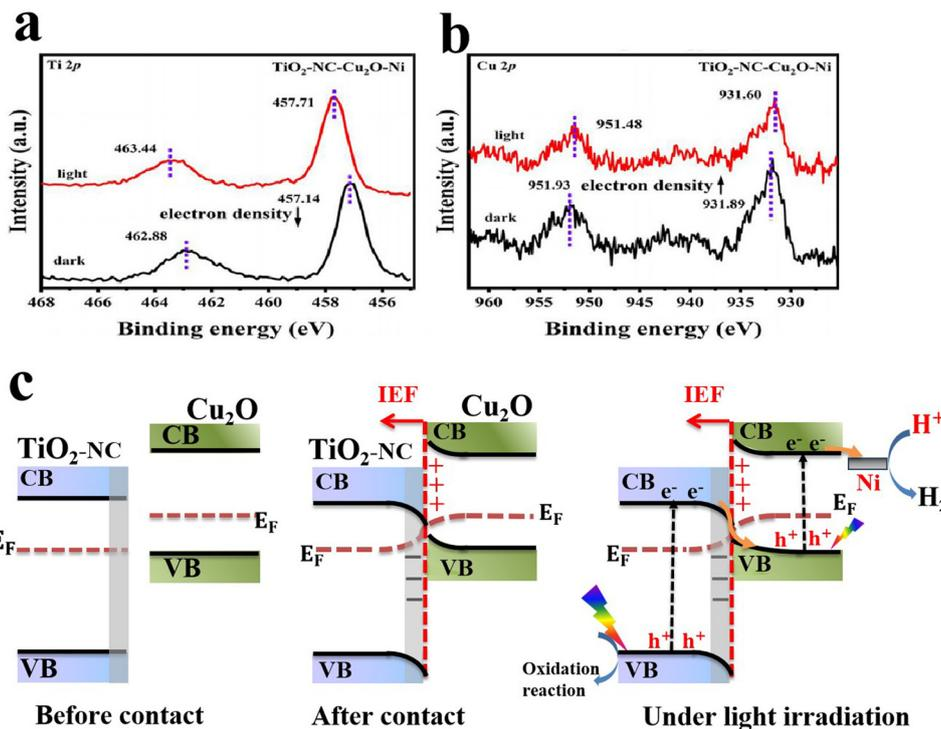
Fig. 16 (a) ISIXPS spectra of (c) Ti 2p and (b) Cu 2p for the TiO<sub>2</sub>-NC-3%Cu<sub>2</sub>O-3%Ni catalyst in the dark as well as under 365 nm light irradiation. Reproduced with permission.<sup>68</sup> Copyright 2024, Elsevier. (c) Schematic representation of interfacial electron transfer and migration over TiO<sub>2</sub>-NC and Cu<sub>2</sub>O before contact (left), after contact (middle), and under light irradiation (right).
