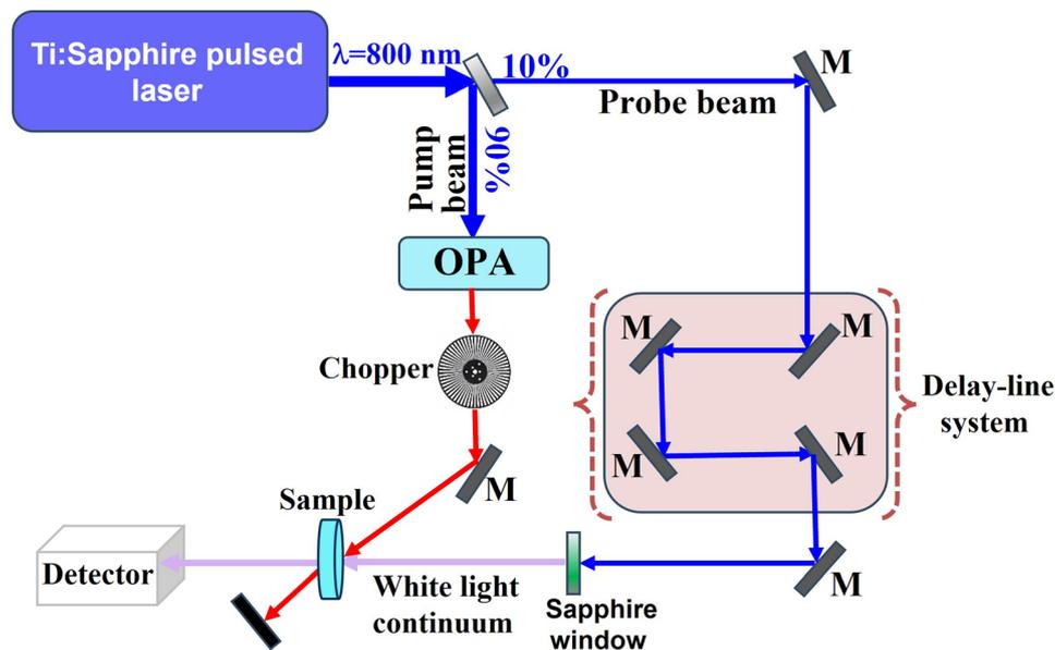
Fig. 14 Schematic layout of the fs-TAS apparatus setup. M: mirror; OPA: optical parametric amplifier.
