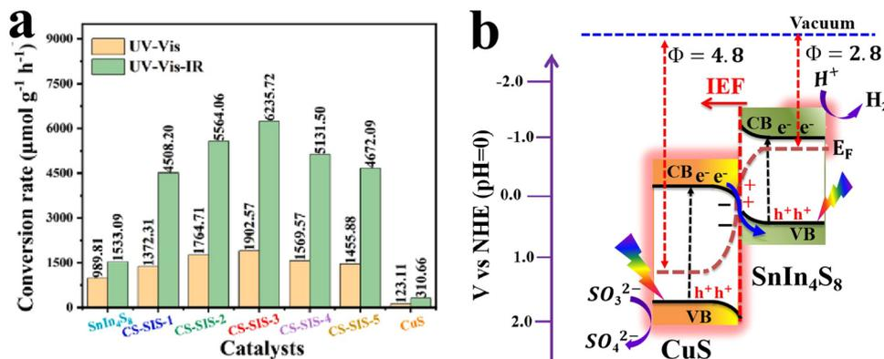
Fig. 27 (a) Average photocatalytic H<sub>2</sub> production over different CuS catalysts under UV-vis and UV-vis-IR illumination. Reproduced with permission.<sup>217</sup> Copyright 2024, Elsevier. (b) Illustration of the charge transfer mechanism over the CuS/SnIn<sub>4</sub>S<sub>8</sub> S-scheme heterojunction. The red glow shows the photothermal effect due to LSPR on CuS.
