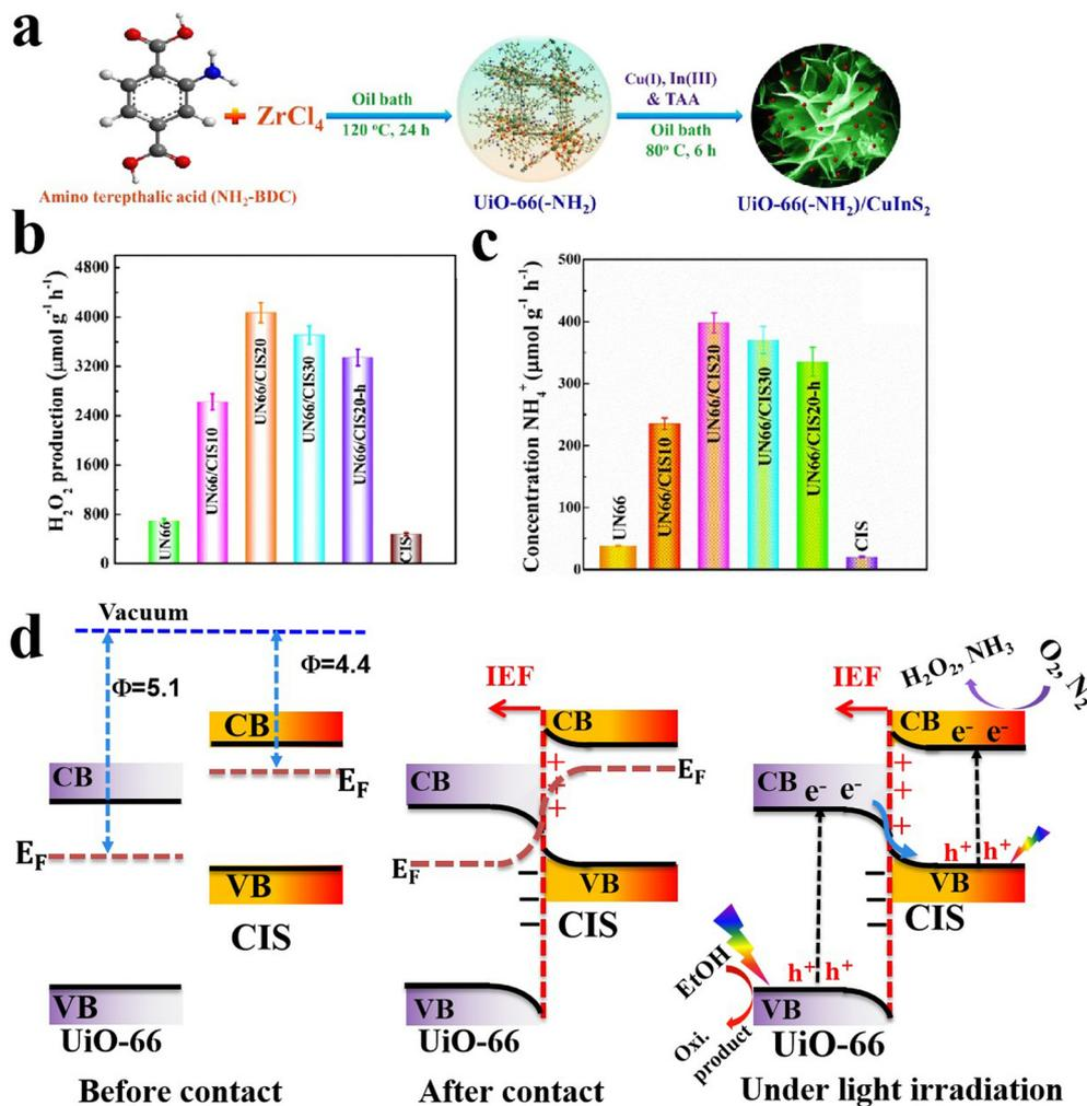
Fig. 29 (a) Fabrication of UiO-66/CIS S-scheme heterojunctions. Photocatalytic performances of the prepared catalysts for (b) H<sub>2</sub>O<sub>2</sub> production and (c) N<sub>2</sub> fixation. Reproduced with permission.<sup>51</sup> Copyright 2023, American Chemical Society. (d) Schematic representation of the band edge potentials of pure CIS and UiO-66 components and plausible S-scheme charge transfer mechanisms in the UiO-66/CIS heterostructures.
