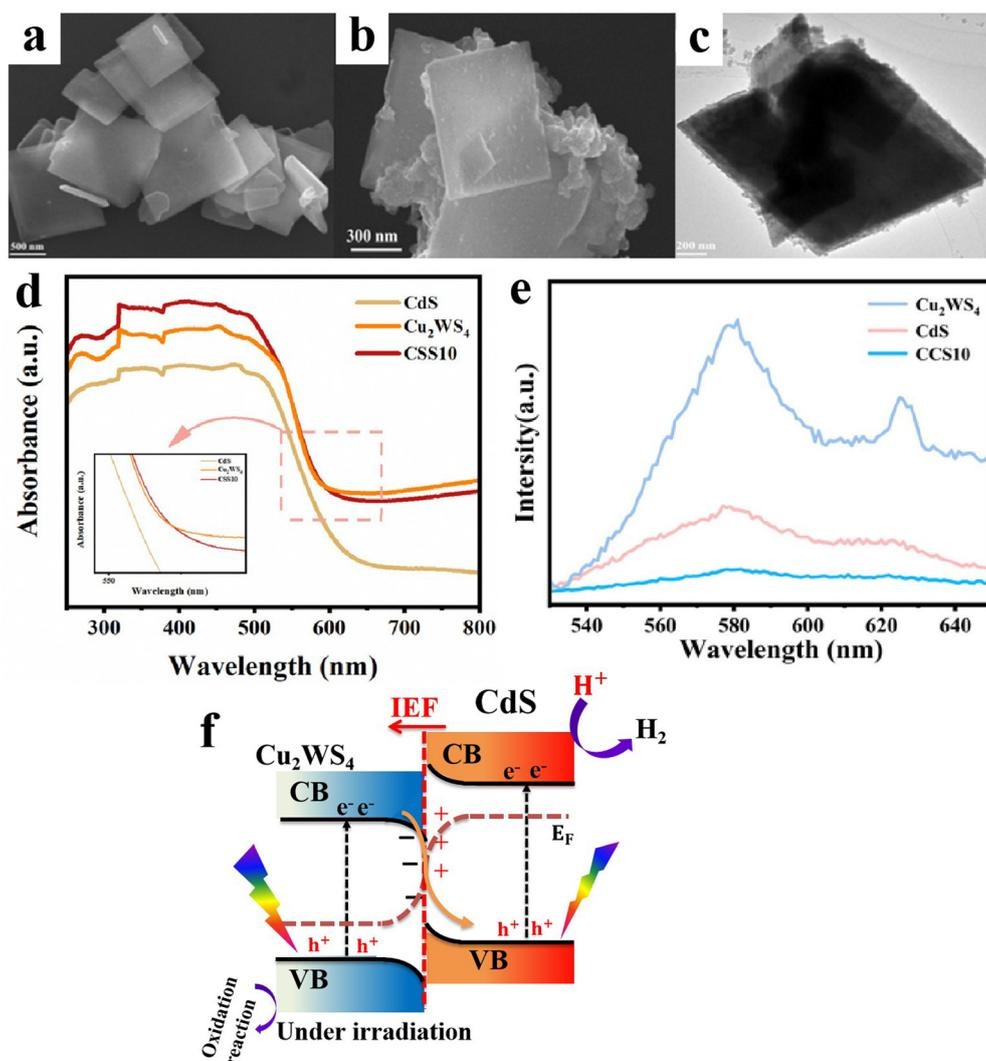
**Fig. 30** SEM images of (a)  $\text{Cu}_2\text{WS}_4$  and (b)  $\text{Cu}_2\text{WS}_4/\text{CdS}$ -10 (CSS10); (c) TEM image of CSS10; DRS (d) and PL curves (e) of the prepared photocatalysts. Reproduced with permission.<sup>230</sup> Copyright 2023, Royal Society of Chemistry. (f) Band structure and proposed charge migration pathway over the  $\text{Cu}_2\text{WS}_4/\text{CdS}$  S-scheme heterojunction.
