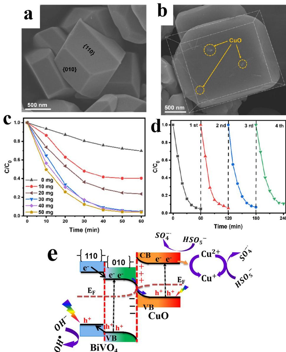
Fig. 22 FESEM images of (a)  $\text{BiVO}_4$  and (b) CuO/ $\text{BiVO}_4$  samples, highlighting the location of CuO NPs. (c) Photocatalytic degradation efficiency of CuO/ $\text{BiVO}_4$  for the NOR solution at different PMS doses and (d) the recyclability of the CuO/ $\text{BiVO}_4$  photocatalyst. Reproduced with permission.<sup>148</sup> Copyright 2024, Elsevier. (e) Proposed mechanism of NOR degradation over the CuO/ $\text{BiVO}_4$ /PMS system.
