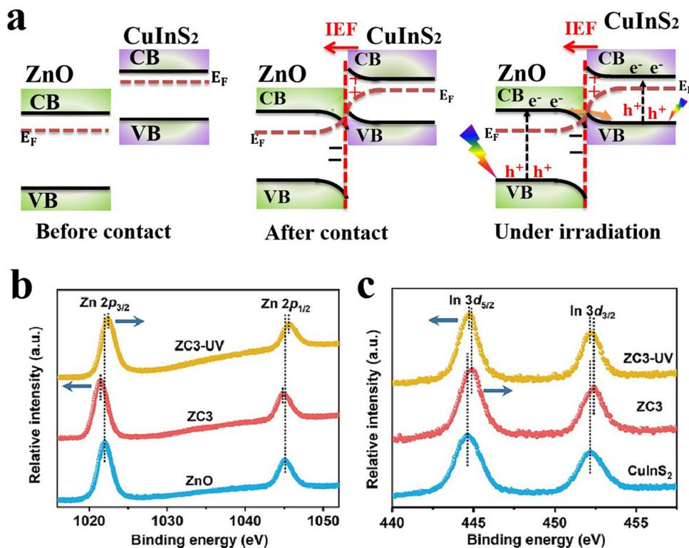
Fig. 10 (a) Schematic representation of the band structure of ZnO and CuInS<sub>2</sub> and the interfacial electron transfer between them both after contact and under light exposure. *Ex situ* and ISIXPS spectra of (b) Zn 2p and (c) In 3d recorded for ZnO, CuInS<sub>2</sub>, and the ZnO/CuInS<sub>2</sub> composite in the dark and under UV irradiation. (b) and (c) were reproduced with permission.<sup>52</sup> Copyright 2024, Wiley-VCH.
