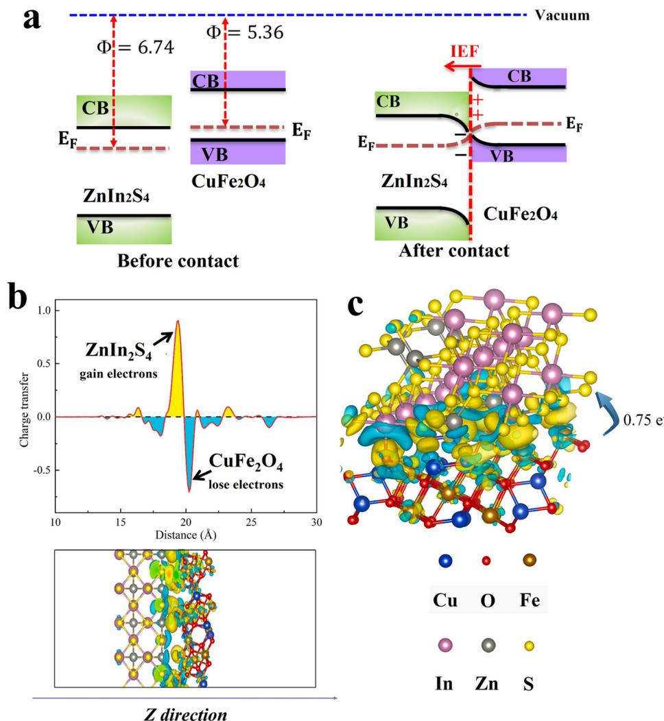
Fig. 13 (a) Schematic illustration of band structure and charge transfer between CuFe<sub>2</sub>O<sub>4</sub> and ZnIn<sub>2</sub>S<sub>4</sub>. (b) The plane average charge density difference and Z-direction differential charge density map. (c) The differential charge density map, where the yellow and cyan electron clouds represent enhanced and depleted electron density with respect to the individual components. Reproduced with permission.<sup>61</sup> Copyright 2024. Elsevier.
