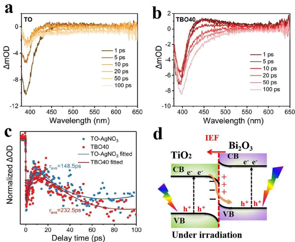
Fig. 15 fs-TAS of  $\text{TiO}_2$  (TO, a) and  $\text{TiO}_2/\text{Bi}_2\text{O}_3$ -40 (TBO40, b) recorded with 340 nm excitation. (c) Corresponding fit of the transient absorption kinetics for TO-AgNO<sub>3</sub> and TBO40 monitoring at 395 nm within a time window of 100 ps. Reproduced with permission.<sup>62</sup> Copyright 2022, Wiley-VCH. (d) Schematic illustration of S-scheme charge transfer within the TBO40.
