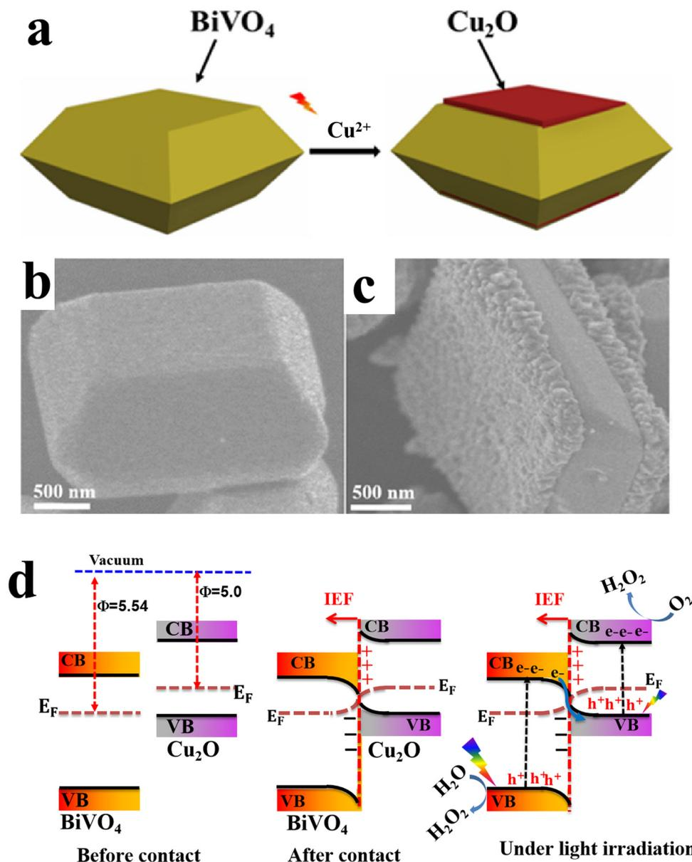
Fig. 17 (a) Scheme illustrating the preparation of the BiVO<sub>4</sub>/Cu<sub>2</sub>O S-scheme heterojunction. FESEM images of (b) BiVO<sub>4</sub> with exposed {010} and {110} facets and (c) BiVO<sub>4</sub>/Cu<sub>2</sub>O, where Cu<sub>2</sub>O is grown selectively over the {010} facets. Reproduced with permission.<sup>79</sup> Copyright 2024, Royal Society of Chemistry. (d) Schematic illustration of the charge transfer mechanism over the BiVO<sub>4</sub>/Cu<sub>2</sub>O photocatalyst.
