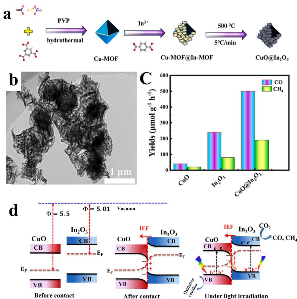
Fig. 21 (a) Schematic of the synthesis of CuO@In<sub>2</sub>O<sub>3</sub> composites; (b) TEM images of CuO@In<sub>2</sub>O<sub>3</sub> composites; (c) production rates of CO and CH<sub>4</sub> production over the studied photocatalysts. Reproduced with permission.<sup>147</sup> Copyright 2023, Elsevier. (d) Schematic layout of the band structure of the CuO/In<sub>2</sub>O<sub>3</sub> S-scheme heterojunction and proposed charge transfer dynamics and reaction mechanism.
