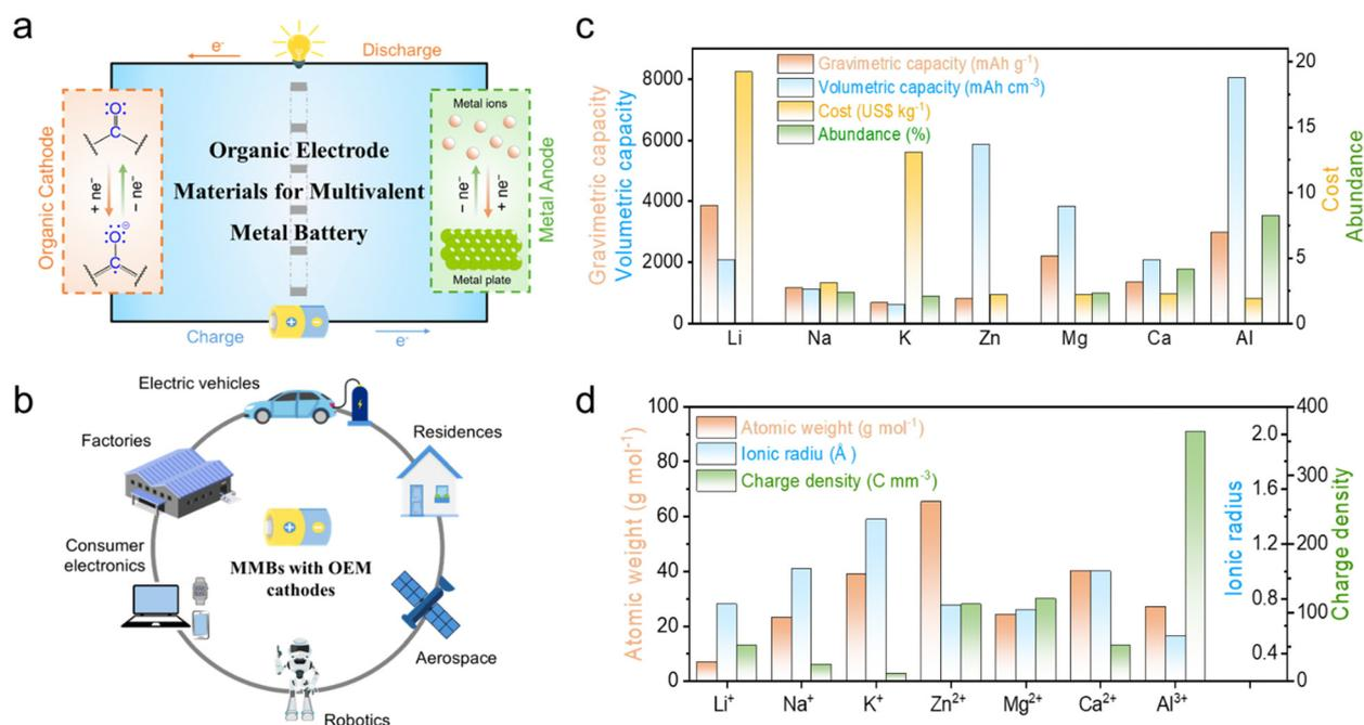
Fig. 1 (a) Schematic illustration of a typical MMB device fabricated using an OEM cathode and a multivalent metal anode. (b) Potential applications of MMBs with OEM cathodes. (c) Comparison of different monovalent and multivalent metal anodes in terms of gravimetric capacity, volumetric capacity, cost, and abundance. (d) Comparison of various monovalent and multivalent cations with regard to atomic weight, ionic radius, and charge density.
