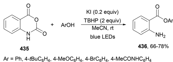
Scheme 213 Decarboxylative C–O bond formation of isatoic anhydride (435) and phenols under KI photocatalysis.
