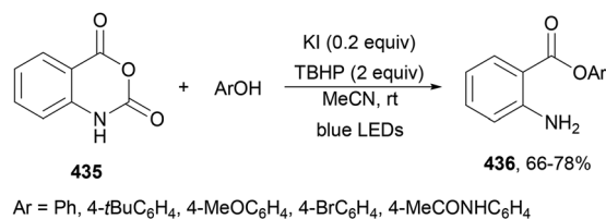
Scheme 213 Decarboxylative C–O bond formation of isoatoic anhydride ( 435 ) and phenols under KI photocatalysis.
