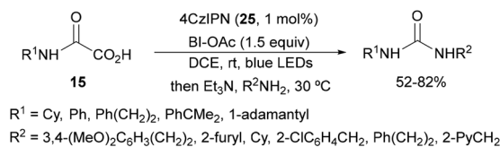
Scheme 250 Decarboxylative amidation of oxamic acids 15 with primary aliphatic amines under 4CzIPN ( 25 ) and BI-OAc photocatalysis.
