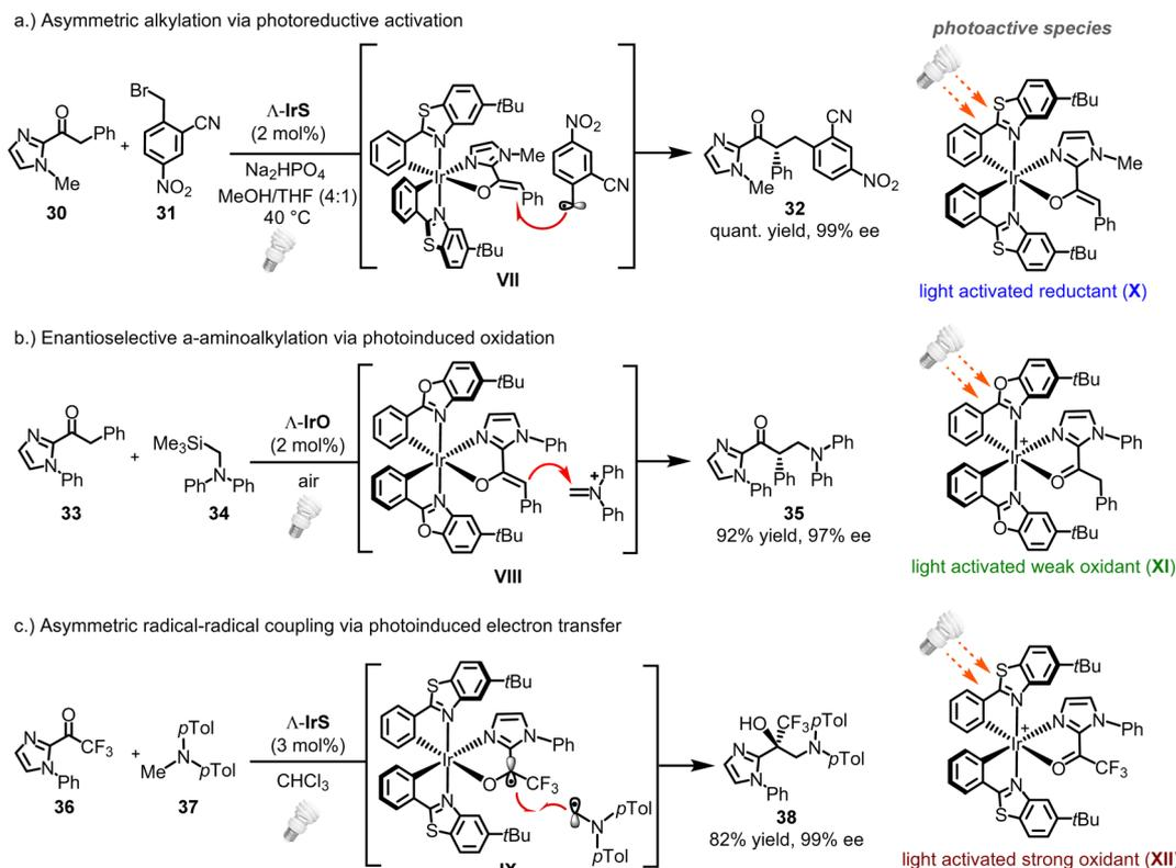
Fig. 8 Asymmetric photoredox catalysis with chiral-at-iridium complexes.
