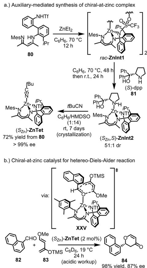
Fig. 20 Chiral-at-zinc catalyst with tetrahedral coordination sphere.
