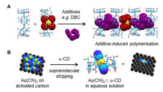
Fig. 36 Gold recovery processes using cyclodextrins: (A) additiveinduced supramolecular polymerisation, in which the addition of an additive causes the precipitation of gold-containing solids; 293,294 (B) a schematic representation of the supramolecular stripping process to remove immobilised Au(CN)<sub>2</sub><sup>-</sup> from the surface of activated carbon.<sup>295</sup>
