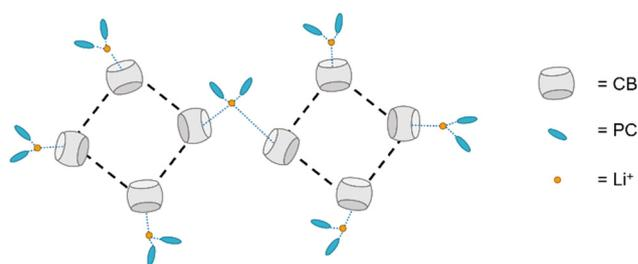
Fig. 5 Diagram depicting the intermolecular interactions between CB, PC, and  $\text{Li}^+$  ions within the electrolyte.<sup>43</sup>
