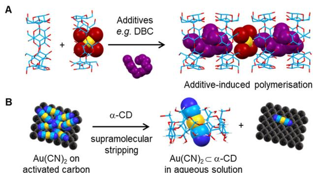
Fig. 36 Gold recovery processes using cyclodextrins: (A) additive-induced supramolecular polymerisation, in which the addition of an additive causes the precipitation of gold-containing solids;<sup>293,294</sup> (B) a schematic representation of the supramolecular stripping process to remove immobilised  $\text{Au}(\text{CN})_2^-$  from the surface of activated carbon.<sup>295</sup>
