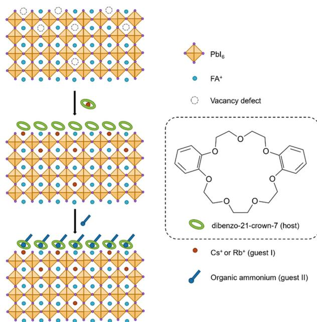
Fig. 8 Schematic of the supramolecular perovskite interface and the dual host-guest complexation strategy.<sup>59</sup>
