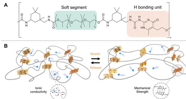
Fig. 4 (A) Chemical structure of SLIC polymer. (B) Illustration depicting the effect of stretching the SLIC polymer. (B) Is reproduced from ref. 39 under creative commons license CC BY 4.0.
