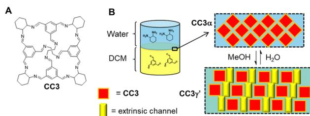
Fig. 26 (A) CC3, a porous organic cage developed by Cooper and colleagues,<sup>240</sup> (B) the formation of crystalline CC3 membranes at the interface between two immiscible solvents. The membranes reversibly transition between two crystalline phases in response to the solvent environment.<sup>244</sup>
