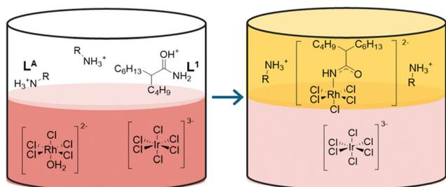
Fig. 38 A schematic depiction of the synergistic liquid-liquid extraction of rhodium ions from iridium-containing mixtures.  $L^A$  = Primene<sup>TM</sup> 81R, a mixture of isomers with  $R = \text{C}_{12-14}\text{H}_{26-30}$ .<sup>305,306</sup>
