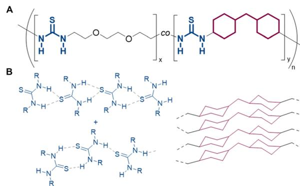
Fig. 22 (A) The structure of P(TUEG<sub>3</sub>-co-TUCy<sub>2</sub>M). (B) The hydrogen bonding patterns of thiourea and the tacking patterns of dicyclohexylmethane units.<sup>198</sup>
