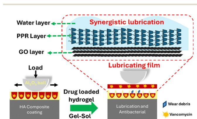
Fig. 18 The structure of hydroxyapatite (HA) hydrogel structure and gel-sol transitions under a load.<sup>143</sup>
