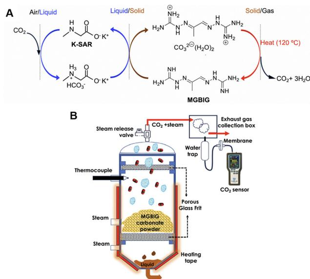
**Fig. 41** (A) A 3-step  $\text{CO}_2$  capture and release cycle based reported by Custelcean and co-workers based on the crystallisation of MBIG carbonate; (B) a schematic illustration of a continuous-flow direct-steam sorbent regeneration (DSR) protocol, reported to increase the efficiency of step iii) in part (A). Reproduced from ref. 345 in line with Elsevier's STM Permission Guidelines (2024).
