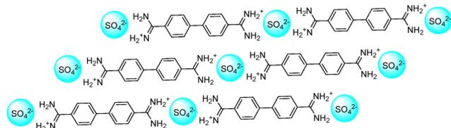
Fig. 42 Chemical representation of the sheet-like structure of the bis-amidinium sulfate precipitate reported by White and co-workers.<sup>349</sup>
