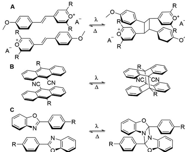
Fig. 9 Photoswitches developed by Han and co-workers which are orientated by supramolecular interactions to enable efficient cycloadditions: (A) styrylpyrilliums,<sup>63</sup> (B) 9,10-di-substituted anthracenes<sup>64</sup> and (C) *p*-functionalised phenylbenzoxazoles.<sup>65</sup>
