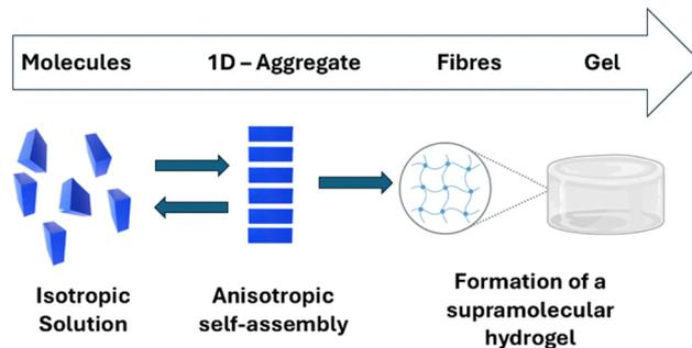
Fig. 16 The hierarchical self-assembly of a hydrogel through the non-covalent interactions of monomers.<sup>125</sup>
