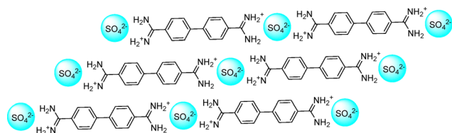
Fig. 42 Chemical representation of the sheet-like structure of the bis-amidinium sulfate precipitate reported by White and co-workers. 349
