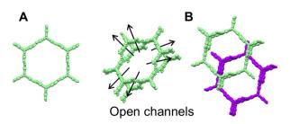
Fig. 27 (A) Two views of the hexagonal units within the 3D honeycomblike frameworks in the HOF reported by Stoddart and colleagues for hydrogen storage; (B) catenation of two hexagons linking two distinct layers (green and purple) within the HOF material. 246
