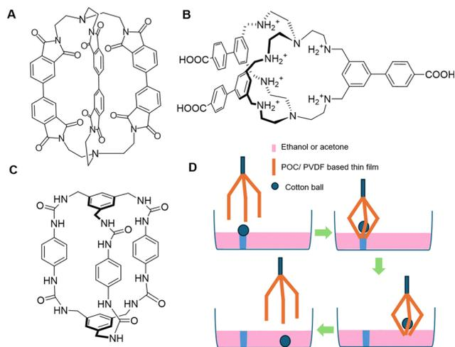
**Fig. 35** Chemical structures of the POCs used as sensors for humidity ((A) ref. 285 and (B) ref. 286) and organic vapours ((C) ref. 287). (D) A general schematic showing how a POC-based robot could grip and then release a cotton ball by having three thin films twisting around it when immersed in a chamber of either acetone or ethanol.<sup>287</sup>
