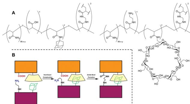
**Fig. 24** (A) The structures of the two hydrogels formed by Osaki *et al.*<sup>215</sup> containing the host–guest units of  $\beta$ -CD and Ad and the condensation units of carboxyl and amino groups. (B) Schematic overview of the host–guest interaction facilitating the correct spatial distance to facilitate the condensation reaction.
