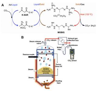
Fig. 41 (A) A 3-step CO<sub>2</sub> capture and release cycle based reported by Custelcean and co-workers based on the crystallisation of MBIG carbonate; (B) a schematic illustration of a continuous-flow direct-steam sorbent regeneration (DSR) protocol, reported to increase the efficiency of step iii) in part (A). Reproduced from ref. 345 in line with Elsevier's STM Permission Guidelines (2024)
