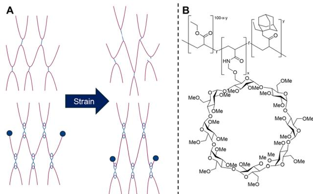
Fig. 21 (A) Schematic overview of crosslinked polymers *versus* slide-ring polymers and their differing response to strain. (B) The structure of the supramolecular elastomer, PAC $\gamma$ CDAAmMe produced by Nomimura *et al.*<sup>196</sup>
