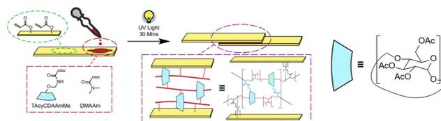
**Fig. 25** Schematic of the fabrication and structure of SC(DMAAm).<sup>216</sup>
