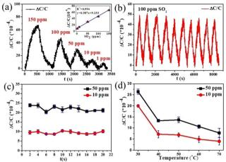
Fig. 18 (a) Detection of SO<sub>2</sub> in the range of 1 to 150 ppm concentration and linear response for the testing range of the inset; (b) reproducibility for the detection of 100 ppm SO<sub>2</sub>; (c) response ability for the sensor at 10 and 50 ppm SO<sub>2</sub> within 20 days; (d) temperature influence on the sensor performance. (Reproduced from ref. 207 Copyright 2021 with permission from John Wiley & Sons)
