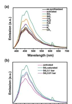
Fig. 16 (a) Comparison of solid-state emission spectra of MUF-16 exposed to different gases, and (b) comparison of solid-state emission spectra of MUF-16 exposed to different SO<sub>2</sub> pressures (Reproduced from ref. 201 Copyright 2024 with permission from American Chemical Society Under CC-BT 4.0 license).
