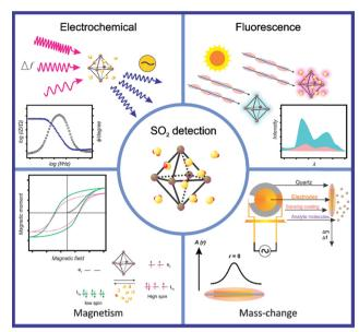
Fig. 21 MOFs applied in different characterization techniques for SO<sub>2</sub> detection.
