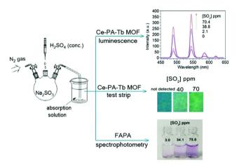
Fig. 13 Determination of SO<sub>2</sub> gas by the methods of standard formaldehyde absorbing pararosaniline (FAPA) spectrophotometry, Ce-PA-Tb luminescence and Ce-PA-Tb test strip with a 254 nm UV lamp. (Reprinted from ref. 195 Copyright 2020 with permission from Royal Society of Chemistry)
