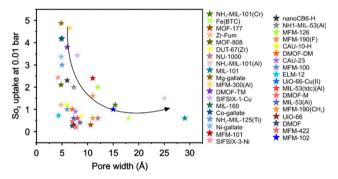
Fig. 11 Relation between SO<sub>2</sub> uptake at 0.01 bar with PLD. For references to the individual MOFs, see Table 1.
