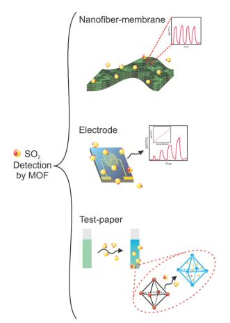
Fig. 20 MOFs applied in different assembled devices for SO<sub>2</sub> detection.
