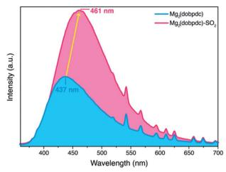
Fig. 14 Emission spectra of Mg<sub>2</sub>(dobpdc) before (blue) and after (pink) exposure to SO<sub>2</sub>. Both samples were excited with 320 nm UV light. (Reproduced from ref. 198 Copyright 2022 with permission from Royal Society of Chemistry).
