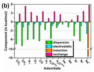
Fig. 15 Non-covalent interactions involved in CO<sub>2</sub> capture mechanisms. (a) Optimized structures and non-covalent interaction maps of CO2 molecule containing cyclo[18]carbon. (b) Components of interaction energy between cyclo[18]carbon and various chemical species obtained from symmetry-adapted perturbation theory (SAPT) calculations. Reproduced with permission.<sup>169</sup> Copyright 2021, Elsevier
