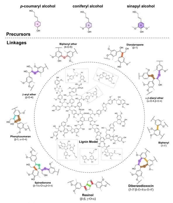
Fig. 1 Main lignin precursors (top), typical inter-unit linkages and proposed structural model macromolecule corresponding to spruce milled-wood lignin. Some of the elements shown in this illustration are inspired by ref. 32. Adapted under terms of the CC-BY 4.0 license.<sup>32</sup> Copyright 2020, Royal Society of Chemistry.
