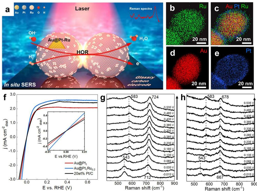
Fig. 55 (a) Schematic illustration of *in situ* SERS study of HOR on Au@PtRu. (b)–(e) Elemental mapping images of the Au@PtRu nanoparticles. (f) HOR polarization curves of commercial 20 wt% Pt/C, Au@Pt, and Au@PtRu. Sweep rate: 10 mV s<sup>-1</sup>. Rotation rate: 1600 rpm. (g) *In situ* SERS spectra of HOR on Au@PtRu and (h) the deuterium isotope experimental results. Reproduced from ref. 566 with permission. Copyright 2022 American Chemical Society.
