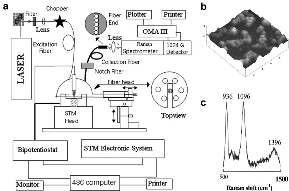
**Fig. 34** The combined STM and SERS experiments. (a) Schematics of the combined STM with Raman instrument based on the remote operation of optical fiber, which enables the simultaneous measurements of STM and SERS of an electrochemical cell. (b) STM images of a HOPG surface after the stripping of Ag. (c) A SERS spectrum of thiourea adsorbed on the surface of (b). Figures are adapted from ref. 347 and 348 Copyright 2007 Wiley. Copyright 1996 Elsevier.
