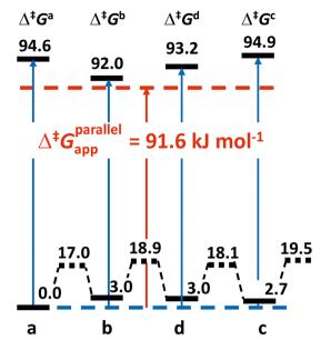
Fig. 4 Individual and apparent Gibbs energies of activation for heterolysis of 4,4'-dimethoxy benzhydrylpyridinium computed with the M06-2X/6-311+G(2d,p)/PCM = EtOH method. (Reproduced from ref. 33 with permission)
