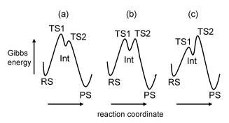
Fig. 6 Gibbs energy profiles to illustrate change in rate-limiting step for reaction of semicarbazide with substituted aromatic aldehydes: (a) ratelimiting addition (step 1), (b) steps 1 and 2 equally rate-limiting, (c) ratelimiting dehydration.
