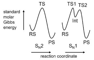
Fig. 1 Energy profiles for nucleophilic substitution reactions following (left) S<sub>N</sub>2 and (right) S<sub>N</sub>1 mechanisms.
