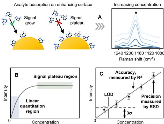
Fig. 2 The key analytical figures of merit in SERS quantitation. (A) Schematic illustrations of the adsorption of analyte molecules on the enhancing substrate surface and the corresponding change in the SERS signal of the analyte observed. (B) and (C) Schematic illustration of a typical calibration curve between analyte concentration and signal intensity from SERS analysis. (C) Schematic illustration of the linear region of the calibration curve.
