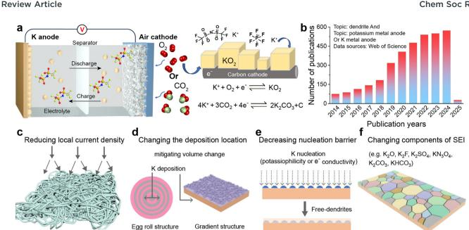
Fig. 2 (a) Schematic illustration of potassium-air batteries. (b) Number of publications related to potassium metal anodes from 2014 to 2025. (c)-(f) Solutions for potassium metal anodes to address infinite volume changes and dendrite growth.
