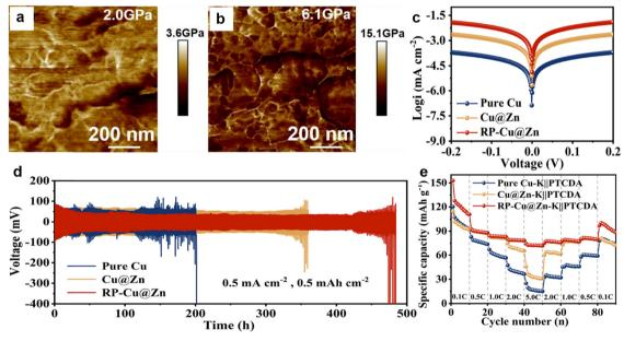
Fig. 24 The distribution of Young's modulus on the surface of (a) bare K and (b)  $K_x P_y \alpha K$ . Reproduced with permission from ref. 228. Copyright 2021, Wiley-VCH. (c) Tafel curves and (d) cycling stability of the pure Cu-K, Cu@Zn-K, and RP-Cu@Zn-K. (e) Rate performance for Pure Cu-K||PTCDA, Cu@Zn-K, and RP-Cu@Zn-K. K||PTCDA, and RP-Cu@Zn-K||PTCDA full cells. Reproduced with permission from ref. 229. Copyright 2024, Elsevier.
