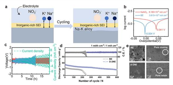
Fig. 34 (a) Schematic diagram of enhanced interface formation. (b) Tafel curves of K||K symmetric cells. (c) Rate current density test of K||K symmetric cells. Reproduced with permission from ref. 273. Copyright 2023, Elsevier. (d) Cycling performance of the full-cells in different electrolytes. (e) SEM images of cycled K-metal anodes and separators (polymer membrane) from K||FeHCF full cells. Reproduced with permission from ref. 274. Copyright 2024, Elsevier.
