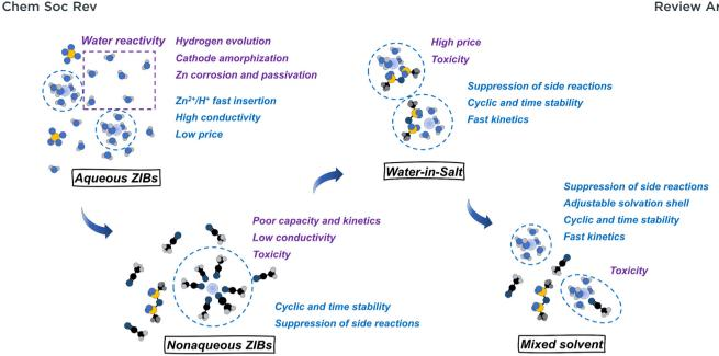
Fig. 20 Research development on rechargeable Zn-ion batteries electrolytes.
