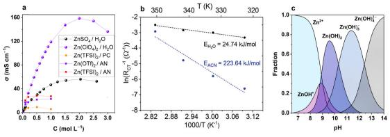
Fig. 3 Electrolytes for Zn-ion batteries. (a) Comparison of conductivity for some aqueous and nonaqueous electrolytes. 74-76 (b) Charge transfer activation energy at Zn metal interface in nonaqueous vs. aqueous zinc electrolyte. Reproduced from ref. 32 with permission from the Royal Society of Chemistry. Copyright 2018. (c) Distribution of Zn(II) hydroxo-complexes at infinite dilution at 298 K.<sup>77</sup>
