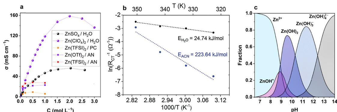
Fig. 3 Electrolytes for Zn-ion batteries. (a) Comparison of conductivity for some aqueous and nonaqueous electrolytes.<sup>74–76</sup> (b) Charge transfer activation energy at Zn metal interface in nonaqueous vs. aqueous zinc electrolyte. Reproduced from ref. 32 with permission from the Royal Society of Chemistry. Copyright 2018. (c) Distribution of Zn(II) hydroxo-complexes at infinite dilution at 298 K.<sup>77</sup>
