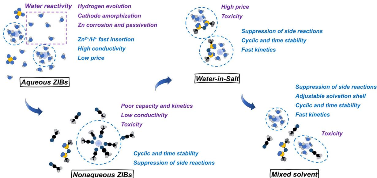
Fig. 20 Research development on rechargeable Zn-ion batteries electrolytes.
