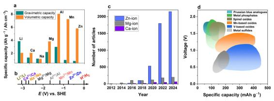
Fig. 1 Comparison of several ion storage systems. (a) Volumetric and gravimetric specific capacities of lithium, sodium, and some multivalent metals. (b) Standard reduction potentials of ions to corresponding metals. (c) Number of articles mentioning multivalent-ion battery in title, and (d) operation voltage vs. specific capacity for Zn-ion batteries. 18,22,23
