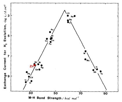
Fig. 74 Volcano plot for the HER. The intermediate Zn metal-hydrogen bond formed during the electrochemical reaction is weak, resulting in a high overpotential (low exchange current) for the HER.813 Reprinted with permission from Journal of Electroanalytical Chemistry and Interfacial Electrochemistry.
