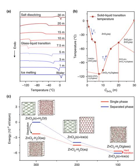
Fig. 49 (a) Differential scanning calorimetry curves and (b) obtained phase transition diagram of a ZnCl<sub>2</sub>/water binary system. (c) Calculated transition state in the transformation from the glass state to the separated crystalline state of a 7.5 m  $ZnCl_2/H_2O$  solution. See Reprinted with permission from Nature Communications
