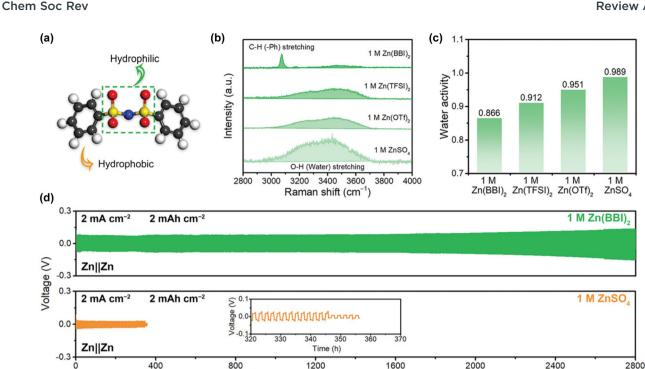
Fig. 54 (a) Atomic structure of the BBI<sup>-</sup> anion, with C, H, O, N, and S atoms denoted in black, light-gray, red, blue, and yellow, respectively. (b) Raman spectra and (c) water activities of various Zn solutions. (d) Cycling performance of symmetric Zn|Zn cells in 1 M Zn(BBI)<sub>2</sub> and 1 M ZnSO<sub>4</sub> electrolytes under the given conditions. 598 Reprinted with permission from Advanced Materials.
