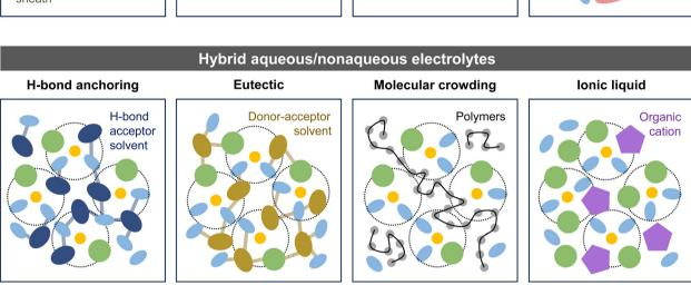
Fig. 41 Schematic comparison of the solution structures of aqueous and hybrid aqueous/nonaqueous electrolytes using diverse strategies
