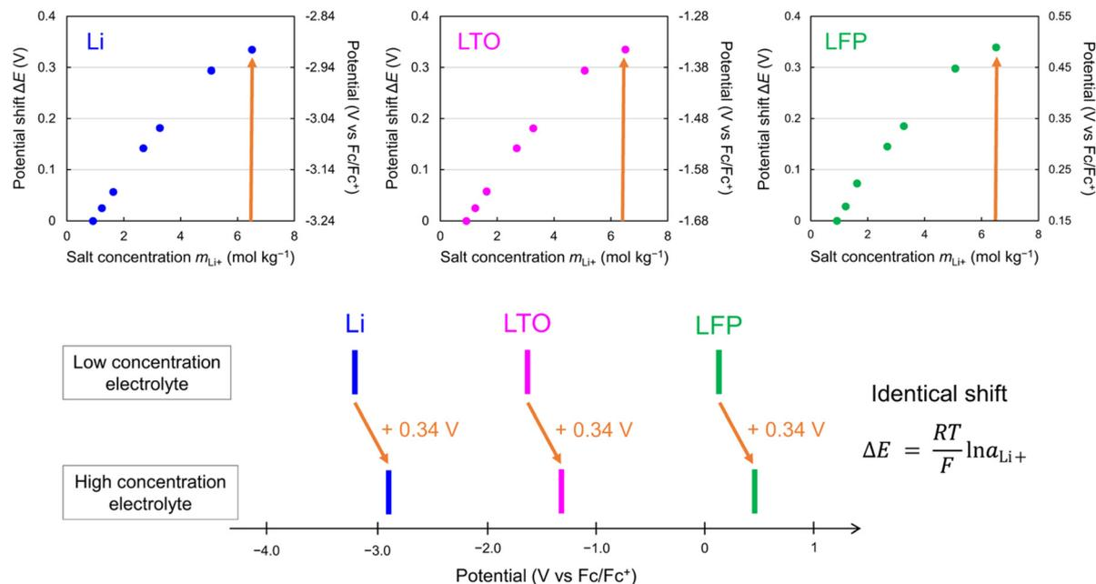
Fig. 37 Simultaneous shift in the redox/reaction potentials with identical magnitude.<sup>343</sup> To maximize the battery performance, the overall potential diagram of full cells and the operating potential window of electrolytes should be optimized.<sup>48,342,343</sup> Reprinted with permission from *Nature Communications*.
