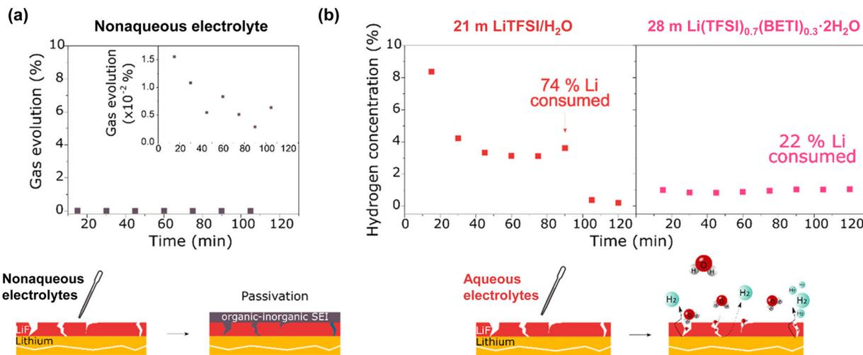
Fig. 32 Estimated gas evolution during exposure of LiF-protected Li metal to (a) nonaqueous and (b) highly salt-concentrated aqueous electrolytes.<sup>333</sup> Reprinted with permission from ACS Energy Letters.
