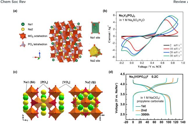
Fig. 28 Crystal structures and electrochemical properties of (a) and (b) Na<sub>3</sub>V<sub>2</sub>(PO<sub>4</sub>)<sub>3</sub><sup>313,316</sup> and (c) and (d) Na<sub>3</sub>(VOPO<sub>4</sub>)<sub>2</sub>F.<sup>317</sup> Reprinted with permission from Electrochemistry (a), ChemElectroChem (b), and Joule (c) and (d).
