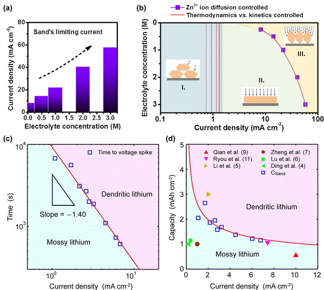
Fig. 73 (a) and (b) Sand's limiting current densities for Zn plating in aqueous ZnSO<sub>4</sub> electrolytes with different concentrations. The inset, model III, represents Zn dendrite growth.<sup>811</sup> (c) and (d) Sand's time and capacity for Li plating in nonaqueous Li electrolytes at various current densities.<sup>812</sup> Reprinted with permission from *Angewandte Chemie International Edition* (a) and (b) and *Energy & Environmental Science* (c) and (d).
