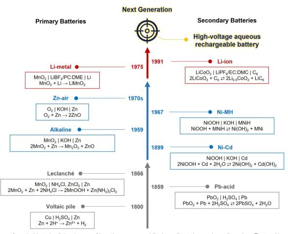
Fig. 1 History of practical batteries, listing the year of invention or commercialization, cell notations, and overall reactions. The transition of battery electrolytes is highlighted in gray (acidic aqueous electrolyte), blue (alkaline aqueous electrolyte), and red (nonaqueous electrolyte) arrows. One of the current technical targets is the development of aqueous rechargeable batteries with high voltage (high energy density), high safety, and high sustainability.
