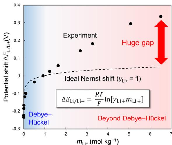
Fig. 35 Anomalous shift in the Li/Li<sup>+</sup> redox potential. The large gap between the experimentally obtained and calculated potential shifts cannot be explained by either the classical Debye–Hückel theory or its phenomenological extensions.<sup>342,343</sup> Reprinted with permission from *Nature Communications*.
