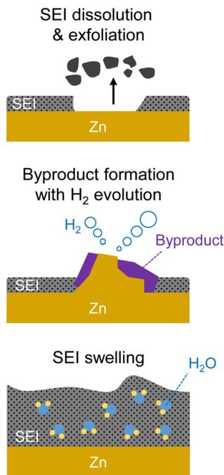
Fig. 57 Various SEI degradation modes in aqueous electrolytes.
