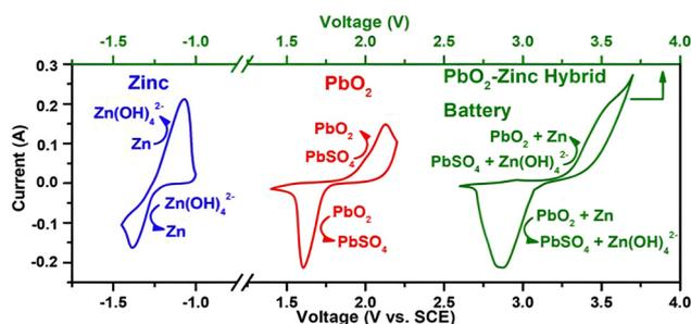
Fig. 79 Cyclic voltammograms of Zn in an alkaline electrolyte (blue),  $\text{PbO}_2$  in an acidic electrolyte (red), and a  $\text{PbO}_2|\text{Zn}$  hybrid battery with an electrolyte decoupling system (alkaline anolyte and acidic catholyte) (green) under a scan rate of  $10 \text{ mV s}^{-1}$ .<sup>867</sup> Reprinted with permission from *Angewandte Chemie International Edition*.
