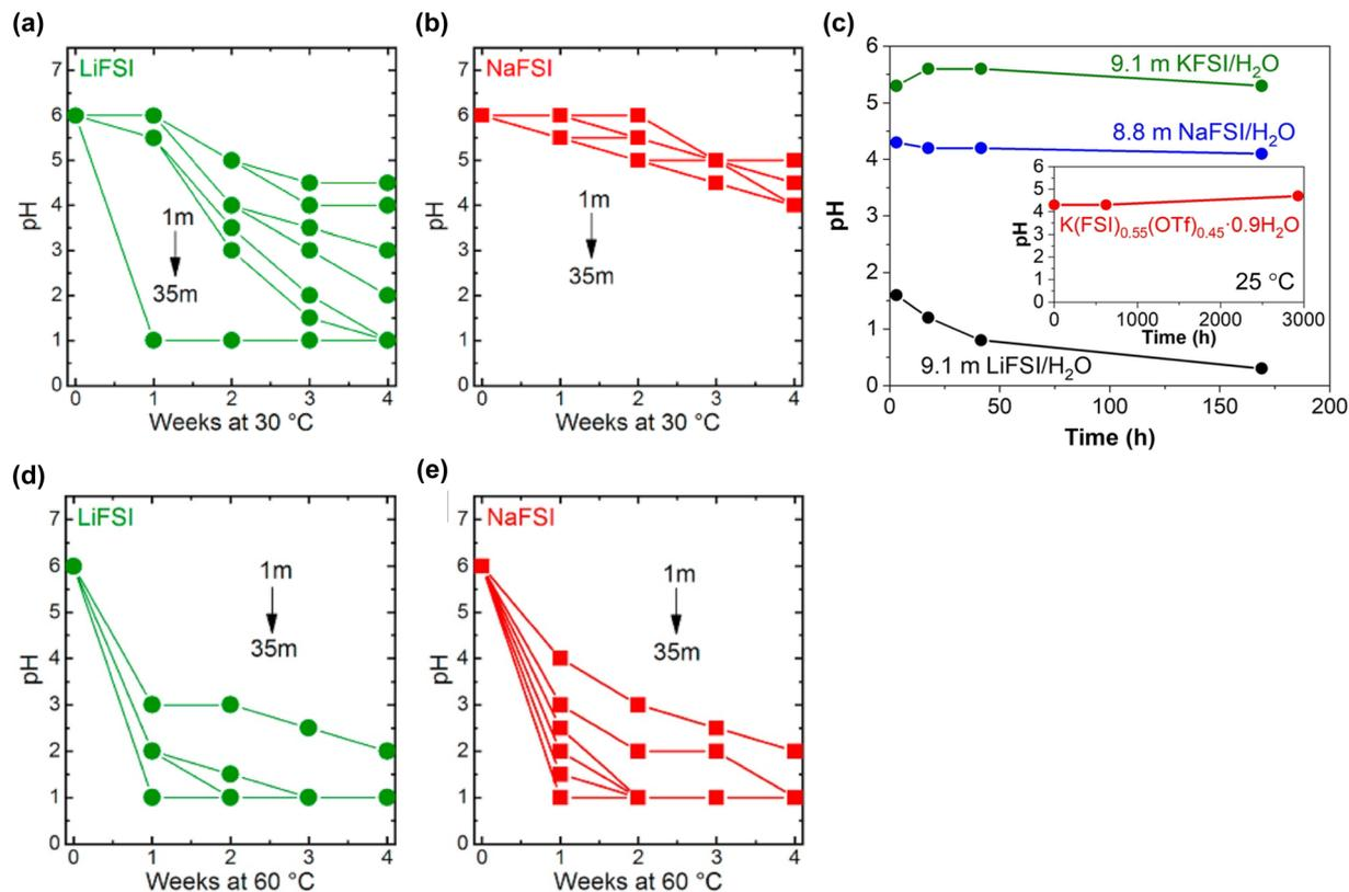
Fig. 39 pH levels of FSI<sup>-</sup> anion-based aqueous electrolytes under various salt concentrations and temperature conditions.<sup>169,170</sup> Reprinted with permission from *Electrochimica Acta* (a), (b), (d) and (e) and *Electrochemistry Communications* (c).
