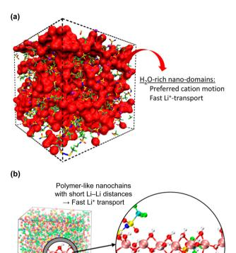
Fig. 16 (a) and (b) Carrier ion transport via vehicle-type and/or hopping-type mechanism in highly salt-concentrated aqueous electrolytes.  $^{213,214}$ Reprinted with permission from ACS Nano (a) and Journal of the American Chemical Society (b)
