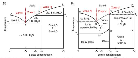
Fig. 18 (a) Equilibrium binary H<sub>2</sub>O-salt and (b) non-equilibrium binary H<sub>2</sub>O-salt phase diagrams of aqueous solutions.<sup>227</sup> Reprinted with permission from Nano Research Energy.
