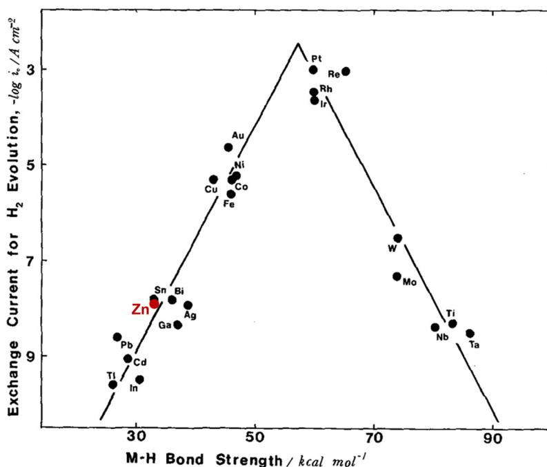
Fig. 74 Volcano plot for the HER. The intermediate Zn metal-hydrogen bond formed during the electrochemical reaction is weak, resulting in a high overpotential (low exchange current) for the HER.<sup>813</sup> Reprinted with permission from *Journal of Electroanalytical Chemistry and Interfacial Electrochemistry*.
