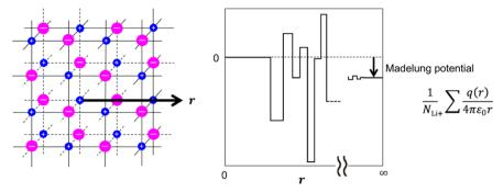
Liquid Madelung potential ( $E_{LM}$ ) for low concentration electrolyte solutions
