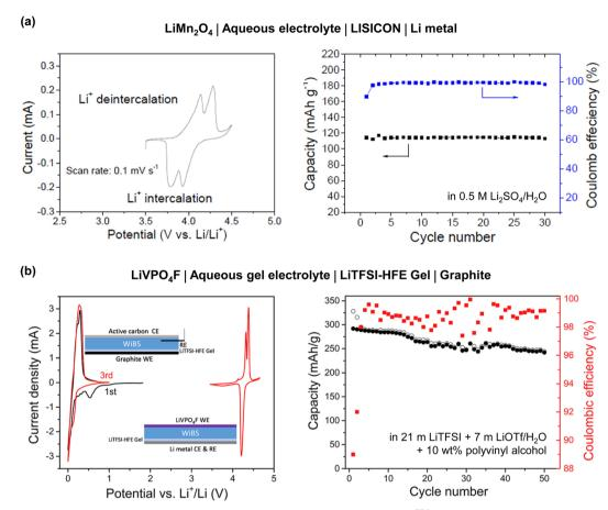
Fig. 33 Electrochemical properties of the (a) LiMn<sub>2</sub>O<sub>4</sub>|LISICON|Li full cell in 0.5 M Li<sub>2</sub>SO<sub>4</sub>/H<sub>2</sub>O<sub>336</sub> and (b) LiVPO<sub>4</sub>F|LiTFSI-HFE gel|graphite full cell in 21 m LiTFSI + 7 m LiOTf/H<sub>2</sub>O + 10 wt% polyvinyl alcohol electrolyte.<sup>337</sup> Reprinted with permission from Scientific Reports (a) and Joule (b).
