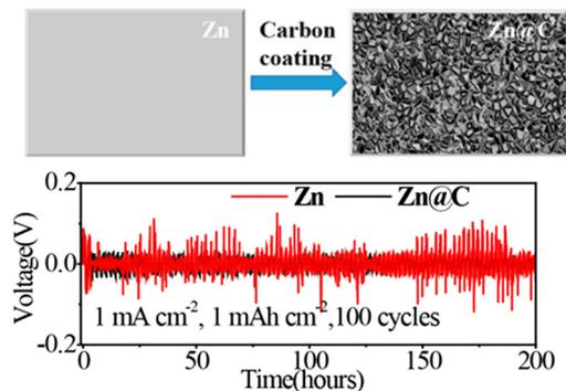
Fig. 58 Prevention of Zn dendrite formation by carbon coating.<sup>651</sup> Reprinted with permission from *ACS Applied Materials & Interfaces*.
