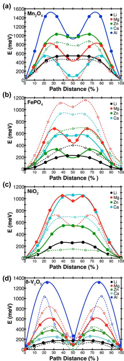
Fig. 45 Computational calculation results for the migration energies of monovalent and multivalent ions in (a) spinel  $\text{Mn}_2\text{O}_4$ , (b) olivine  $\text{FePO}_4$ , (c) layered  $\text{NiO}_2$ , and (d) orthorhombic  $\delta\text{-V}_2\text{O}_5$  structures.<sup>435</sup> Reprinted with permission from *Chemistry of Materials*.
