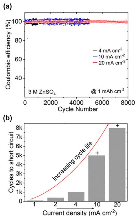
Fig. 71 (a) Coulombic efficiencies of Zn plating and stripping in  $\text{Ti}|\text{3 M ZnSO}_4/\text{H}_2\text{O}|\text{Zn}$  cells at various current densities. (b) Chart representation showing a drastic increase in the Coulombic efficiency with increasing current density.<sup>804</sup> Reprinted with permission from *ACS Applied Materials & Interfaces*.
