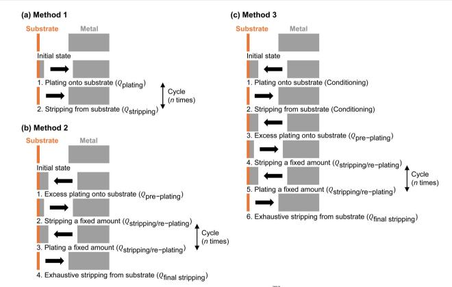
Fig. 68 (a)-(c) Protocols to estimate the Coulombic efficiency of metal plating and stripping. Reprinted with permission from Advanced Energy Materials.
