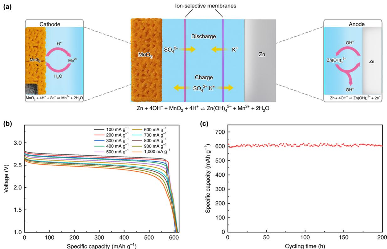
Fig. 78 (a) The working mechanism of an electrolyte-decoupled  $\text{MnO}_2|\text{Zn}$  battery. (b) and (c) Discharge voltage profiles and long-term cycling stability of the cell.<sup>862</sup> Reprinted with permission from *Nature Energy*.
