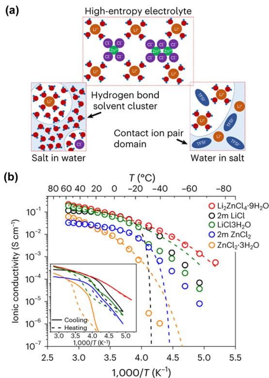
Fig. 50 (a) Illustration of solution structures in different electrolytes: salt-in-water, water-in-salt, and high-entropy electrolytes. (b) Ionic conductivity of the  $\text{Li}_2\text{ZnCl}_4 \cdot 9\text{H}_2\text{O}$  electrolyte compared with those of different concentrated and diluted aqueous solutions.<sup>586</sup> Reprinted with permission from *Nature Sustainability*.
