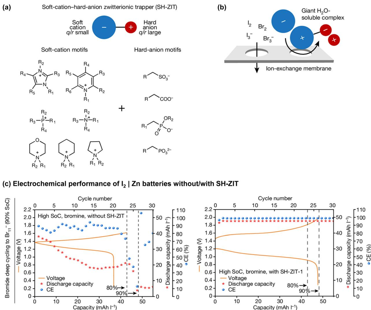
**Fig. 77** (a) Design principle and (b) proposed reaction mechanism of soft-hard zwitterionic trappers (SH-ZITs) with polyhalides, leading to the formation of soluble phases and reduced permeability. (c) Electrochemical performance of 2 M KBr catholyte charged to 80–90% state of charge without/with 2 M SH-ZIT. Excess 1,1'-bis[3-sulfonatopropyl]-4,4'-bipyridinium and 2 M KBr anolyte were utilized with cation-exchange membranes.<sup>858</sup> Reprinted with permission from *Nature*.
