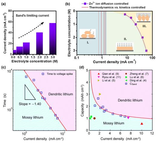
Fig. 73 (a) and (b) Sand's limiting current densities for Zn plating in aqueous ZnSO4 electrolytes with different concentrations. The inset, model III, represents Zn dendrite growth. 811 (c) and (d) Sand's time and capacity for Li plating in nonaqueous Li electrolytes at various current densities. 812 Reprinted with permission from Angewandte Chemie International Edition (a) and (b) and Energy & Environmental Science (c) and (d).
