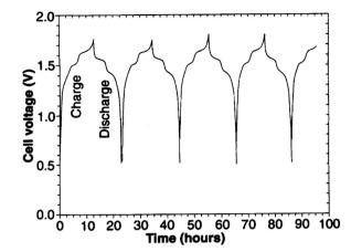
Fig. 3 Charge and discharge curves of a prototype aqueous LiMn<sub>2</sub>O<sub>4</sub>|-VO<sub>2</sub>(B) battery. 17,33 Reprinted with permission from Journal of The Electrochemical Society.
