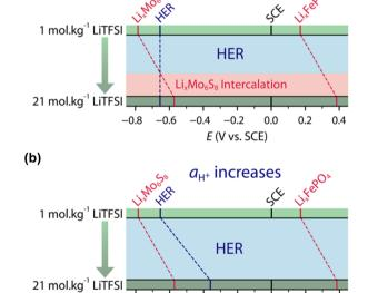
Fig. 13 Electrode potential shifts (a) without and (b) with consideration of the H<sup>+</sup> activity in LiTFSI/H<sub>2</sub>O electrolytes. 192,193 Reprinted with permission from The Journal of Chemical Physics
