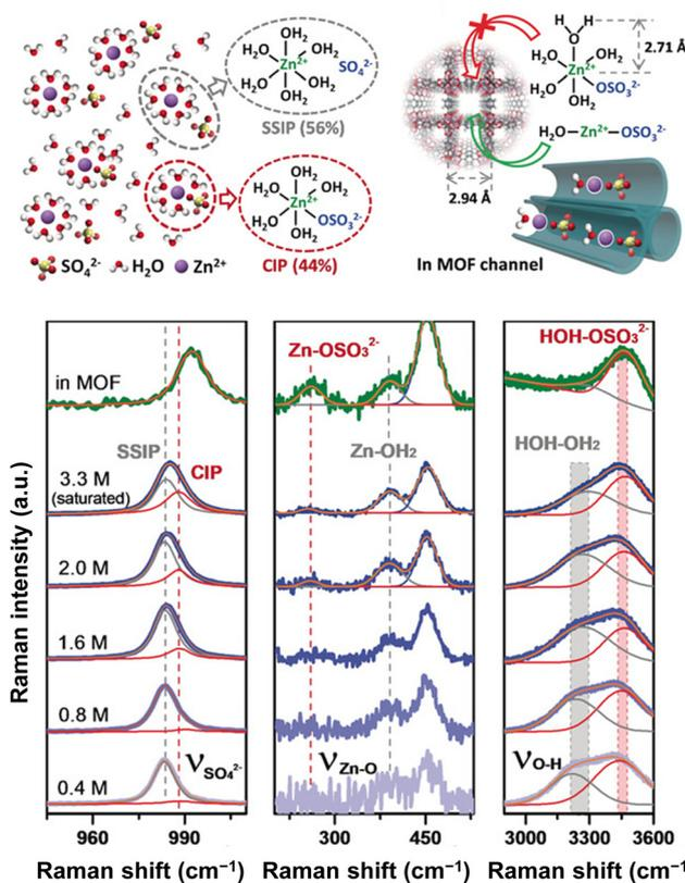
Fig. 61 Construction of a super-saturated  $\text{ZnSO}_4$  electrolyte in metal-organic-framework channels, demonstrated by Raman spectroscopy.<sup>735</sup> Reprinted with permission from *Angewandte Chemie International Edition*.
