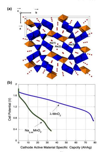
Fig. 27 Crystal structure of Na $_{0.44}$ MnO $_2$ . $^{311}$  (b) Galvanostatic discharge curves of Na $_{0.44}$ MnO $_2$  and  $\lambda$ -MnO $_2$  in 1 M Na $_2$ SO $_4$ /H $_2$ O. $^{312}$  Reprinted with permission from Sensors and Actuators B (a) and Journal of Power Sources (b)
