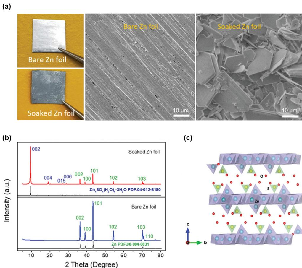
Fig. 48 (a) Photographs and SEM images and (b) XRD patterns before and after soaking Zn metal in a 1 m  $ZnSO_4$  solution for several days. (c) Crystal structure of the byproduct,  $Zn_4SO_4(OH)_6 \cdot 3H_2O$ .<sup>444</sup> Reprinted with permission from *Advanced Functional Materials*.
