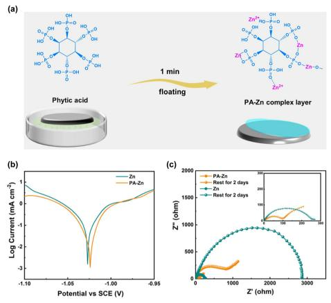
Fig. 65 (a) Preparation of phytic acid-treated Zn metal (PA-Zn). (b) Tafel curves showing increased corrosion potential in PA-Zn. (c) Nyguist plots demonstrating a significant difference in the surface charge-transfer resistance between bare Zn and PA-Zn before and after immersion in the 2 M ZnSO<sub>4</sub> solution for two days.<sup>786</sup> Reprinted with permission from ACS Applied Materials & Interfaces
