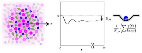
Fig. 36 Concept of the (a) classical Madelung potential for inorganic crystals, (b) and (c) liquid Madelung (Ewald) potential, represented by the sum of overall electrostatic interactions between the surrounding ions and/or solvents and the central Li<sup>+</sup> in the electrolyte. <sup>343</sup> Reprinted with permission from Nature Communications.
