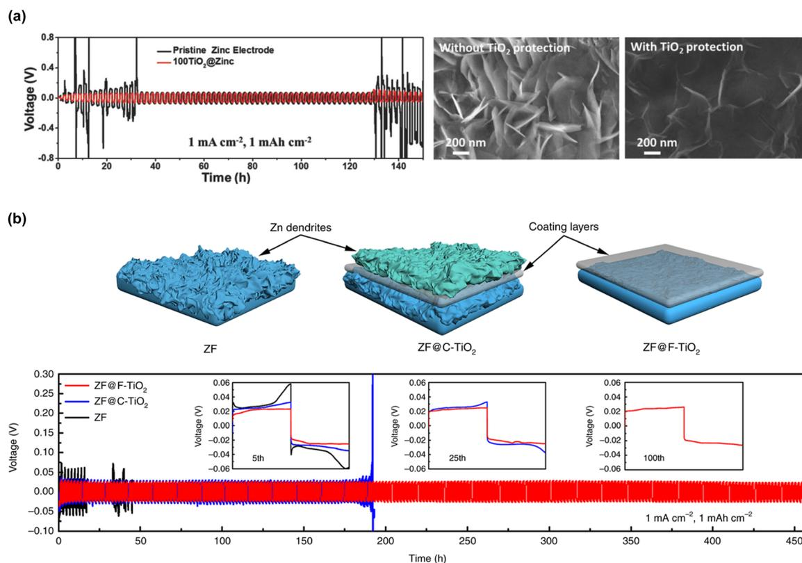
Fig. 59 (a) Performance of Zn|Zn symmetric cells with and without an 8 nm-thick TiO<sub>2</sub> coating on Zn metal.<sup>611</sup> (b) Schematic of Zn plating and Zn|Zn symmetric cell results under different coating conditions. ZF, C-TiO<sub>2</sub>, and F-TiO<sub>2</sub> correspond to Zn foil, commercial TiO<sub>2</sub>, and highly (001) facet-exposed TiO<sub>2</sub>, respectively.<sup>671</sup> Reprinted with permission from *Advanced Materials Interfaces* (a) and *Nature Communications* (b).
