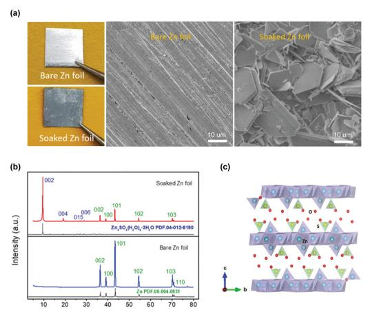
Fig. 48 (a) Photographs and SEM images and (b) XRD patterns before and after soaking Zn metal in a 1 m ZnSO<sub>4</sub> solution for several days. (c) Crystal structure of the byproduct, Zn<sub>4</sub>SO<sub>4</sub>(OH)<sub>6</sub>·3H<sub>2</sub>O.<sup>444</sup> Reprinted with permission from Advanced Functional Materials.
