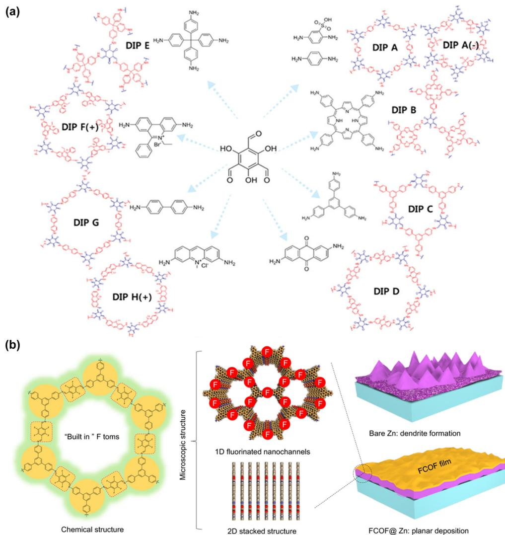
Fig. 62 (a) Structures of diverse covalent organic frameworks (COFs), formed from the 1,3,5-triformylphloroglucinol precursor and various aromatic amine linkers.<sup>740</sup> (b) Suppression of Zn dendrite formation by a fluorinated COFs film.<sup>741</sup> Reprinted with permission from *Advanced Materials* (a) and *Nature Communications* (b).
