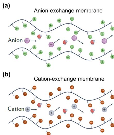
Fig. 80 Schematic representation of ion transport mechanisms in (a) anion- and (b) cation-exchange membranes.<sup>831</sup> Reprinted with permission from *Nature Review Chemistry*.
