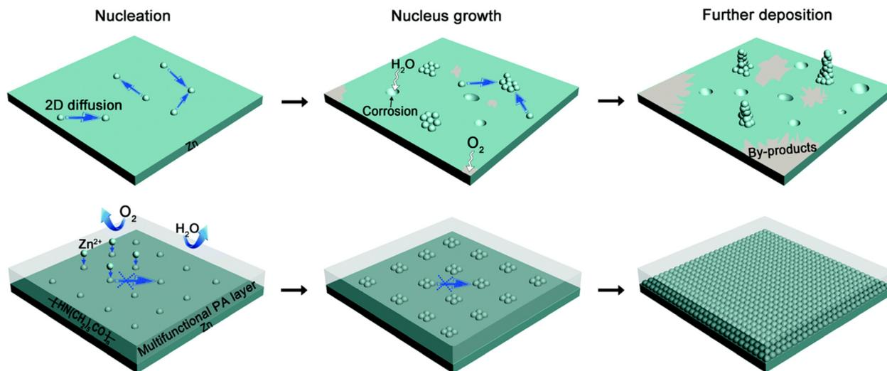
Fig. 63 Mechanism of suppressed Zn dendrite growth with a multifunctional polymeric interphase composed of polyamide and  $\text{Zn}(\text{OTf})_2$ . Initial Zn nucleation was delocalized by the introduced polymeric interphase.<sup>752</sup> Reprinted with permission from *Energy & Environmental Science*.
