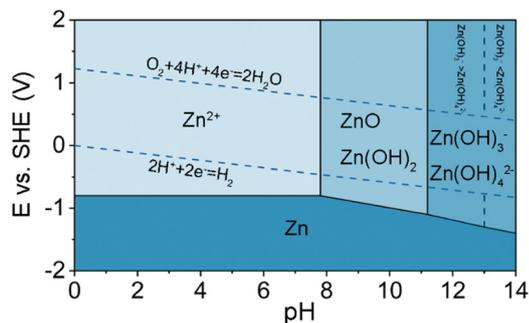
Fig. 47 Pourbaix diagram of Zn in aqueous electrolytes.<sup>577,580</sup> Reprinted with permission from *Journal of Materials Chemistry A*.
