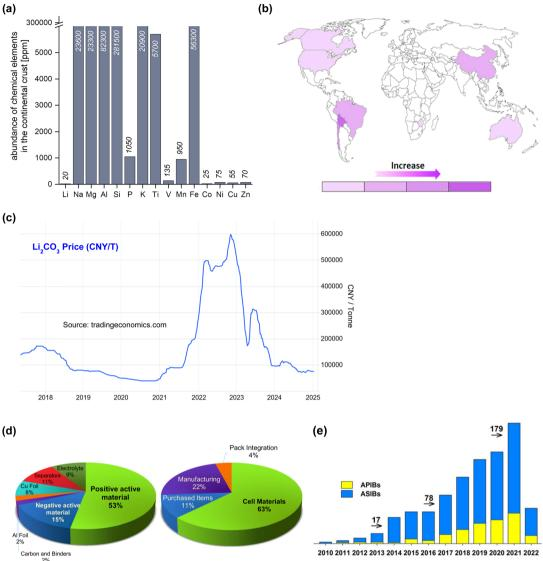
Fig. 8 (a) Elemental abundance in Earth's crust, 92 (b) distribution of Li resources on Earth, 96 (c) evolution of the price of Li per metric ton of Li<sub>2</sub>CO<sub>3</sub> equivalent units,<sup>97</sup> (d) the estimated cost percentage of Li-ion electric vehicle battery components,<sup>98</sup> (e) number of papers published on aqueous Naand K-ion batteries. <sup>99</sup> Reprinted with permission from Energy Storage Materials (b) and Journal of Physics: Energy (e).
