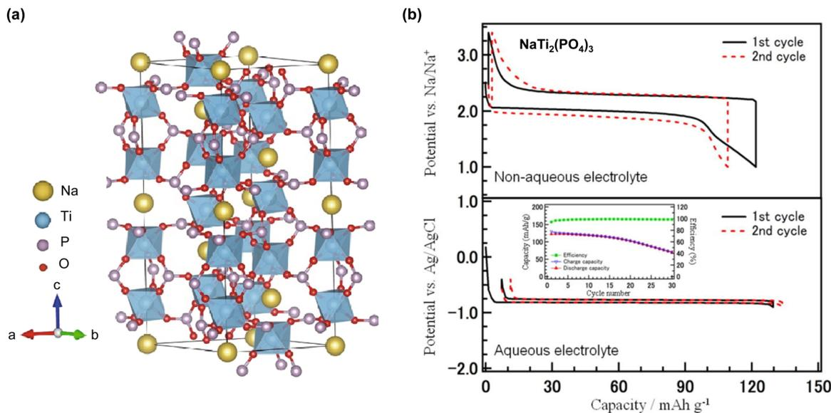
Fig. 29 (a) and (b) Crystal structure and electrochemical properties of  $\text{NaTi}_2(\text{PO}_4)_3$ .<sup>318,319</sup> The sodiation/desodiation curves of  $\text{NaTi}_2(\text{PO}_4)_3$  were obtained in 1 M  $\text{NaClO}_4$ /ethylene carbonate : dimethyl carbonate (1 : 1, v : v) and 2 M  $\text{Na}_2\text{SO}_4/\text{H}_2\text{O}$ . Reprinted with permission from *Nano-micro Letters* (a) and *Journal of The Electrochemical Society* (b).
