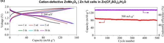
Fig. 52 Cyclic voltammograms of the Zn plating/stripping in (a) 1 M Zn(OTf)<sub>2</sub> and (b) 1 M ZnSO<sub>4</sub> solutions. (c) Galvanostatic charge and discharge curves at 50 mA  $g^{-1}$  and (d) long-term cycling performance of carbon-coated cation-defective ZnMn<sub>2</sub>O<sub>4</sub>|Zn full cells in 3 M Zn(OTf)<sub>2</sub>/H<sub>2</sub>O at 500 mA  $g^{-1.595}$ Reprinted with permission from Journal of the American Chemical Society
