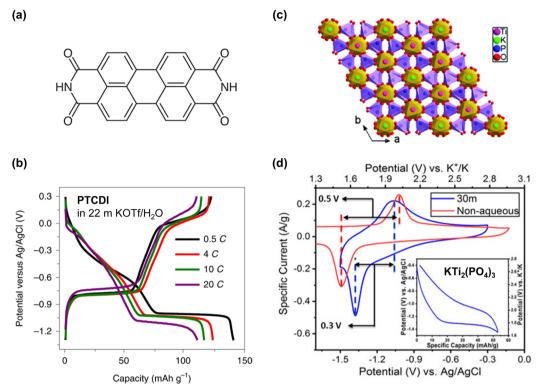
Fig. 31 (a) and (b) Molecular structure and electrochemical properties of PTCDI.<sup>122</sup> (c) and (d) Crystal structure and electrochemical properties of KTi<sub>2</sub>(PO<sub>4</sub>)<sub>3</sub> in 30 m KOAc/H<sub>2</sub>O. <sup>188,330</sup> Reprinted with permission from Nature Energy (a) and (b), Chemical Communications (c) and ACS Energy Letters (d).
