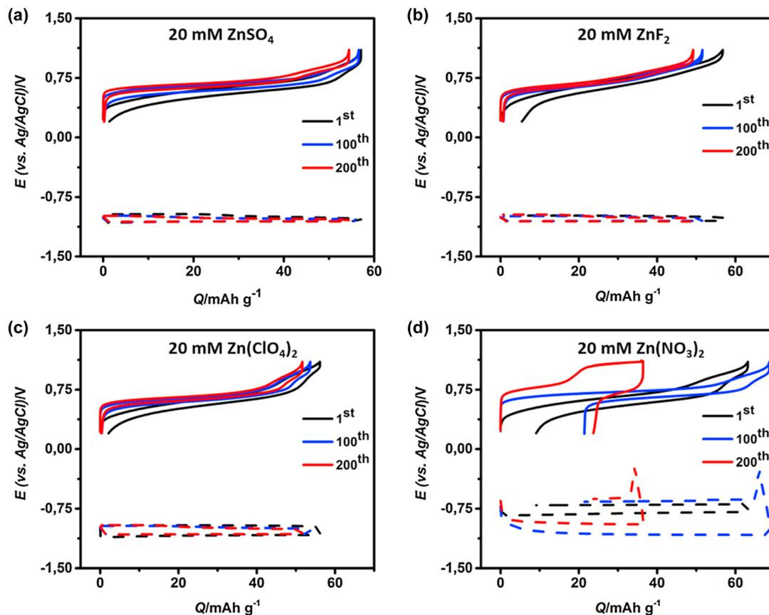
Fig. 51 Potential profiles of the copper hexacyanoferrate cathode (solid line) and Zn-metal anode (dashed line) in (a) 20 mM  $\text{ZnSO}_4$ , (b) 20 mM  $\text{ZnF}_2$ , (c) 20 mM  $\text{Zn}(\text{ClO}_4)_2$ , and (d) 20 mM  $\text{Zn}(\text{NO}_3)_2$  solutions.<sup>592</sup> Reprinted with permission from *Electrochimica Acta*.
