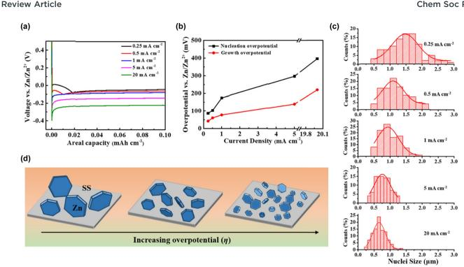
Fig. 72 (a) Voltage profiles of galvanostatic Zn plating on SUS. (b) Variation in nucleation and growth overpotentials with respect to the current density. (c) Histograms of Zn particle sizes after plating with a capacity of 0.1 mA h cm<sup>-2</sup>. (d) Schematic of Zn growth at different overpotentials. 805 Reprinted with permission from ACS Applied Materials & Interfaces
