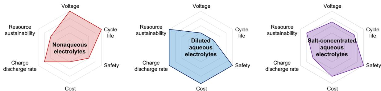
Fig. 4 Advantages and limitations of nonaqueous, diluted aqueous, and salt-concentrated aqueous electrolytes.
