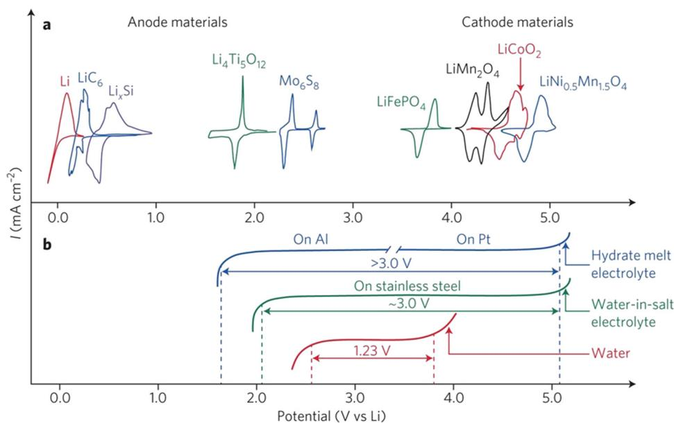
Fig. 5 (a) and (b) Broadened operating potential window in highly salt-concentrated aqueous electrolytes, such as water-in-salt (21 m  $\text{LiTFSI}/\text{H}_2\text{O}$ ) and dihydrate melt (28 m  $\text{Li}(\text{TFSI})_{0.7}(\text{BETI})_{0.3}\cdot 2\text{H}_2\text{O}$ ), contributing to an increase in output voltage of aqueous batteries.<sup>88</sup> Reprinted with permission from *Nature Energy*.
