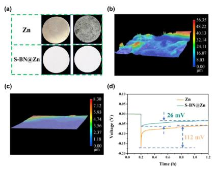
Fig. 64 (a)-(c) Photographs and three-dimensional distribution images of bare Zn and sulfonate group-modified boron nitride-coated Zn(S-BN@Zn) before and after 50 cycles in symmetric cells. (d) Decreased initial Zn nucleation overpotential on S-BN@Zn.<sup>778</sup> Reprinted with permission from *Energy* Storage Materials.
