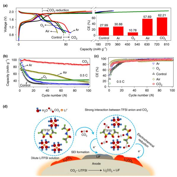
Fig. 42 (a)–(c) Electrochemical performance of an aqueous  $LiMn_2O_4|Mo_6S_8$  full cell in 5 m  $LiTFSI/H_2O$  saturated by various gases, and (d) the schematic of the SEI formation mechanism in a 5 m LiTFSI/H<sub>2</sub>O + sat. CO<sub>2</sub> electrolyte. 420 Reprinted with permission from Nature Chemistry.
