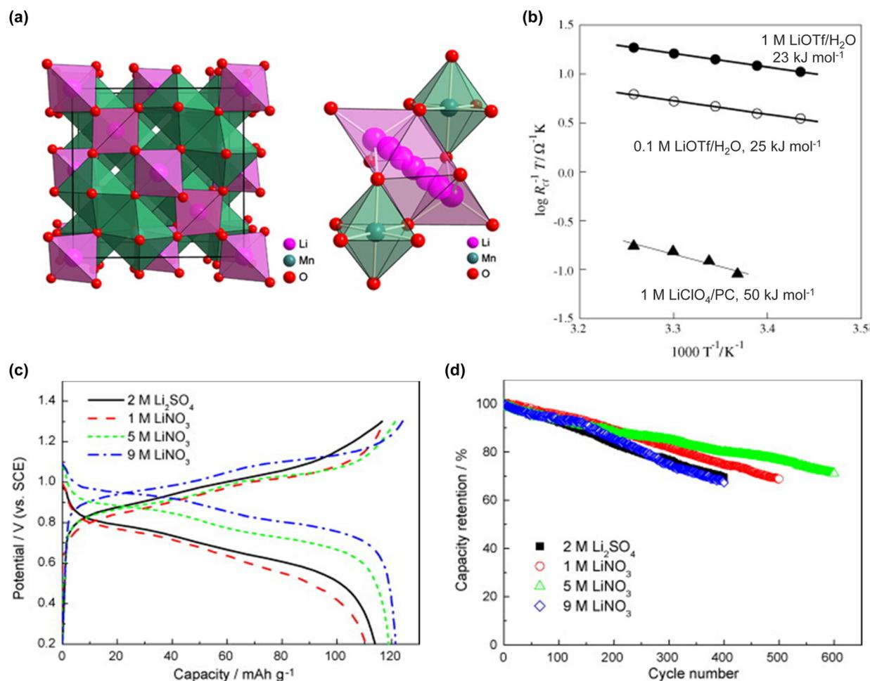
Fig. 21 Crystal structure and  $\text{Li}^+$  diffusion pathway in spinel  $\text{LiMn}_2\text{O}_4$ .<sup>268</sup> (b) Activation energies for interfacial  $\text{Li}^+$  ion transfer reactions,<sup>266</sup> (c) charge/discharge curves, and (d) cycling stability of  $\text{LiMn}_2\text{O}_4$  in the given electrolytes.<sup>267</sup> Reprinted with permission from *Progress in Natural Science: Materials International* (a) and *Journal of Power Sources* (b)–(d).
