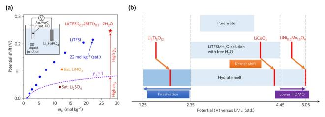
Fig. 34 (a) Electrode potential shift depending on the electrolyte concentration. (b) Relationship between the operating potential windows of aqueous electrolytes and the reaction potentials of electrodes. The upshifted electrode potential in the hydrate melt contributes to mitigating electrolyte reduction on the Li<sub>4</sub>Ti<sub>5</sub>O<sub>12</sub> surface. <sup>19</sup> Reprinted with permission from *Nature Energy*.
