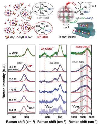
Fig. 61 Construction of a super-saturated ZnSO<sub>4</sub> electrolyte in metalorganic-framework channels, demonstrated by Raman spectroscopy.<sup>735</sup> Reprinted with permission from Angewandte Chemie International Edition.
