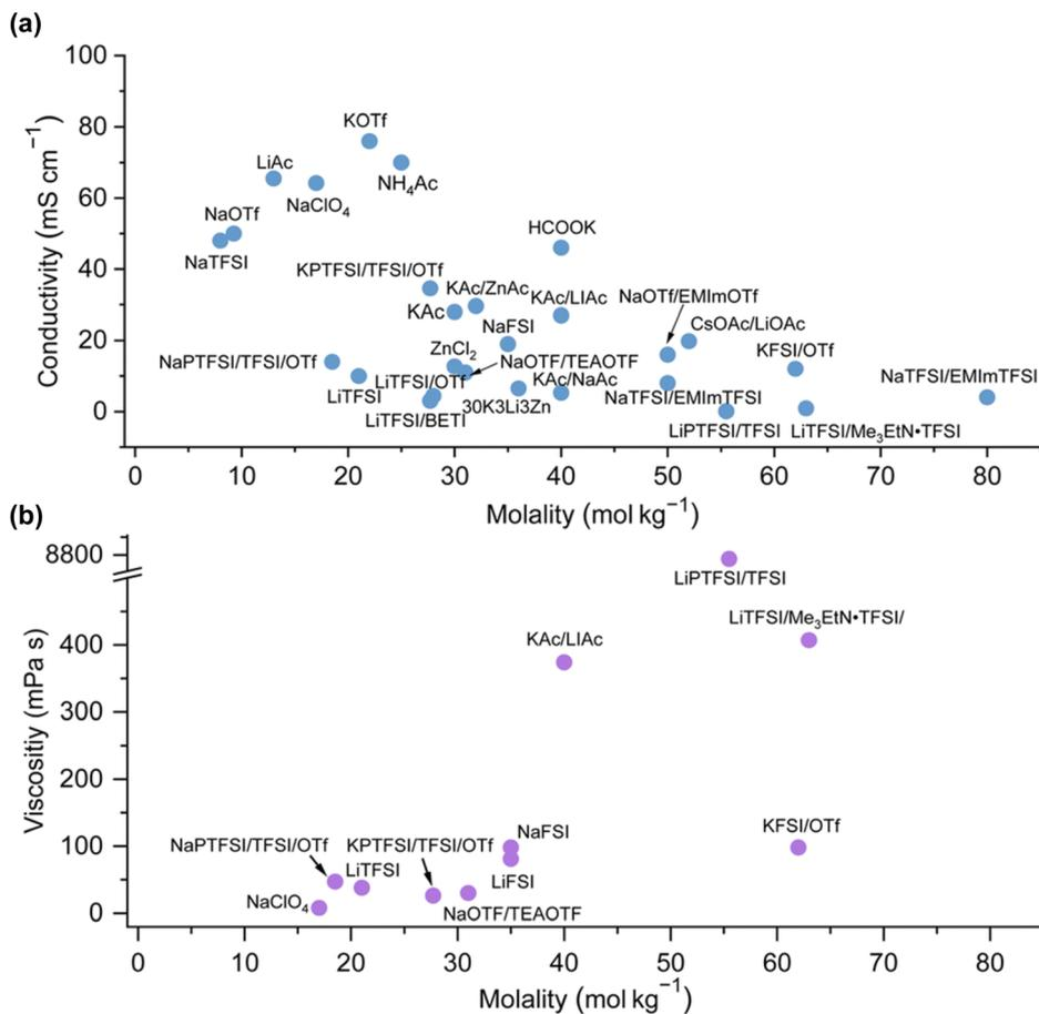
Fig. 17 (a) Ionic conductivity and (b) viscosity of various aqueous electrolytes.<sup>226</sup> Reprinted with permission from *Energy & Environmental Science*.
