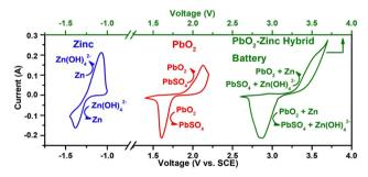
**Fig. 79** Cyclic voltammetry curves of Zn in an alkaline electrolyte (blue),  $PbO_2$  in an acidic electrolyte (red), and a  $PbO_2$ |Zn battery with an electrolyte decoupling system (alkaline anolyte and acidic catholyte) (green) under a scan rate of 10 mV s<sup>-1.867</sup> Reprinted with permission from Angewandte Chemie International Edition.
