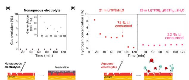
Fig. 32 Estimated gas evolution during exposure of LiF-protected Li metal to (a) nonaqueous and (b) highly salt-concentrated aqueous electrolytes. 333 Reprinted with permission from ACS Energy Letters.
