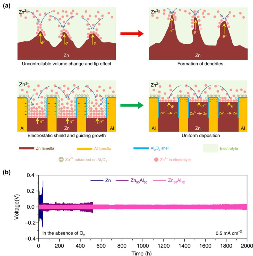
Fig. 60 (a) Schematic of suppressed Zn dendrite growth on lamella-nanostructured eutectic Zn<sub>88</sub>Al<sub>12</sub> alloys. (b) Long-term cycling of symmetric batteries in an O<sub>2</sub>-free aqueous ZnSO<sub>4</sub> solution.<sup>672</sup> Reprinted with permission from *Nature Communications*.
