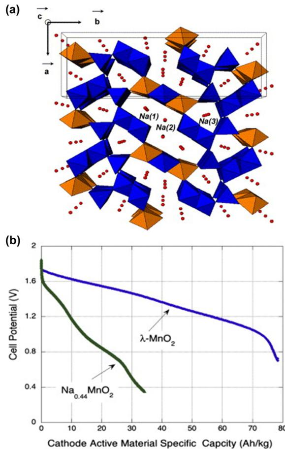
Fig. 27 Crystal structure of  $\text{Na}_{0.44}\text{MnO}_2$ .<sup>311</sup> (b) Galvanostatic discharge curves of  $\text{Na}_{0.44}\text{MnO}_2$  and  $\lambda\text{-MnO}_2$  in 1 M  $\text{Na}_2\text{SO}_4/\text{H}_2\text{O}$ .<sup>312</sup> Reprinted with permission from *Sensors and Actuators B* (a) and *Journal of Power Sources* (b).
