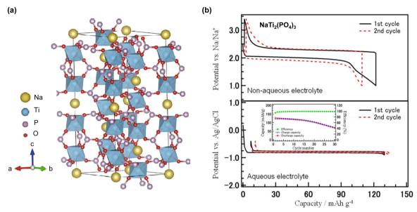
Fig. 29 (a) and (b) Crystal structure and electrochemical properties of NaTi<sub>2</sub>(PO<sub>4</sub>)<sub>3</sub>, <sup>318,319</sup> The sodiation/desodiation curves of NaTi<sub>2</sub>(PO<sub>4</sub>)<sub>3</sub> were obtained in 1 M NaClO<sub>4</sub>/ethylene carbonate: dimethyl carbonate (1:1, v:v) and 2 M Na<sub>2</sub>SO<sub>4</sub>/H<sub>2</sub>O. Reprinted with permission from Nano-micro Letters (a) and Journal of The Electrochemical Society (b).
