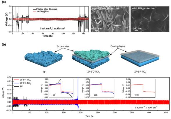
Fig. 59 (a) Performance of Zn|Zn symmetric cells with and without an 8 nm-thick TiO<sub>2</sub> coating on Zn metal.<sup>611</sup> (b) Schematic of Zn plating and Zn|Zn symmetric cell results under different coating conditions. ZF, C-TiO2, and F-TiO2 correspond to Zn foil, commercial TiO2, and highly (001) facet-exposed  $\overline{\text{TiO}}_2$ , respectively. <sup>671</sup> Reprinted with permission from Advanced Materials Interfaces (a) and Nature Communications (b)
