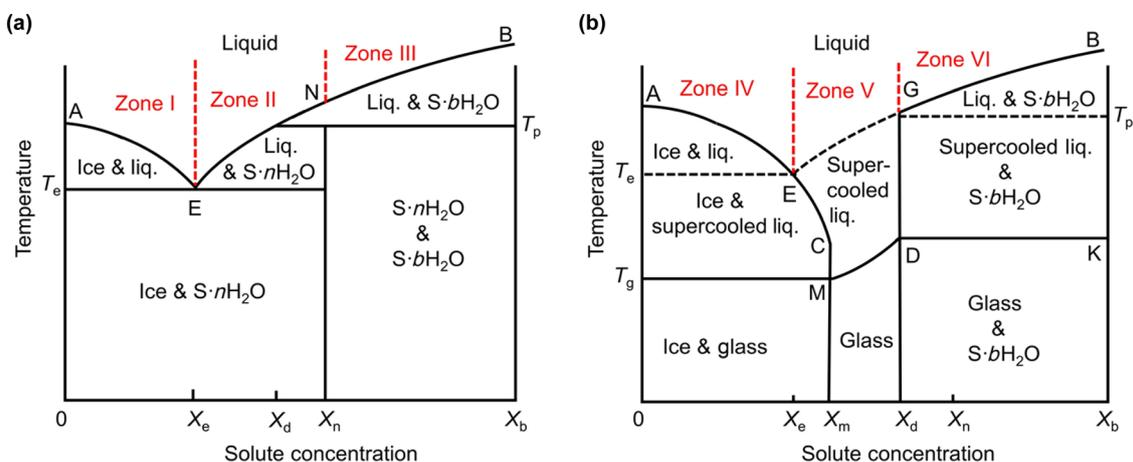
Fig. 18 (a) Equilibrium binary  $\text{H}_2\text{O}$ -salt and (b) non-equilibrium binary  $\text{H}_2\text{O}$ -salt phase diagrams of aqueous solutions.<sup>227</sup> Reprinted with permission from *Nano Research Energy*.
