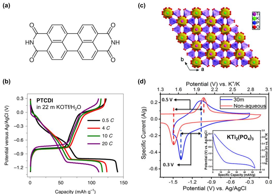
Fig. 31 (a) and (b) Molecular structure and electrochemical properties of PTCDI.<sup>122</sup> (c) and (d) Crystal structure and electrochemical properties of  $\text{KTi}_2(\text{PO}_4)_3$  in 30 m KOAc/ $\text{H}_2\text{O}$ .<sup>188,330</sup> Reprinted with permission from *Nature Energy* (a) and (b), *Chemical Communications* (c) and *ACS Energy Letters* (d).
