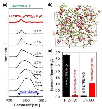
Fig. 12 (a) Raman spectra of LiPTFSI solutions and the monohydrate melt, Li(PTFSI)<sub>0.6</sub>(TFSI)<sub>0.4</sub>·1H<sub>2</sub>O. (b) Solution structure of the monohydrate melt obtained through DFT-MD simulations. (c) Number of hydrogen bonds and coordination to cations around a water molecule in the given electrolytes.85 Reprinted with permission from Electrochemistry Communications.
