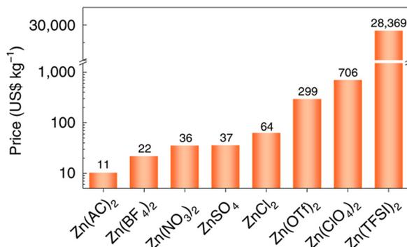
Fig. 53 Cost comparison of various Zn salts.<sup>597,598</sup> Zn(Ac)<sub>2</sub> and Zn(OAc)<sub>2</sub> refer to the same chemical compound, Zn(CH<sub>3</sub>COO)<sub>2</sub>. Reprinted with permission from *Nature Sustainability*.
