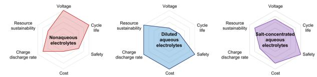
Advantages and limitations of nonaqueous, diluted aqueous, and salt-concentrated aqueous electrolytes.
