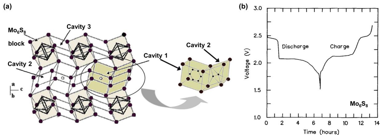
Fig. 25 (a) and (b) Crystal structure and electrochemical properties of  $\text{Mo}_6\text{S}_8$ .<sup>297–299</sup> Reprinted with permission from *Inorganic Chemistry* (a) and *Canadian Journal of Physics* (b).
