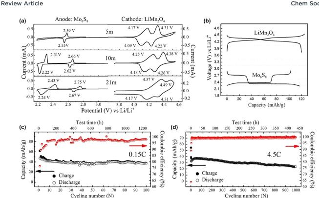
Fig. 6 (a) and (b) Cyclic voltammograms and galvanostatic charge and discharge curves of LiMn<sub>2</sub>O<sub>4</sub> cathode and Mo<sub>6</sub>S<sub>8</sub> anode in LiTFSI/H<sub>2</sub>O with various concentrations. (c) and (d) Electrochemical performance of aqueous  $LiMn_2O_4|Mo_6S_8$  full cells in water-in-salt 21 m  $LiTFSI/H_2O$  electrolyte. <sup>18</sup> Reprinted with permission from Science
