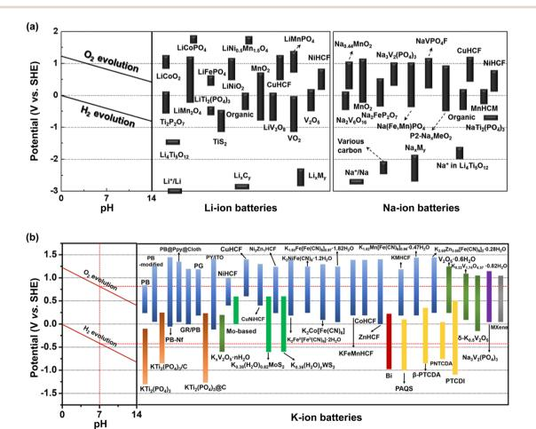
Fig. 20 Thermodynamic potential window of water and redox potentials of cathode and anode active materials for (a) Li-, Na-, and (b) K-ion batteries. 260,261 Reprinted with permission from Chemical Reviews (a) and Energy & Environmental Science (b).
