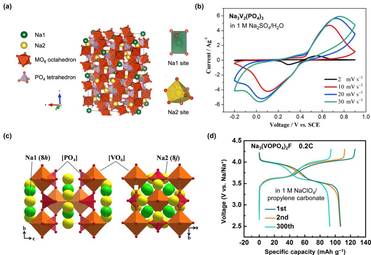
Fig. 28 Crystal structures and electrochemical properties of (a) and (b)  $\text{Na}_3\text{V}_2(\text{PO}_4)_3$ <sup>313,316</sup> and (c) and (d)  $\text{Na}_3(\text{VOPO}_4)_2\text{F}$ .<sup>317</sup> Reprinted with permission from *Electrochemistry* (a), *ChemElectroChem* (b), and *Joule* (c) and (d).
