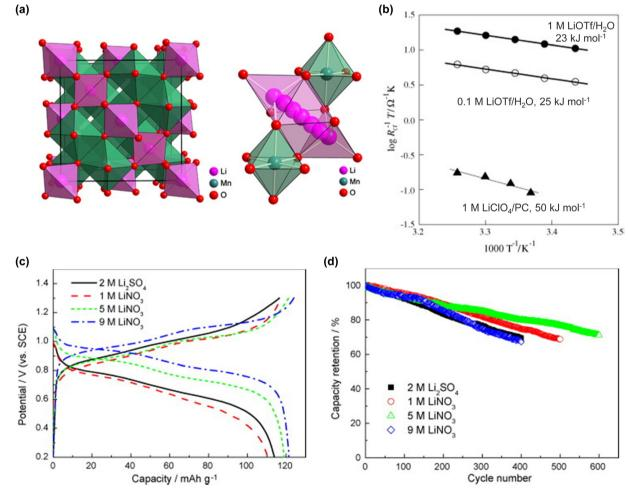
Fig. 21 Crystal structure and Li<sup>+</sup> diffusion pathway in spinel LiMn<sub>2</sub>O<sub>4</sub>.<sup>268</sup> (b) Activation energies for interfacial Li<sup>+</sup> ion transfer reactions,<sup>266</sup> (c) charge/ discharge curves, and (d) cycling stability of LiMn<sub>2</sub>O<sub>4</sub> in the given electrolytes.<sup>267</sup> Reprinted with permission from *Progress in Natural Science: Materials* International (a) and Journal of Power Sources (b)-(d)
