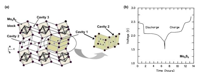
Fig. 25 (a) and (b) Crystal structure and electrochemical properties of Mo<sub>6</sub>S<sub>8</sub>.<sup>297-299</sup> Reprinted with permission from *Inorganic Chemistry* (a) and Canadian Journal of Physics (b).
