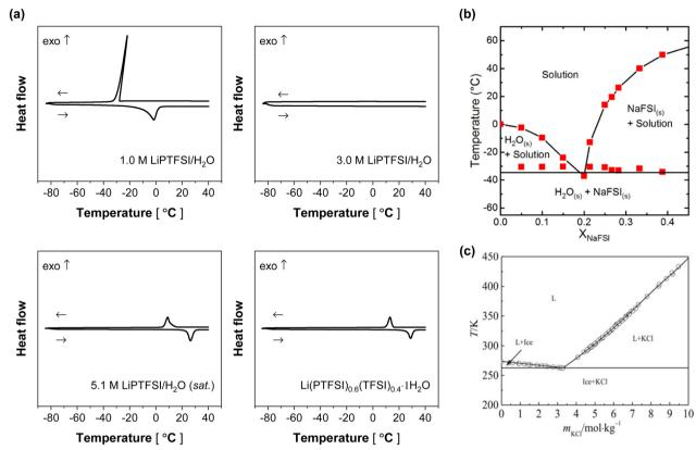
Fig. 19 (a) Thermal stability of LiPTFSI-based aqueous electrolytes evaluated by differential scanning calorimetry at a rate of 5  $^{\circ}$ C min<sup>-1,85</sup> Phase diagrams of (b) NaFSI-H<sub>2</sub>O<sup>89</sup> and (c) KCl-H<sub>2</sub>O binary systems.<sup>231</sup> Reprinted with permission from *Electrochemistry Communications* (a), *ACS Materials Letters* (b), and *Calphad* (c).
