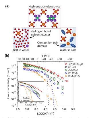
Fig. 50 (a) Illustration of solution structures in different electrolytes: saltin-water, water-in-salt, and high-entropy electrolytes. (b) Ionic conductivity of the Li<sub>2</sub>ZnCl<sub>4</sub>·9H<sub>2</sub>O electrolyte compared with those of different concentrated and diluted aqueous solutions. 586 Reprinted with permission from Nature Sustainability
