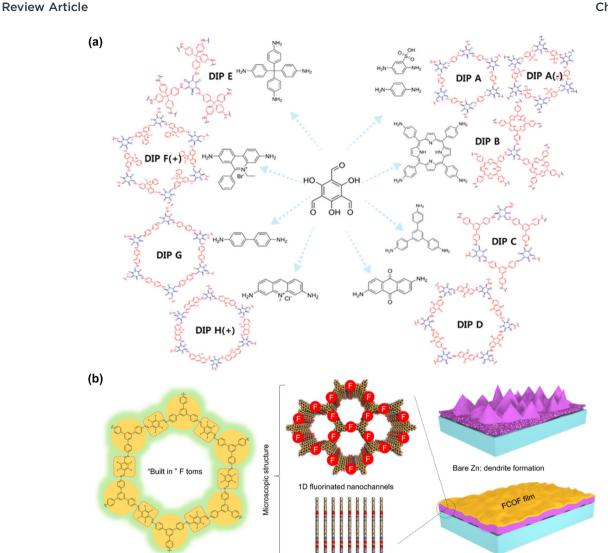
Fig. 62 (a) Structures of diverse covalent organic frameworks (COFs), formed from the 1,3,5-triformylphloroglucinol precursor and various aromatic amine linkers.<sup>740</sup> (b) Suppression of Zn dendrite formation by a fluorinated COFs film.<sup>741</sup> Reprinted with permission from *Advanced Materials* (a) and Nature Communications (b).
