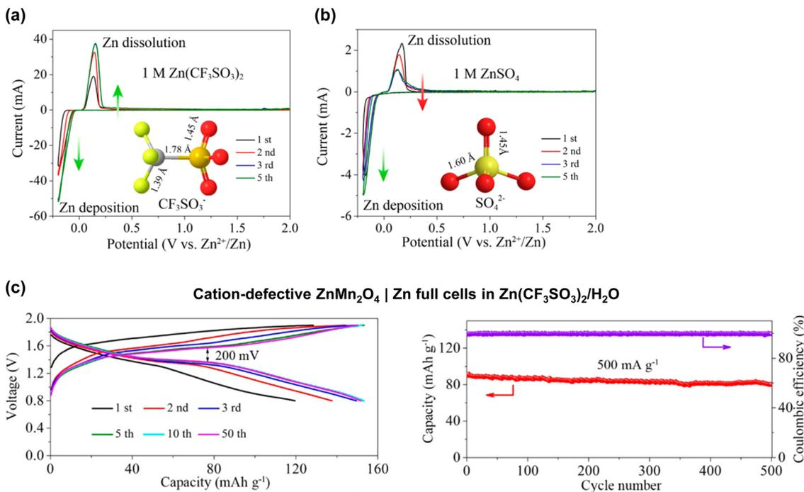
Fig. 52 Cyclic voltammograms of the Zn plating/stripping in (a) 1 M Zn(OTf)<sub>2</sub> and (b) 1 M ZnSO<sub>4</sub> solutions. (c) Galvanostatic charge and discharge curves at 50 mA g<sup>-1</sup> and (d) long-term cycling performance of carbon-coated cation-defective ZnMn<sub>2</sub>O<sub>4</sub>|Zn full cells in 3 M Zn(OTf)<sub>2</sub>/H<sub>2</sub>O at 500 mA g<sup>-1</sup>.<sup>595</sup> Reprinted with permission from *Journal of the American Chemical Society*.
