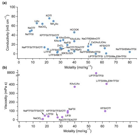
Fig. 17 (a) Ionic conductivity and (b) viscosity of various aqueous electrolytes.<sup>226</sup> Reprinted with permission from Energy & Environmental Science
