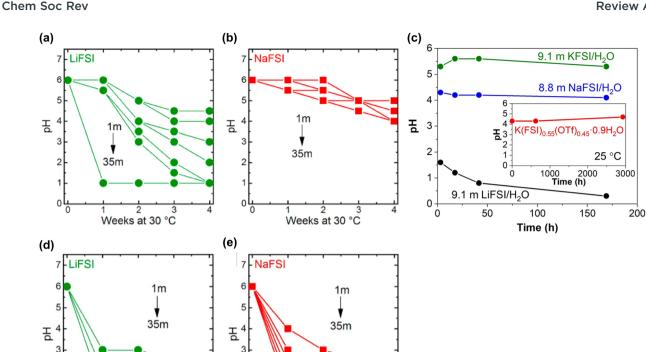
Fig. 39 pH levels of FSI<sup>-</sup> anion-based aqueous electrolytes under various salt concentrations and temperature conditions. 169,170 Reprinted with permission from Electrochimica Acta (a), (b), (d) and (e) and Electrochemistry Communications (c),
