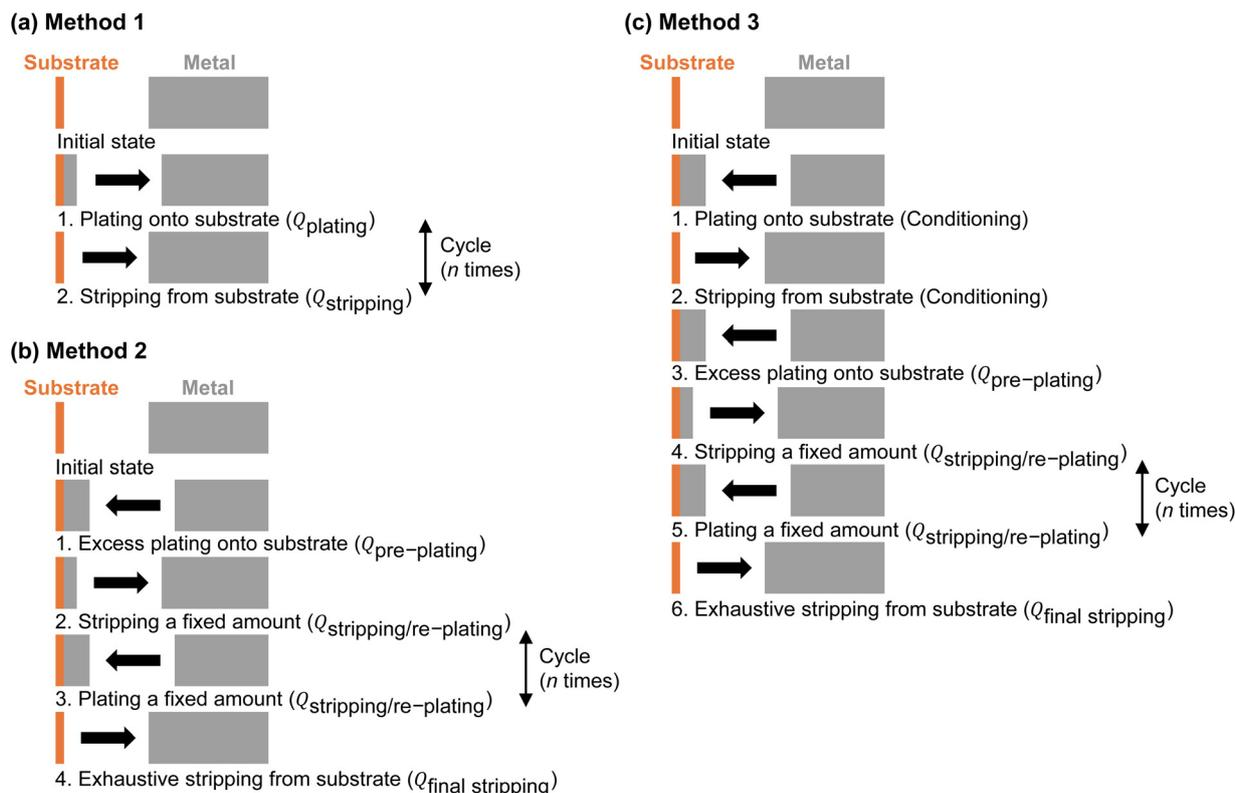
Fig. 68 (a)–(c) Protocols to estimate the Coulombic efficiency of metal plating and stripping.<sup>793</sup> Reprinted with permission from *Advanced Energy Materials*.
