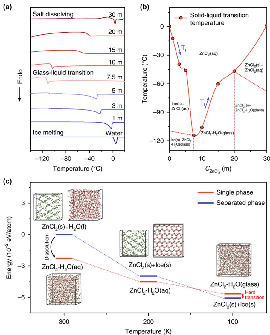
Fig. 49 (a) Differential scanning calorimetry curves and (b) obtained phase transition diagram of a ZnCl<sub>2</sub>/water binary system. (c) Calculated transition state in the transformation from the glass state to the separated crystalline state of a 7.5 m ZnCl<sub>2</sub>/H<sub>2</sub>O solution.<sup>585</sup> Reprinted with permission from *Nature Communications*.
