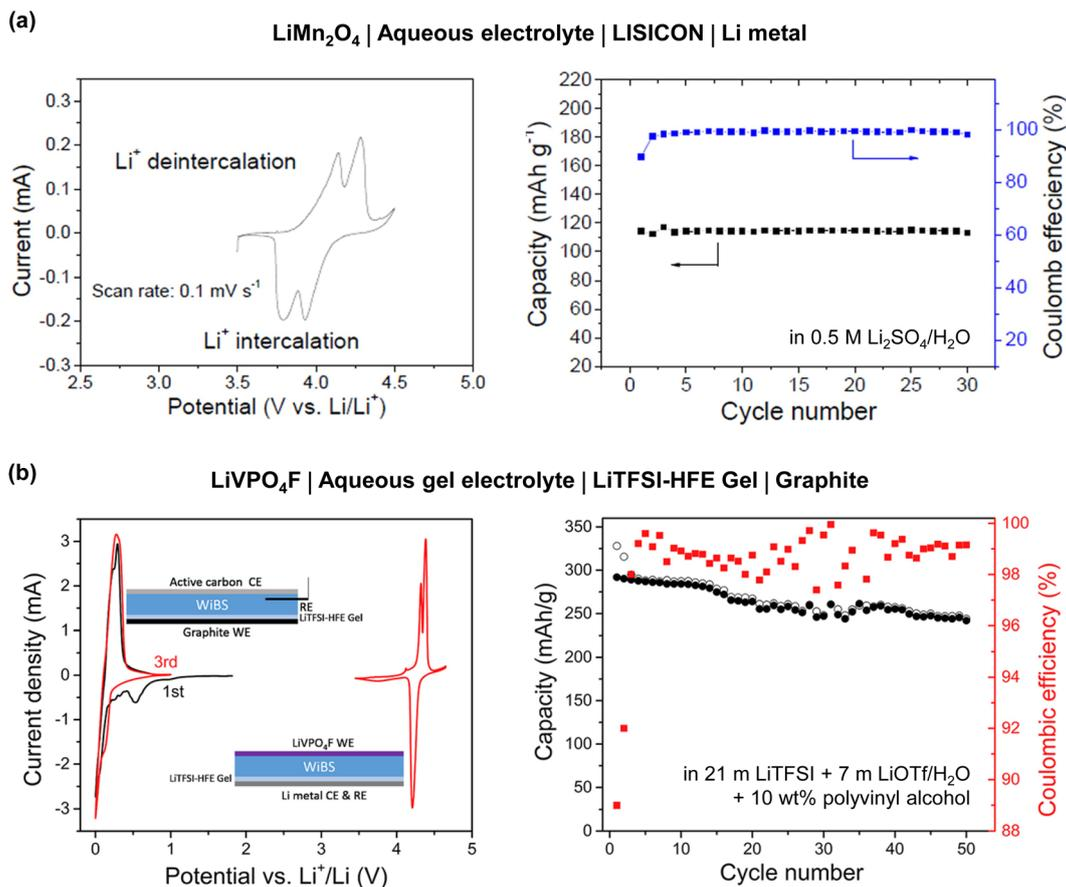
Fig. 33 Electrochemical properties of the (a) LiMn<sub>2</sub>O<sub>4</sub>|LISICON|Li full cell in 0.5 M Li<sub>2</sub>SO<sub>4</sub>/H<sub>2</sub>O<sup>336</sup> and (b) LiVPO<sub>4</sub>F|LiTFSI-HFE gel|graphite full cell in 21 m LiTFSI + 7 m LiOTf/H<sub>2</sub>O + 10 wt% polyvinyl alcohol electrolyte.<sup>337</sup> Reprinted with permission from *Scientific Reports* (a) and *Joule* (b).
