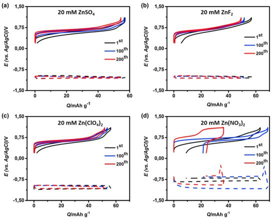
Fig. 51 Potential profiles of the copper hexacyanoferrate cathode (solid line) and Zn-metal anode (dashed line) in (a) 20 mM ZnSO<sub>4</sub>, (b) 20 mM ZnF<sub>2</sub>, (c) 20 mM Zn(ClO<sub>4</sub>)<sub>2</sub>, and (d) 20 mM Zn(NO<sub>3</sub>)<sub>2</sub> solutions.<sup>592</sup> Reprinted with permission from Electrochimica Acta
