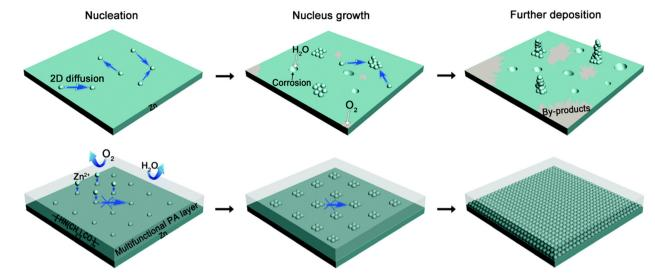
Fig. 63 Mechanism of suppressed Zn dendrite growth with a multifunctional polymeric interphase composed of polyamide and Zn(OTf)<sub>2</sub>. Initial Zn nucleation was delocalized by the introduced polymeric interphase. 752 Reprinted with permission from Energy & Environmental Science.
