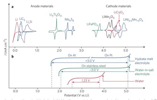
Fig. 5 (a) and (b) Broadened operating potential window in highly salt-concentrated aqueous electrolytes, such as water-in-salt (21 m LiTFSI/H<sub>2</sub>O) and dihydrate melt (28 m Li(TFSI)<sub>0.7</sub>(BETI)<sub>0.3</sub>·2H<sub>2</sub>O), contributing to an increase in output voltage of aqueous batteries.<sup>88</sup> Reprinted with permission from Nature Energy.
