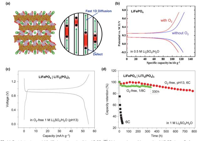
Fig. 23 (a) Crystal structure and Li<sup>+</sup> diffusion pathway in olivine LiFePO<sub>4</sub>.<sup>287</sup> (b) Increased reversible capacity of LiFePO<sub>4</sub> in an O<sub>2</sub>-free aqueous electrolyte. (c) Charge/discharge curves and (d) long-term cycling of aqueous LiFePO<sub>4</sub>|LiTi<sub>2</sub>(PO<sub>4</sub>)<sub>3</sub> full cells under the given conditions. (e) Reprinted with permission from *Nano Letters* (a), *Electrochimica Acta* (b) and *Nature Chemistry* (c) and (d).
