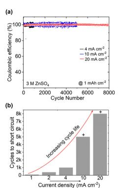
Fig. 71 (a) Coulombic efficiencies of Zn plating and stripping in Ti|3 M ZnSO<sub>4</sub>/H<sub>2</sub>O|Zn cells at various current densities. (b) Chart representation showing a drastic increase in the Coulombic efficiency with increasing current density. 804 Reprinted with permission from ACS Applied Materials & Interfaces
