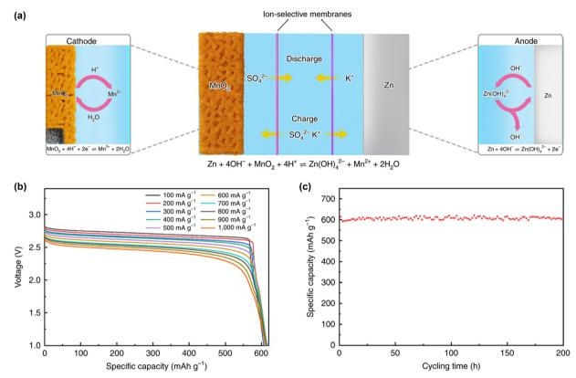
Fig. 78 (a) The working mechanism of an electrolyte-decoupled  $MnO_2|Zn$  battery. (b) and (c) Discharge voltage profiles and long-term cycling stability of the cell. 862 Reprinted with permission from *Nature Energy*.
