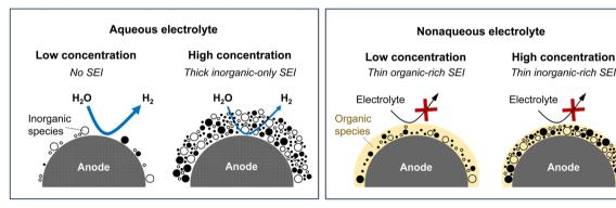
Fig. 40 Schematic comparison of SEI components in aqueous and nonaqueous electrolytes across various salt concentrations.
