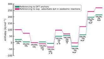
Fig. 18 Enthaloy diagram with enthaloies of formation derived with the standard referencing approach and using the molecular fragment basis set with isodesmic reactions. The enthalpy diagrams are aligned to  $C_2H_6*$  + CO<sub>2</sub>\* to demonstrate that using a molecular fragment basis set changes the adsorption enthalpies and the surface reaction enthalpies.
