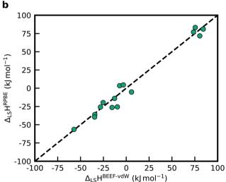
Fig. 6 (a) Comparison of the difference between the enthalpies of formation from the BEEF-vdW and RPBE functional using different sets of references to determine the elemental chemical potentials: least-squares regression,  $CH_4/H_2/H_2O$ , and  $C_2H_6/H_2/CO$ . The mean absolute deviation (MAD) is reported in the legend. (b) Aligning the two DFT datasets for the test case with different xc-functionals using linear regression to determine the elemental chemical potentials
