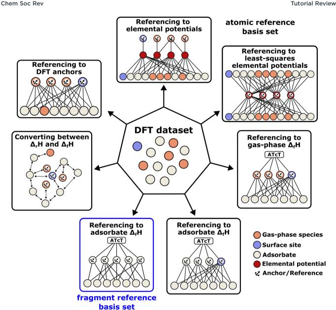
Fig. 4 Overview of the different methods to convert a DFT dataset to enthalpies of formation and construct a global or local thermochemical network. The methods can be grouped into atomic reference basis sets that conserve surface reaction energies from DFT and molecular fragment reference basis sets that exploit error cancellation. The methods can use only DFT energies, apply direct corrections to DFT energies, and consider experimental gasphase species or adsorbate data.
