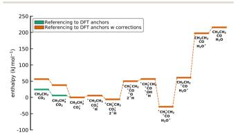
Fig. 8 Enthalpy diagram with the relative enthalpies derived from the corrected DFT energies of  $CO_2$  (+31.8 kJ  $mol^{-1}$ ) and  $H_2$  (+8.7 kJ  $mol^{-1}$ ) using referencing approach compared with the  $\Delta_{\mathsf{A}}H$  from the uncorrected DFT energies. The enthalpy diagrams are aligned to  $C_2H_6^* + CO_2^*$  to demonstrate that the adsorption enthalpy of CO2 was corrected
