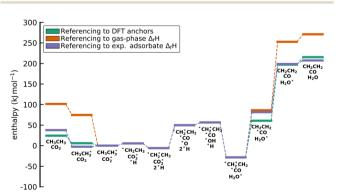
Fig. 11 Enthalpy diagram with the enthalpies of formation derived with the standard referencing approach, using the gas-phase  $\Delta_{\rm f}H$  as references, and using experimental enthalpies of formation of adsorbates as reference. The enthalpy diagrams are aligned to  $C_2H_6^* + CO_2^*$  to demonstrate the changes in the adsorption enthalpies, while all surface reaction enthalpies are conserved.
