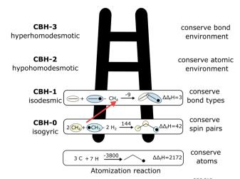
Fig. 15 Types of error cancellation reactions in the CBH $^{209,210}$  scheme to determine the enthalpy of formation of the 1-propyl radical using BEEF-vdW DFT energies. The reported differences in  $\Delta_{\rm f}H$  are with respect to the ATcT value of 118 kJ mol $^{-1}$ . The value above the arrow is the reaction enthalpy and all values are reported in kJ mol $^{-1}$ . The atomization reaction is not part of the CBH method.
