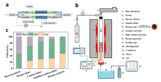
Fig. 8 (a) Non-thermal plasma/catalytic reactor. Reproduced with permission. 63 Copyright 2023, Elsevier. (b) A two-stage fixed bed system for plasmacatalytic pyrolysis. (c) Influence of plasma and catalyst on PP pyrolysis product distribution, gas and oil compositions. (b) and (c) Reproduced with permission.<sup>64</sup> Copyright 2022, Elsevier.
