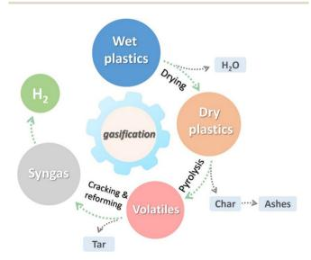
Fig. 10 Main reactions and steps of plastic gasification process.
