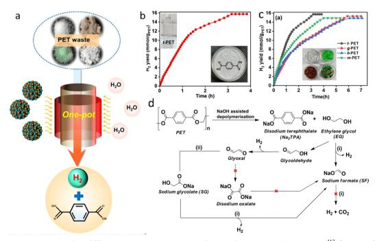
Fig. 12 (a) One-pot H<sub>2</sub> production from PET upcycling by aqueous phase reforming. Reproduced with permission.<sup>112</sup> Copyright 2023, American Chemical Society. (b) Time course plot of H2 yield for the one-pot depolymerization of t-PET. (c) H2 yield for the depolymerization of different plastics. (d) The proposed reaction pathway. (b)-(d) Reproduced with permission. 113 Copyright 2023, Wiley-VCH.
