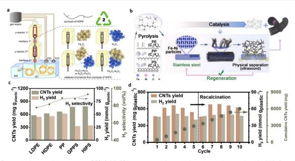
Fig. 4 (a) Schematic diagram of the μ-reactor-GC/MS-FID-TCD system used for pyrolysis and catalytic upgrading of HDPE. Reproduced with permission.<sup>51</sup> Copyright 2023, American Chemical Society. (b)-(d) Pyrolysis-catalysis of waste plastics to H<sub>2</sub> and CNTs using a modified stainlesssteel 316 catalyst. Reproduced with permission.<sup>52</sup> Copyright 2023, Natl Acad Sciences.
