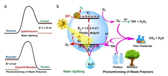
Fig. 13 (a) Endothermic and exothermic water splitting and photoreforming of waste plastics. (b) Mechanistic pathways of waste plastics photoreforming. Reproduced with permission.<sup>31</sup> Copyright 2023, American Chemical Society.
