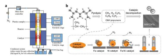
Fig. 3 Schematic depiction of reaction apparatus and processes for conventional pyrolysis-catalytic reforming. (a) A tandem two-stage reactor system. Reproduced with permission. <sup>35</sup> Copyright 2021, Elsevier. (b) Pyrolysis and catalytic decomposition of PP for H<sub>2</sub> and CNTs production with Fe/Ni catalyst. Reproduced with permission.<sup>36</sup> Copyright 2020, Elsevier.
