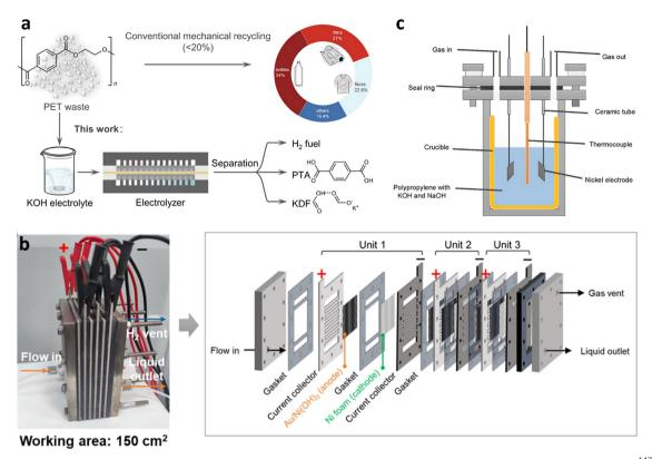
Fig. 15 (a) Conventional and electrocatalytic routes for PET recycling to commodity chemicals and H<sub>2</sub> fuel. Reproduced with permission. 147 Copyright 2021, Springer Nature. (b) Photograph and schematic illustration of the stacked membrane-free flow electrolyzer. Reproduced with permission. 150 Copyright 2023, American Chemical Society. (c) The solar thermo-coupled electrochemical set-up for indoor experiment. Reproduced with permission.<sup>154</sup> Copyright 2020, Elsevier.
