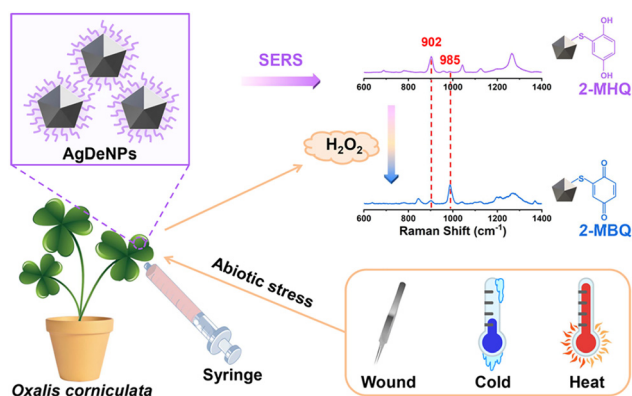
Fig. 44 Schematic illustration of the SERS-based detection of H 2 O 2 by AgDeNPs@MHQ in Oxalis corniculata leaves subjected to abiotic stresses, such as heat and mechanical damage. Figure reproduced with permission from ref. 647.
