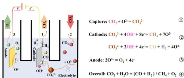
Fig. 16 Schematic illustration of a reactor for reactive  $\text{CO}_2$  capture, featuring a commercial  $\text{CuNi}_{18}$  sheet as the cathode and a corrosion-resistant Ni sheet as the anode in molten  $\text{Li}_{1.427}\text{Na}_{0.359}\text{K}_{0.214}\text{CO}_3 \sim 0.15\text{LiOH}$ . Reproduced with permission from ref. 101.
