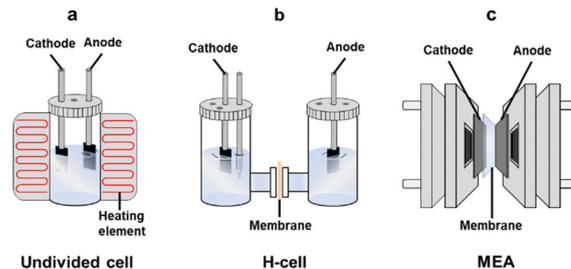
Fig. 7 Three types of reactors used for the electrochemical conversion of captured CO<sub>2</sub>: (a) an undivided cell for molten carbonate electrolysis at high temperatures, (b) an H-cell, and (c) an MEA for electrolysis of aqueous bicarbonate and carbamate solutions at room temperature.
