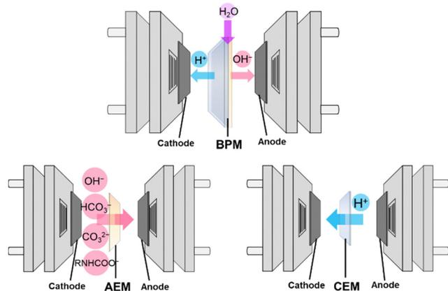
**Fig. 9** Schematic illustration of three typical types of ion exchange membranes used in electrochemical conversion of captured CO<sub>2</sub>.
