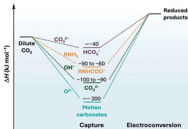
Fig. 3 Schematic representation of the energetics for the electrochemical conversion of captured CO<sub>2</sub>. Enthalpy changes in CO<sub>2</sub> absorption are shown for each capture medium. For ease of representation, energy levels are not to scale.
