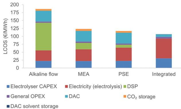
Fig. 17 Comparison of the LCOS of different routes of capture and electrochemical conversion of  $\text{CO}_2$  from air. The terms "alkaline flow," "MEA," and "PSE" (porous solid electrolyte) refer to the independent route using these respective cell configurations. The "General OPEX" category accounts for operational and maintenance costs. Reproduced with permission from ref. 188.
