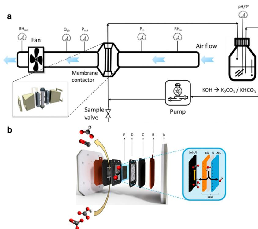
Fig. 12 Integration of atmospheric CO<sub>2</sub> capture and the subsequent electrochemical conversion of the captured CO<sub>2</sub>: (a) diagram of the CO<sub>2</sub> capture setup and (b) the electrolytic cell for converting captured CO<sub>2</sub>. Reproduced with permission from ref. 84.
