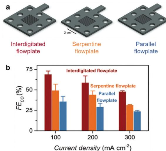
Fig. 11 (a) Interdigitated, serpentine, and parallel cathodic flow plate designs used in bicarbonate electrolysis. (b)  $\text{FE}_{\text{CO}}$  as a function of current density for interdigitated, serpentine, and parallel flow plates tested in a bicarbonate electrolyzer equipped with porous silver electrodes. Reproduced with permission from ref. 79.
