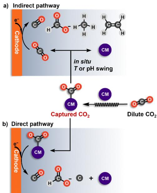
Fig. 4 Illustration of the two pathways of electrochemically reactive  $\text{CO}_2$  capture: (a) Indirect with the captured  $\text{CO}_2$  converted back to  $\text{CO}_2$  at the electrode–electrolyte interface before its electrochemical reduction; (b) direct with the captured  $\text{CO}_2$  as a reactant in the electrochemical step. CM: capture medium.
