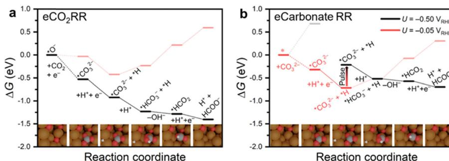
Fig. 6 Energy profiles of (a)  $\text{CO}_2$  reduction by  $\text{CO}_2$  adsorption on an  $^*\text{O}$  site at Cu and further reduction to formate at an applied potential of  $-0.5 \text{ V vs. RHE}$ , and (b)  $\text{CO}_3^{2-}$  reduction to formate at applied potentials of  $-0.05 \text{ V vs. RHE}$  (red),  $-0.50 \text{ V vs. RHE}$  (black), and with the potential pulsed from  $-0.05$  to  $-0.50 \text{ V vs. RHE}$ . Reproduced with permission from ref. 118.
