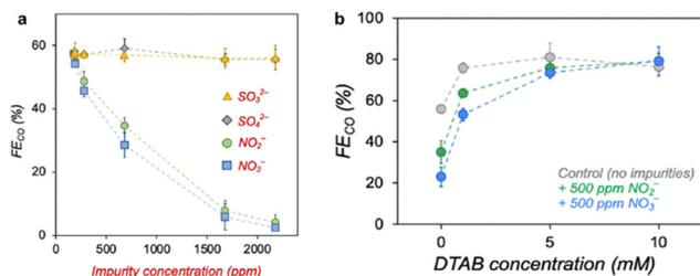
Fig. 14 FE<sub>CO</sub> for electrolysis of 3 M KHCO<sub>3</sub> solution at 100 mA cm<sup>-2</sup> using a porous silver foam cathode with (a) 0–2000 ppm of flue gas impurities and (b) as a function of DTAB concentration. Reproduced with permission from ref. 81.
