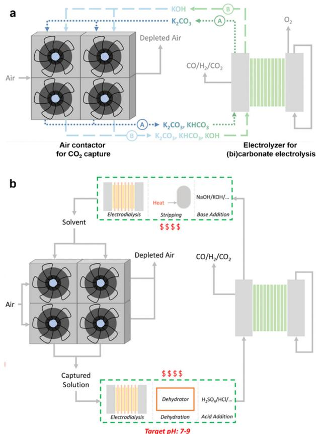
**Fig. 13** Schematic of the integration route proposed in the literature, with the air contactors on the left and the electrolyzer stacks on the right. (a) The two pathways for CO<sub>2</sub> capture from the air are (A) K<sub>2</sub>CO<sub>3</sub>-based and (B) KOH-based. (b) Potential solutions to address the different pH requirements of the capture and conversion processes are shown inside the green dashed boxes at the top and bottom. Reproduced with permission from ref. 168.
