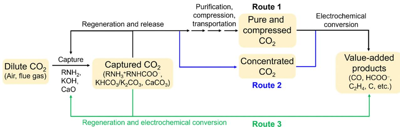
Fig. 1 Three routes for CO<sub>2</sub> capture and electrochemical conversion: (1) independent, (2) coupled, and (3) integrated.
