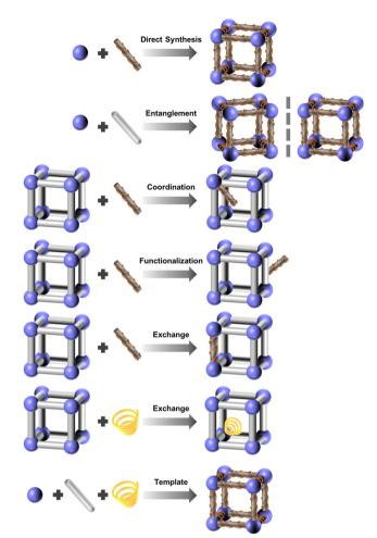
Fig. 12 Classical construction methods for chiral MOFs. The original quests in the framework have been omitted for clarify.
