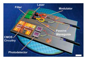
Fig. 61 Overview of plasmonic integrated circuit components featuring high functionality on small wafer footprints. Adapted with permission from ref. 795; Copyright 2012 Springer Nature.
