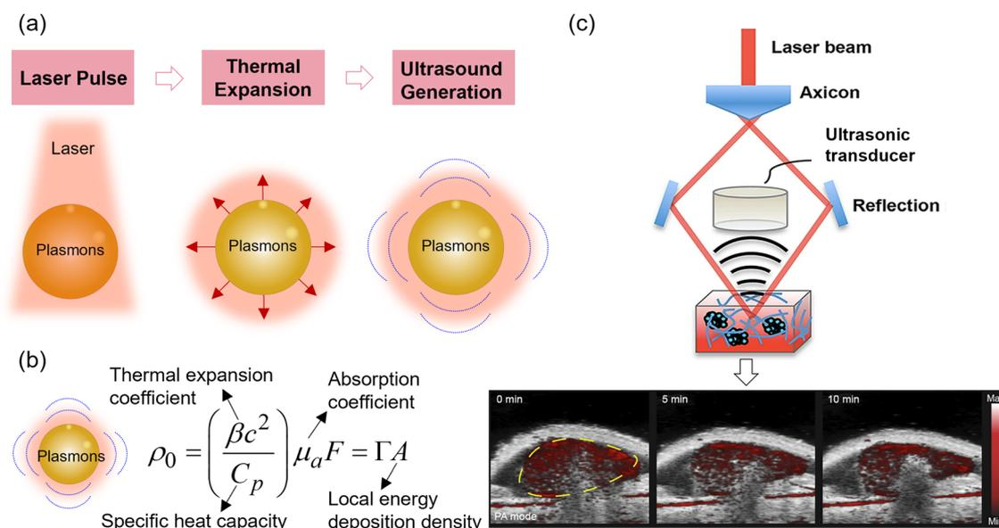
**Fig. 19** Plasmon-enhanced photoacoustic effects in the kHz range. (a) Schematic diagram showing the enhancement of ultrasound generation in photoacoustic effects via the pressure difference induced by plasmon-enhanced thermal expansion. (b) Factors affecting pressure difference ( $\rho_0$ ) in plasmon-enhanced photoacoustic effects. (c) Schematic diagram of the plasmon-enhanced photoacoustic imaging. Adapted with permission from ref. 200; Copyright 2021 American Chemical Society.
