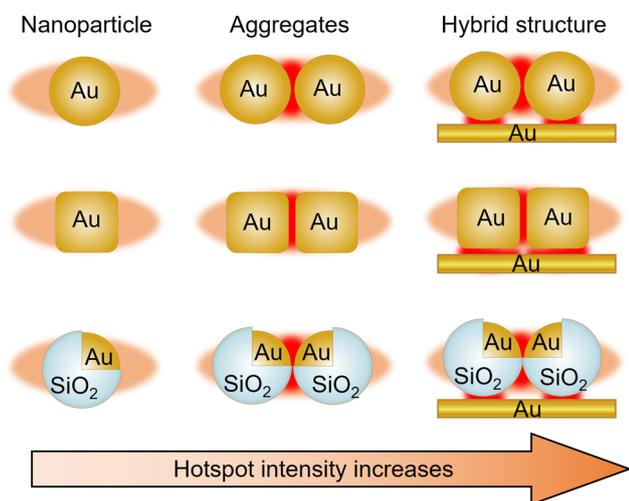
Fig. 25 Schematic diagram of a typical zero-dimensional plasmonic nanostructure.
