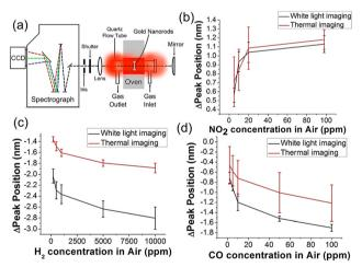
Fig. 54 Thermal energy harvesting with plasmonic-based chemical sensors. (a) Schematic of the thermal imaging setup. Calibration graphs from thermal and white light imaging for (b) NO<sub>2</sub>, (c) H<sub>2</sub> and (d) CO analyte gases in an air background. Adapted with permission from ref. 769; Copyright 2014 American Chemical Society.
