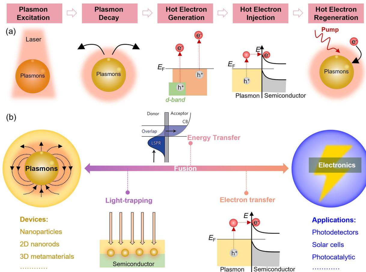
**Fig. 10** Plasmonic fusion with electronics. (a) Schematic view of plasmon generation and decay, hot-electron generation, injection, and regeneration. (b) Plasmonic fusion with electronics *via* light-trapping, electron transfer, and energy transfer.
