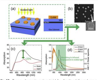
Fig. 57 Copper plasmonic metamaterial for directional thermal energy management. (a) Sketch of the operating structure. (b) SEM images of the fabricated disk. (c) Absorption spectra with front and back incidence after reduction treatment. (d) Simulated absorption spectra with front and back incidence. Adapted with permission from ref. 782; Copyright 2020 Elsevier.
