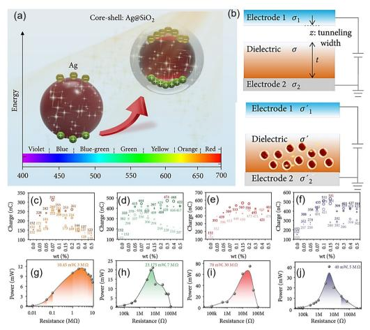
Fig. 59 Surface plasmon effect dominated high-performance TENG. (a) Superiority of Ag@SiO2 NPs in generating the surface plasmon effect. (b) Capacitor model of a TENG, both undoped (upper) and doped with Ag@SiO2 (lower). (c)-(f) Output voltage of Ag, Ag@SiO2-3 nm, Ag@SiO2-6 nm, and Ag@SiO2-12 nm with visible light. (g)-(j) Output power of Ag, Ag@SiO2-3 nm, Ag@SiO2-6 nm, and Ag@SiO2-12 nm with visible light. Adapted with permission from ref. 657; Copyright 2022 AAAS
