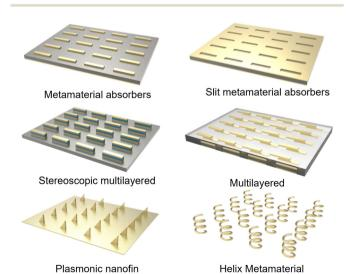
Fig. 28 Schematic diagram of a typical three-dimensional plasmonic
