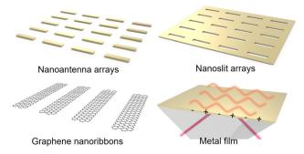
Fig. 27 Schematic diagram of a typical two-dimensional plasmonic nanostructure.
