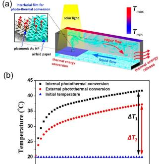
Fig. 53 Efficient solar-thermal energy harvesting via internal plasmonic heating. (a) Schematic of solar-thermal energy harvest driven by interfacial plasmonic heating. (b) Temperature progression profiles for solar water heating systems, comparing conventional and new solar-thermal designs. Adapted with permission from ref. 766; Copyright 2016 American Chemical Society
