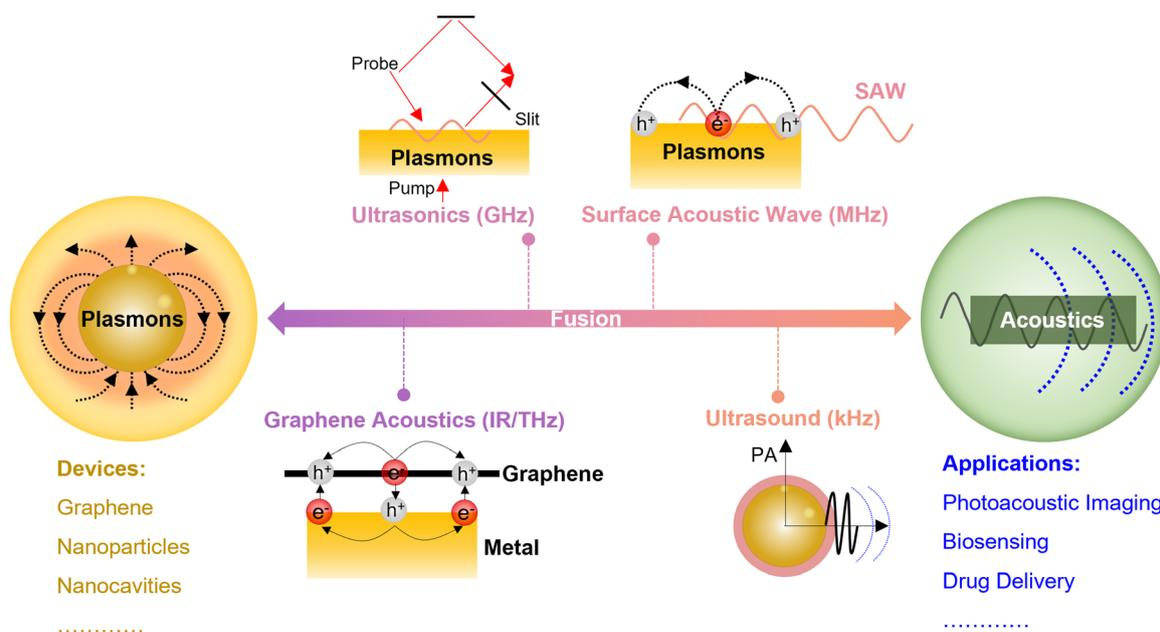
Fig. 18 Plasmonic fusion with acoustics. The combination of plasmon and acoustic devices includes ultrasound in the kHz region, SAWs in the MHz region, ultrasounds in the GHz region, and graphene acoustics in the IR/THz region.
