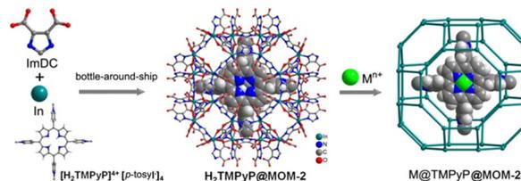
Fig. 4 View of the bottle-around-ship synthesis of H<sub>2</sub>TMPyP@MOM-2 *via* the encapsulation of H<sub>2</sub>TMPyP porphyrin cation in the anionic MOF named MOM-2, and the synthesis of M@TMPyP@MOM-2 *via* post-synthetic metalation. Adapted from ref. 44 with permission of the American Chemical Society, Copyright 2008.
