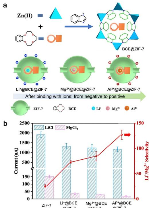
Fig. 7 Preparation of  $\text{M@BCE@ZIF-7}$  ( $\text{M} = \text{Li}^+, \text{Mg}^{2+}, \text{Al}^{3+}$ ) with a change of channel charges from negative to positive. (b) Current values across various membranes and the corresponding  $\text{Li}^+/\text{Mg}^{2+}$  selectivity. Reproduced from ref. 59 with permission of Wiley-VCH Verlag GmbH & Co, Copyright 2023.
