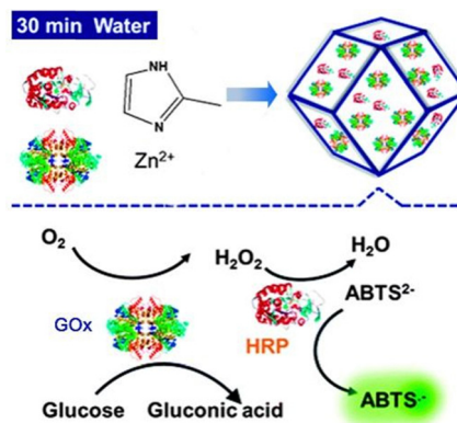
Fig. 24 GOx and HRP-contained ZIF-8 that performed the oxidation of glucose and electron transport to water. Reproduced from ref. 107 with permission of the Royal Society of Chemistry, Copyright 2015.
