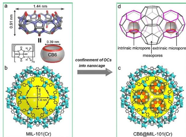
**Fig. 12** Illustration of the impregnation synthesis of CB6@MIL-101 materials. Views of (a) CB6 molecule; (b) mesoporous cage with hexagonal windows in MIL-101; (c) CB6s in the larger cage of MIL-101; (d) CB6 being selectively doped into the larger cages in MIL-101 while leaving the smaller cages empty. Adapted from ref. 25 with permission of Wiley-VCH Verlag GmbH & Co., Copyright 2020.
