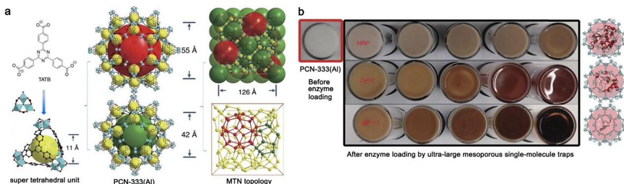
Fig. 16 (a) Structure illustrations of PCN-333(Al); (b) Color variations of PCN-333(Al) when loaded with enzymes (top-down: HRP, Cyt *c*, MP-11) in the mesoporous cages as single-molecule traps at different concentrations. Reproduced from ref. 79 with permission of Nature Publishing Group, Copyright 2015.
