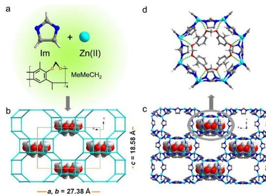
Fig. 10 The synthesis and structural features of MeMeCH<sub>2</sub>@*mer*-ZIF-10. (a) Imidazolate, zinc ion, and MeMeCH<sub>2</sub> as precursors of materials. (b) Wireframe and (c) ball-and-stick view of the *mer*-ZIF-10 framework, occupied by cavitands. (d) Top view of MeMeCH<sub>2</sub> situated in the double-eight ring of *mer*-ZIF-10. Adapted from ref. 65 with permission of the American Chemical Society, Copyright 2014.
