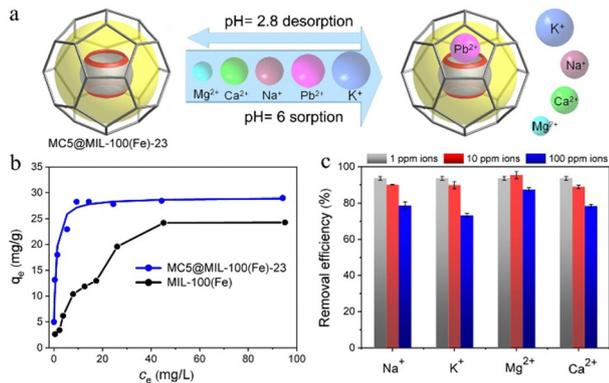
Fig. 21 (a) Schematic view of selective capture of  $\text{Pb}^{2+}$  by  $\text{MC5@MIL-100(Fe)-23}$  among other mineral cations in water. (b)  $\text{Pb}^{2+}$  adsorption isotherms by  $\text{MC5@MIL-100(Fe)-23}$  and  $\text{MIL-100(Fe)}$ . (c) The effects of coexisting ions on the removal efficiency of  $\text{Pb}^{2+}$  at  $1 \text{ mg L}^{-1}$  (1 ppm) by  $\text{MC5@MIL-100(Fe)-23}$ . Reprinted from ref. 39 with permission of Wiley-VCH Verlag GmbH & Co., Copyright 2021.
