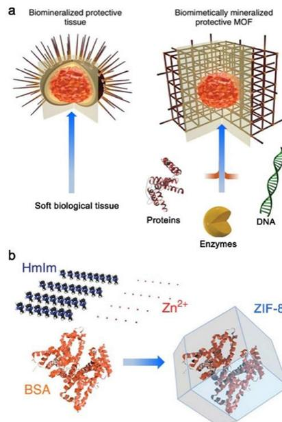
Fig. 19 (a) Schematic view of a hard porous protective shell of a sea urchin that is biomimetalized by soft biological tissue and the biomimetically mineralized MOFs; (b) *in situ* encapsulation of the BSA within ZIF-8 via biomimetalization processes. Reprinted from ref. 89 with permission of Nature Publishing Group, copyright 2015.
