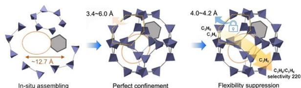
Fig. 9 Schematic view of perfect confinement of B15C5 within ZIF-8 nanocages for the suppression of framework flexibility, thus enhancing  $C_3H_6/C_3H_8$  separation. Adapted from ref. 61 with permission of Wiley-VCH Verlag GmbH & Co, Copyright 2024.
