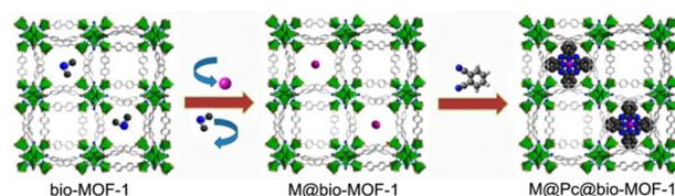
Fig. 6 Schematic presentation of ship-in-bottle synthesis of M@Pc@bio-MOF-1 (M = Co<sup>2+</sup>, Ni<sup>2+</sup>, Cu<sup>2+</sup>). Reprinted from ref. 55 with permission of the American Chemical Society, Copyright 2014.
