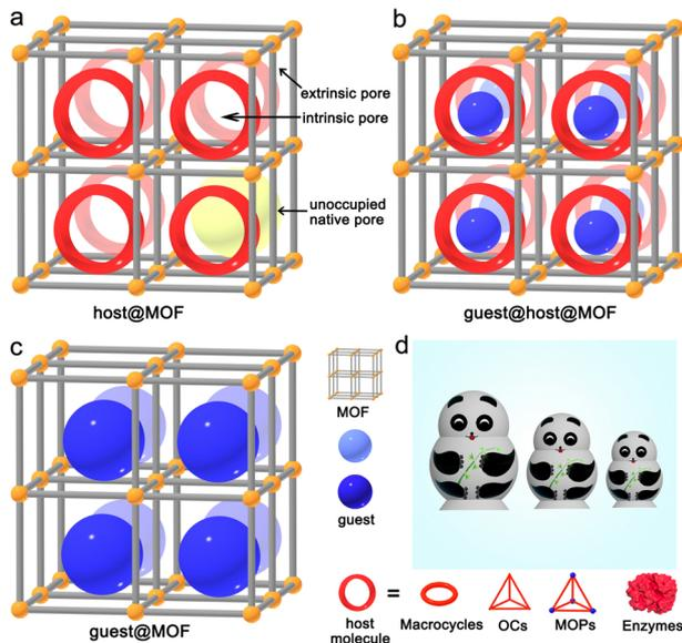
**Fig. 1** Schematic views of (a) host@MOF materials composed of MOFs as the host matrix and encapsulated host molecules such as macrocycles, organic cages (OCs), metal–organic polyhedrons (MOPs) or enzymes; (b) guest@host@MOF materials and (c) traditional guest@MOF materials. (d) Russian (Matryoshka) dolls to symbolize guest@host@MOF materials.
