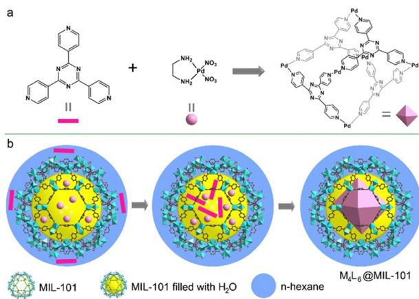
Fig. 14 (a) Schematic preparation of  $M_6L_4$  cages, and (b) the “ship-in-bottle” synthesis of  $M_6L_4$ @MIL-101(Cr). Reproduced from ref. 34 with permission of the American Chemical Society, Copyright 2016.
