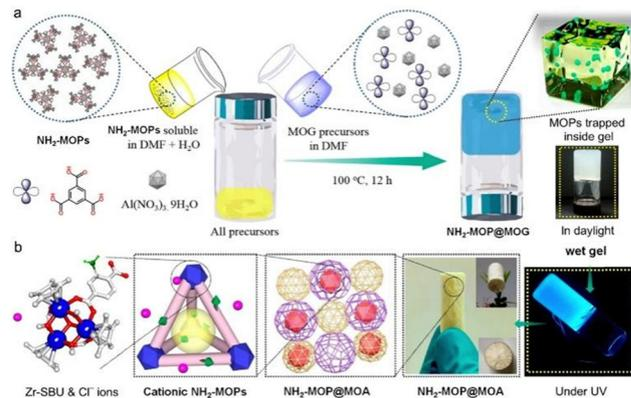
Fig. 15 (a) Schematic preparation of the cationic  $NH_2$ -MOP@MOG composite material *via* the “bottle-around-ship” synthesis; the wet-gel composite in daylight. (b) From left to right: Illustration of the Zr-SBU; surrounding free  $Cl^-$  ions of  $NH_2$ -MOP;  $NH_2$ -MOP@MOA; the lightweight composite aerogel form of  $NH_2$ -MOP@MOA; the wet-gel composite is luminescent. Adapted from ref. 74 with permission of Wiley-VCH Verlag GmbH & Co., Copyright 2022.
