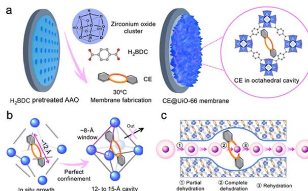
Fig. 8 (a) Fabrication of CE@UiO-66 membranes, such as DB15C5@UiO-66 and DB18C6@UiO-66. (b) Perfect confinement of CE ( $\sim 12$  Å) in the UiO-66 cage. (c) Size and interaction sieving of monovalent ions in CE@UiO-66 membranes. Adapted from ref. 60 with permission of the American Association for the Advancement of Science, Copyright 2024.
