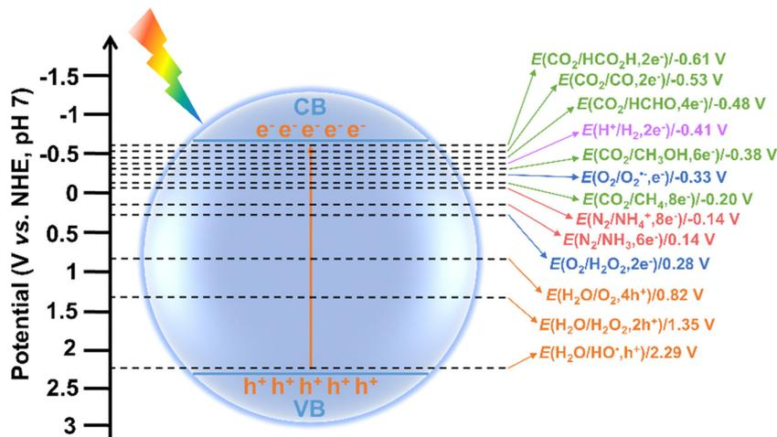
Fig. 3 Redox potentials of different species in photocatalysis.
