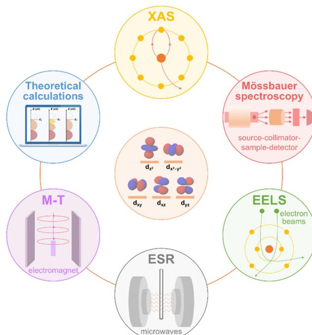
Fig. 5 Techniques for studying electron spin state.
