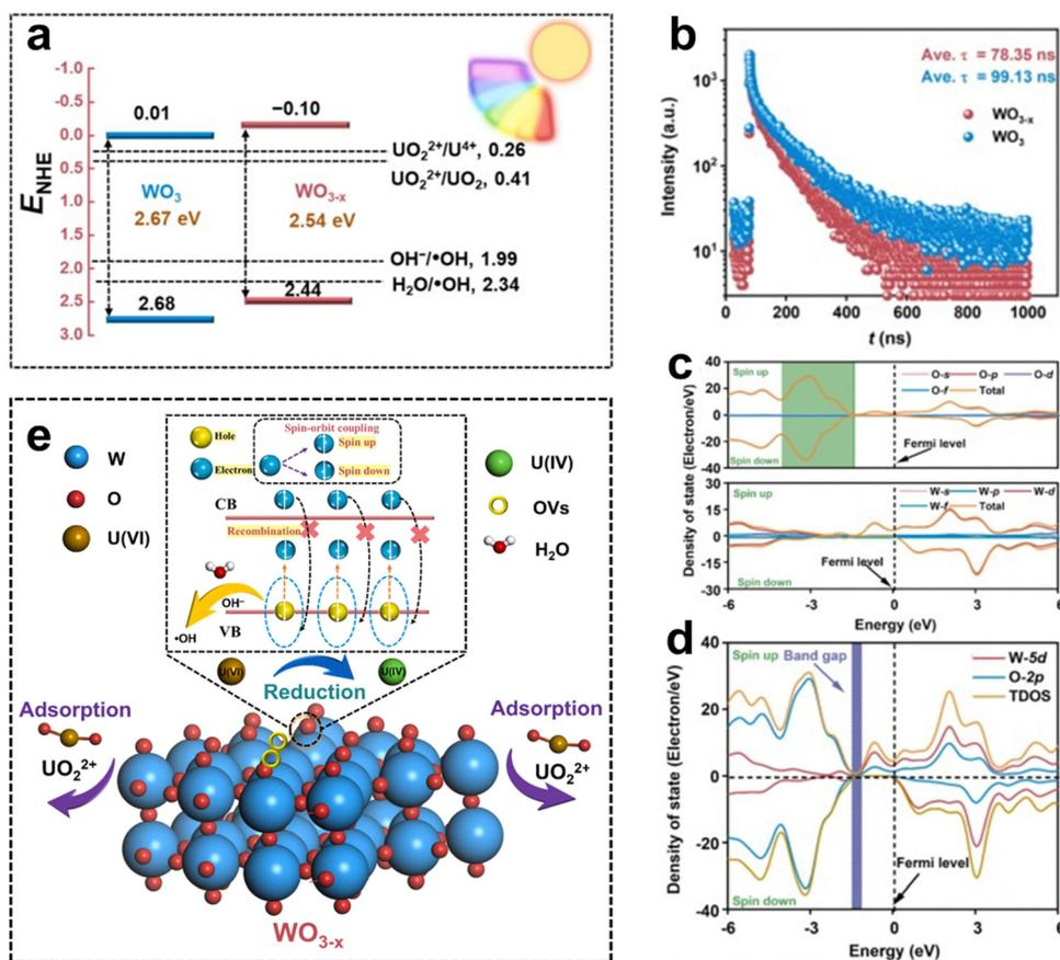
Fig. 14 O defect-induced spin polarization in  $\text{WO}_{3-x}$  for photocatalytic reduction and immobilization of  $\text{U}(\text{VI})$ . (a) Band structures and (b) TRPL spectra of  $\text{WO}_{3-x}$  and  $\text{WO}_3$ . (c) PDOS and (d) DOS spectra of  $\text{WO}_{3-x}$ . (e) The schematic diagram on removal of  $\text{U}(\text{VI})$  by  $\text{WO}_{3-x}$  through adsorption and photocatalytic reduction. Reproduced with permission from ref. 112. Copyright 2023 Elsevier.
