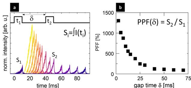
Fig. 19 Complex nature of luminescence originating from the multiple level and multiple dopant interactions in PA mode, where ESA absorption depends on the residual population of the looping level ( $n_2$ ), and thus, two subsequent excitation pulses (a) induce a pulse-gap dependent emission and the so-called (b) paired-pulse signal facilitation (PPF).<sup>13</sup> Adapted with permission from.<sup>13</sup> Copyright 2023, John Wiley and Sons (<https://creativecommons.org/licenses/by/4.0/>).
