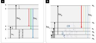
Fig. 22 MIR photon counting (a) five-level quantum counter scheme  $(hv_p - pump, hv_s - signal, hv_f - fluorescence.$  Wavy arrows indicate non-radiative transitions). 145 (b) IR detection scheme based on Pr3+ 245 Dashed arrows are possible cross relaxations (CR) responsible for photon avalanche phenomenon. Transparent lines are additional possible CR and fluorescence transitions not shown in ref. 245
