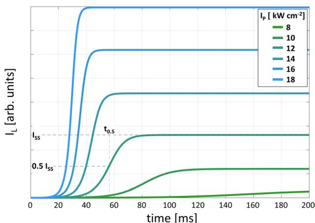
Fig. 4 DRE-simulated kinetic profiles of luminescence intensity rise for different excitation intensities. The 50% rise time ( $t_{0.5}$ ) is shown as the time at which the intensity reaches half of the steady state intensity ( $I_{\text{SS}}$ ).
