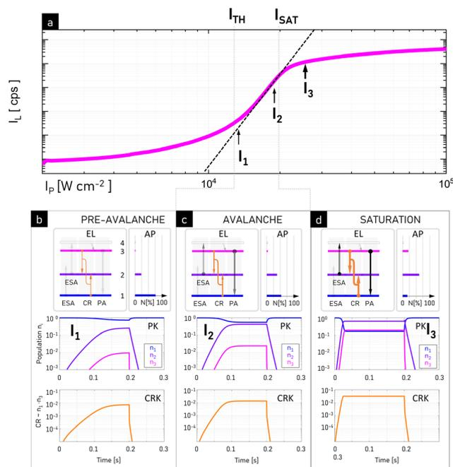
**Fig. 6** Pump power-dependent PA luminescence intensity and population dynamics. (a) Typical S-shape relationship between pump ( $I_p$ ) and luminescence ( $I_l$ ) intensities. (b)–(d) Simulated kinetics of the population of ground ( $n_1$ ), intermediate ( $n_2$ ) and emitting ( $n_3$ ) levels as well as cross-relaxation strength  $CR \cdot n_1 \cdot n_2$  in pre-avalanche (b), avalanche (c) and saturation (d) regions.
