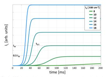
**Fig. 4** DRE-simulated kinetic profiles of luminescence intensity rise for different excitation intensities. The 50% rise time ( $t_{0.5}$ ) is shown as the time at which the intensity reaches half of the steady state intensity ( $l_{SS}$ ).
