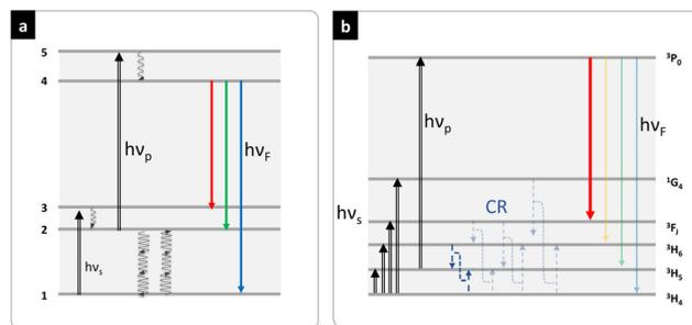
Fig. 22 MIR photon counting (a) five-level quantum counter scheme ( $h\nu_p$  – pump,  $h\nu_s$  – signal,  $h\nu_f$  – fluorescence. Wavy arrows indicate non-radiative transitions).<sup>145</sup> (b) IR detection scheme based on  $\text{Pr}^{3+}$ .<sup>245</sup> Dashed arrows are possible cross relaxations (CR) responsible for photon avalanche phenomenon. Transparent lines are additional possible CR and fluorescence transitions not shown in ref. 245.
