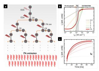
Fig. 1 'Chain reaction' mechanism of PA emission (a) and basic features of PA emission - pump power-dependent PA luminescence intensity (b) compared to linear (N = 1) and nonlinear (N = 2, 3, 4, 5) luminescence behaviour, as well as PA luminescence rise times upon switching on photoexcitation (c); curves in (c) correspond to circles in (b) of the respective shade of red colour.
