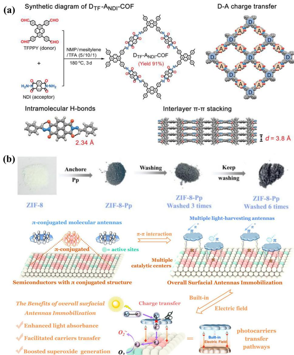
**Fig. 6** (a) Preparation route of the novel COF and its structural features. ((a) Reproduced from ref. 78 with permission from Wiley-VCH, Copyright 2023). (b) Physical roadmap for the preparation of ZIF-8-Pp and the schematic of the large-scale and extensive built-in electric field that will be formed between the two through  $\pi$ - $\pi$  interaction and the corresponding effect manifestation. ((b) Reproduced from ref. 79 with permission from the American Chemistry Society, Copyright 2022).
