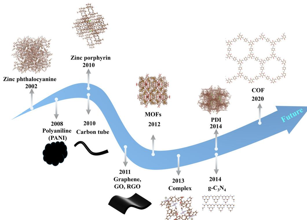
Fig. 4 Development history of materials with  $\pi$ - $\pi$  interactions used in photocatalysis.
