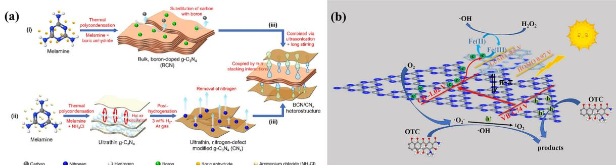
Fig. 9 (a) Preparation route of BCN/ $\text{CN}_x$  hybrid materials ((a) Reproduced from ref. 32 with permission from Elsevier, Copyright 2023). (b) Illustration of the photo-Fenton reaction mechanism of FePc/ $g\text{-C}_3\text{N}_4$  composites. ((b) Reproduced from ref. 171 with permission from Elsevier, Copyright 2023).
