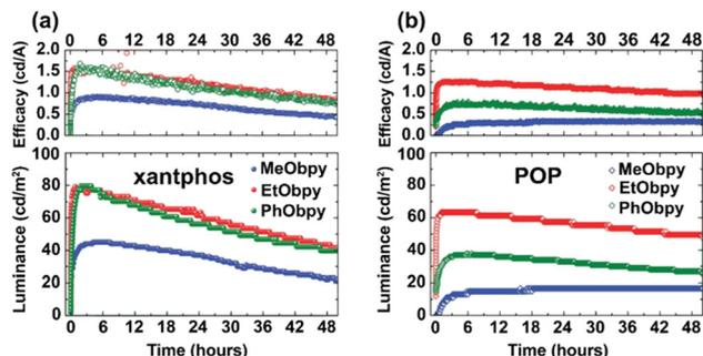
Fig. 37 Efficacy (top) and luminance (bottom) versus time for LECs employing Cu(I) complexes with RObpy and either (a) xantphos or (b) POP ligands. LECs were driven at an average current density of 50 A m<sup>-2</sup>. Reproduced from ref. 340. Copyright 2018, Royal Society of Chemistry.
