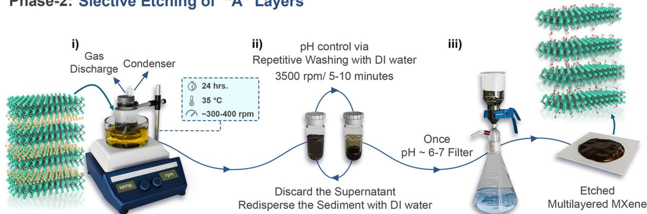
**Scheme 3** (i) Laboratory settings typically followed for etching (ii) washing procedure for pH control. (iii) Depiction of the filtration assembly and as-etched MXene cake obtained after filtration. Note: this method is universal for almost all MAX phases etched via the wet-chemical route.
