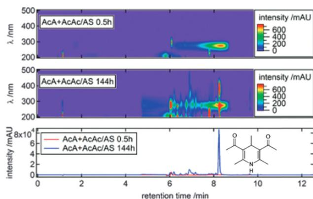
**Fig. 16** HPLC-PDA heatmaps for acetaldehyde + acetylacetone/ammonium sulfate at 0.5 h (top) and 144 h (middle) of reaction time. PDA chromatograms integrated over the 300–500 nm wavelength range retrieved from the two above records. The assigned structure of BrC species eluted at 8.3 min is shown in bottom panel, representing the neutral formula,  $C_{12}H_{17}O_2N$ . Reproduced from ref. 53 with permission from the Royal Chemical Society, copyright 2016.
