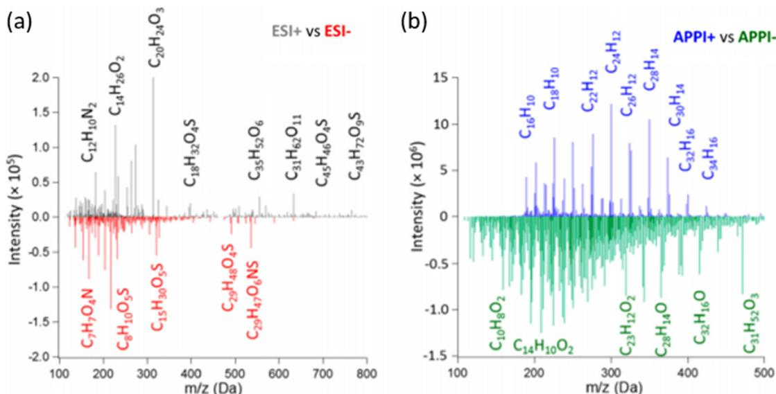
Fig. 3 HRMS detection of solvent-extractable BBOA components assisted with electrospray ionization (ESI) and dopant assisted atmospheric pressure ionization (APPI), with spectra recorded in positive (+) and negative (–) polarities, respectively. Molecular formulas correspond to neutral molecules. Peak intensities are plotted as positive and negative features reflecting polarity of the detected ions. Reproduced from ref. 59 with permission from the American Chemical Society, copyright 2018.
