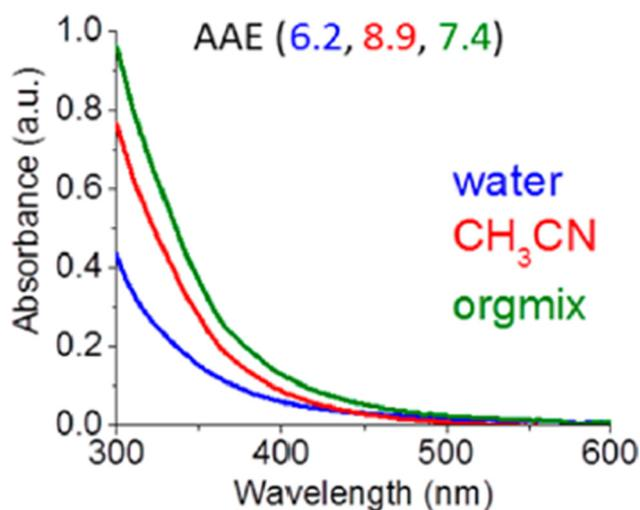
Fig. 1 UV-Vis spectra BrC solutions extracted with different solvents for the same BBOA sample. The amount of extracted BrC generally follows the trend: 'orgmix' > single polar solvent (acetonitrile, methanol) > water. Accordingly, the Absorption Ångström Exponent (AAE) values measured for BrC extracts tend to increase with higher extraction efficiency. Reproduced from ref. 58 with permission from the American Chemical Society, copyright 2017.
