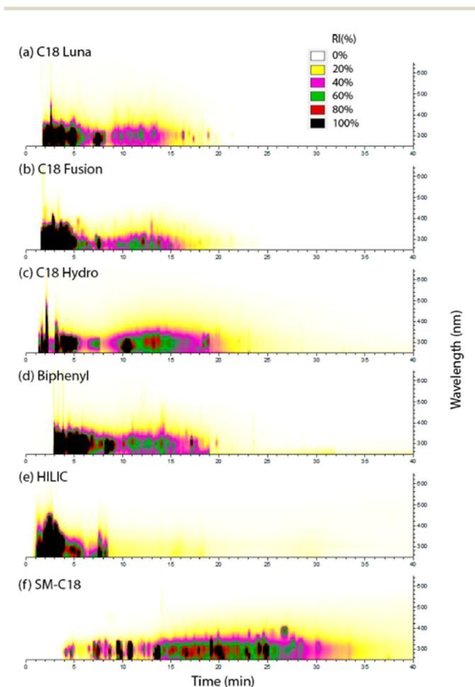
Fig. 2 HPLC–PDA chromatograms of laboratory generated BrC species formed by the aqueous-phase reactions of methylglyoxal (MG) and ammonium sulfate (AS), separated on six HPLC columns. Reproduced from ref. 52 with permission from the American Chemical Society, copyright 2016.
