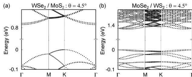
Fig. 5 Tight-binding band structure of twisted heterobilayer TMDs for (a) twisted bilayer WSe<sub>2</sub> / MoS<sub>2</sub> and (b) MoSe<sub>2</sub> / WS<sub>2</sub> heterostructure at twist angle  $\theta = 4.5^\circ$ .<sup>146</sup> Adapted under the terms of the CC BY license from ref. 146 Copyright (2021) IOP Publishing.
