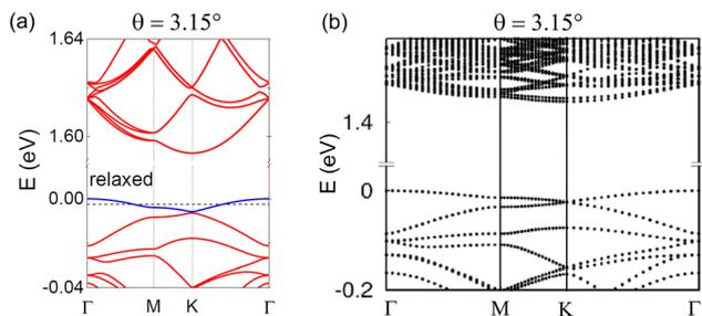
Fig. 4 Tight-binding band structure of twisted homobilayer MoS<sub>2</sub> at  $\theta = 3.15^\circ$ . (a) Bands obtained from a TB model from ref. 173 and 148. Adapted with permission from ref. 148. Copyright (2022) by the American Physical Society. (b) Bands calculated from the TB model from ref. 146. Adapted under the terms of the CC BY license from ref. 146. Copyright (2021) IOP Publishing.
