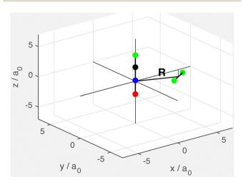
Fig. 3 Geometry of the global minimum of the HCNO-H<sub>2</sub> complex. The Jacobi vector is indicated in the figure. The equilibrium intermolecular separation R equals 5.64 $a_0$ , and the angles defining the orientation of the complex are  $\theta_1 = 102^\circ$ ,  $\theta_2 = 48^\circ$ ,  $\phi = 0^\circ$ . The color coding of the atoms is as follows: H, green; C, black; N, blue; O, red.
