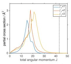
Fig. 4 Partial cross sections for the collision of the  $j_1 = 0$  level of HCNO with  $o-H_2$  at a total energy of 100 cm $^{-1}$ . The final levels are indicated in the legend. The vertical dashed line shows the highest partial wave included in the initegral cross section
