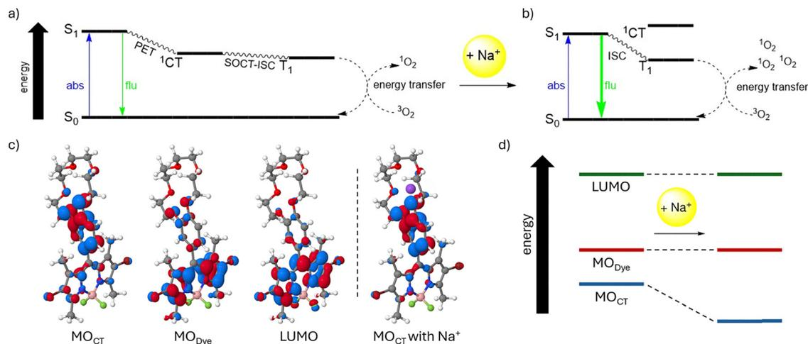
Fig. 5 Jablonski diagram of the postulated mechanism of the photosensitized production of  $^1\text{O}_2$  in the PS **1** in polar solvents (a) without  $\text{Na}^+$  and (b) with  $\text{Na}^+$ . (c) Molecular orbitals (MOs) of **1** corresponding to the  $S_1$  and  $^1\text{CT}$  excited states (see further explanations in the text). (d) Relative MO energy level changes of **1** due to the addition of  $\text{Na}^+$ .
