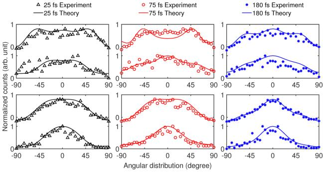
Fig. 7 Angular distribution of  $Cl^+$  with respect to laser polarization axis for *cis*- (1st row) and *trans*-DCE (2nd row) for the  $Cl^+ + C_2H_2Cl^+$  fragmentation channel. In each plot, the top curve shows the angular distribution for the high-energy component of KER and the bottom curve shows the angular distribution for the low-energy component of KER.
