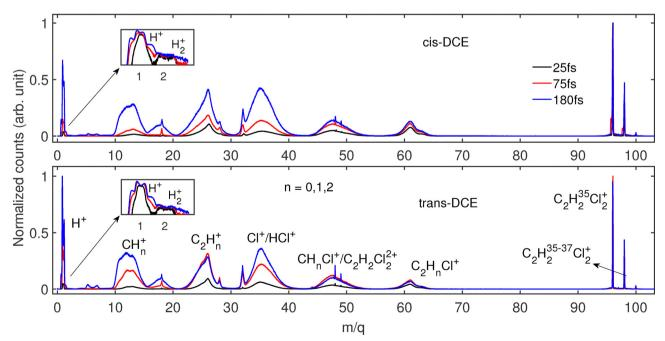
Fig. 2 Calibrated mass spectra of *cis*-DCE [top] and *trans*-DCE [bottom] recorded for linearly polarized laser pulses at 25, 75, and 180 fs pulse durations and fixed peak intensity.
